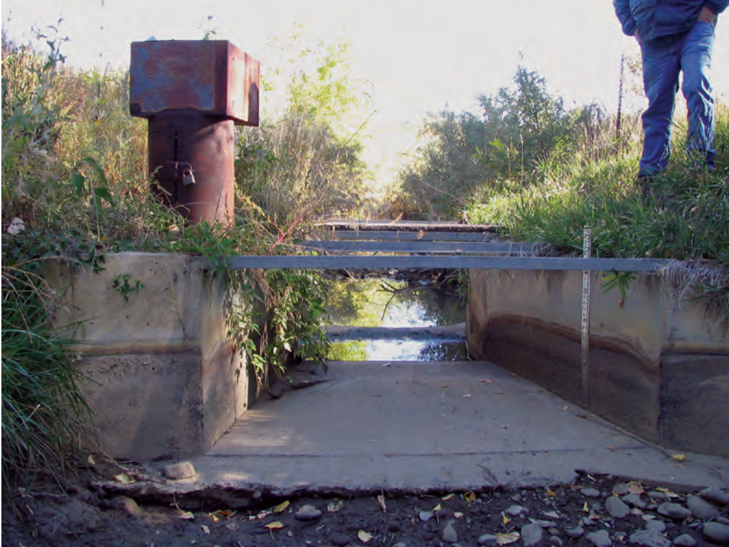
Figure 2. Water-stage recorder and Parshall flume at measurement site HOHG (Hoehne Canal headgate).
