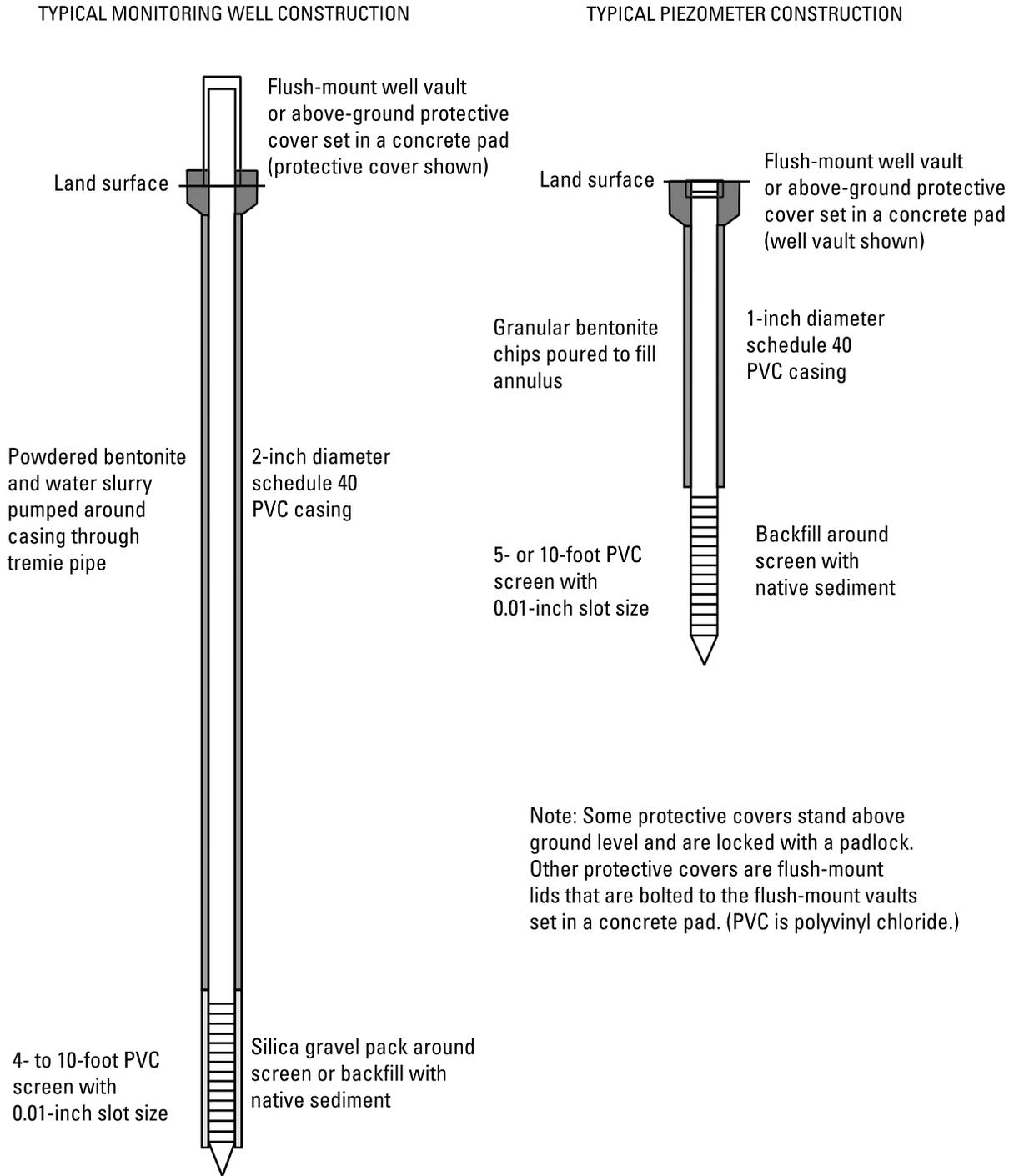
**Figure 6.** Diagram of monitoring wells and piezometers for investigation of the hydrogeologic framework in Quaternary deposits at the U.S. Army Atterbury Joint Maneuver Training Center near Edinburgh, Indiana.
