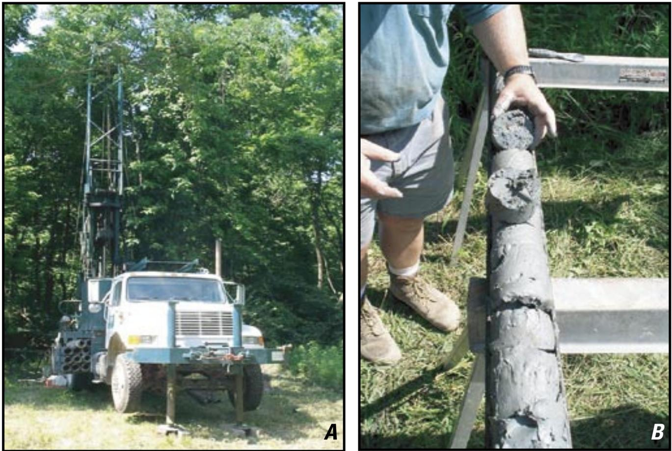
**Figure 4.** Photographs of (A) the truck-mounted hollow-stem auger drill rig used to collect sediment cores and construct monitoring wells and (B) an example core collected with this drill rig at the U.S. Army Atterbury Joint Maneuver Training Center, near Edinburgh, Indiana.
