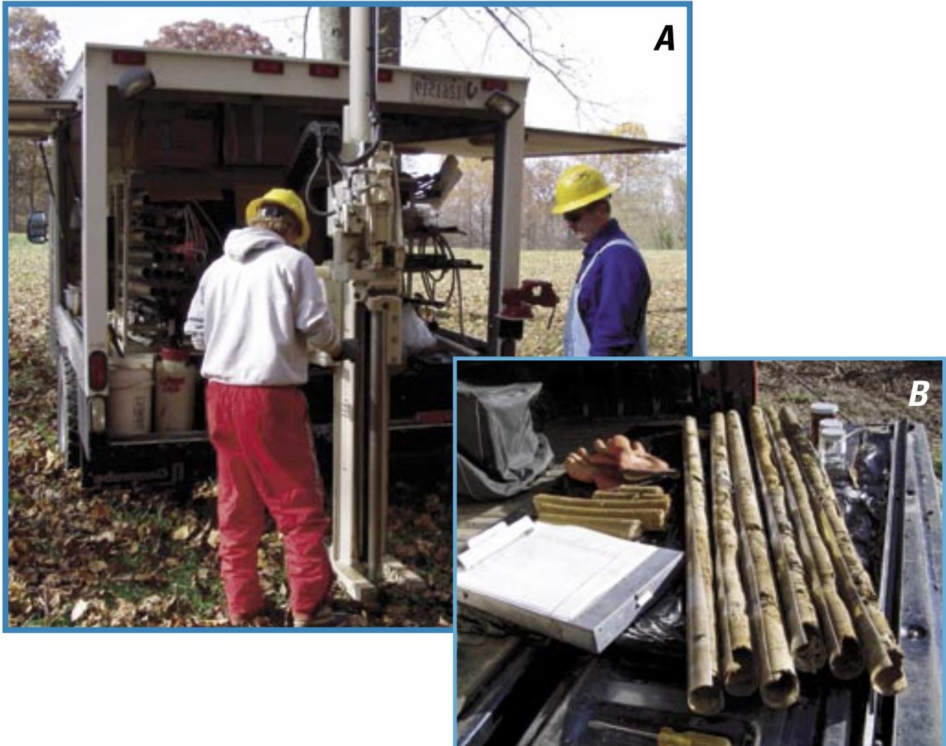
**Figure 5.** Photographs of (A) the direct-push drill rig used to collect sediment cores and construct piezometers at the U.S. Army Atterbury Joint Maneuver Training Center, near Edinburg, Indiana, and (B) a core collected with this drill rig.
