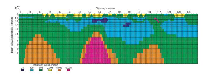
Appendix 5–7.4. Sections from line 2 showing inversion results of the (A) field data and (B) synthetic forward-model data for the Wenner-Schlumberger array, as well as (C) the forward model itself for the scenario without voids.
