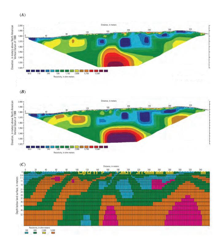
Appendix 5–2.4. Sections from line 3 showing inversion results of the (A) field data and (B) synthetic forward-model data for the Wenner-Schlumberger array, as well as (C) the forward model itself for the scenario without voids.
