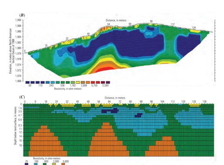
Appendix 5–7.3. Sections from line 2 showing inversion results of the (A) field data and (B) synthetic forward-model data for the Wenner-Schlumberger array, as well as (C) the forward model itself for the scenario with voids.
