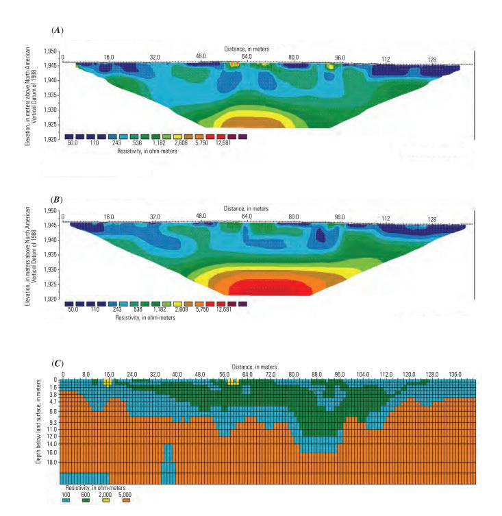
Appendix 5–1.5. Sections from line 6 showing inversion results of the (A) field data and (B) synthetic forward-model data for the high-resolution Wenner-Schlumberger array, as well as (C) the forward model itself for the scenario with voids.
