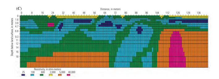
Appendix 5–6.4. Sections from line 5 showing inversion results of the (A) field data and (B) synthetic forward-model data for the Wenner-Schlumberger array, as well as (C) the forward model itself for the scenario without voids.
