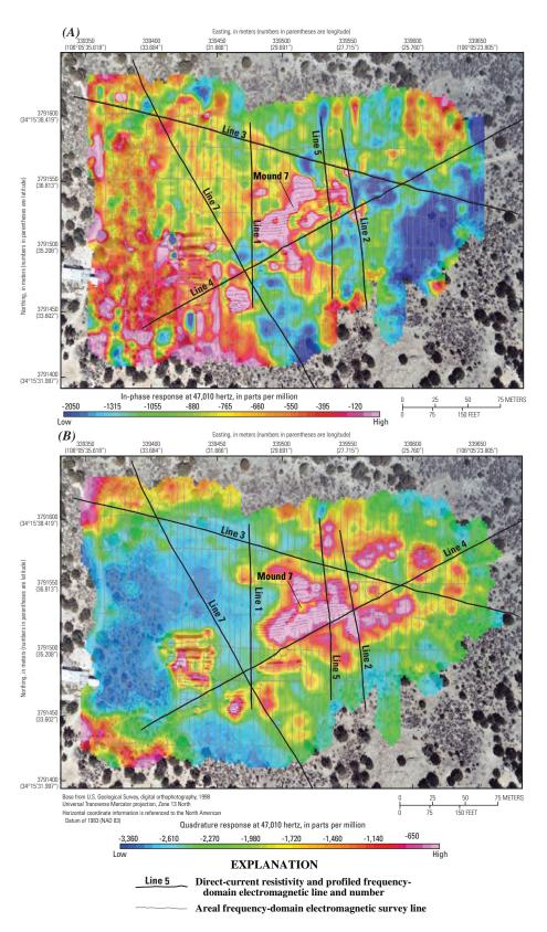
**Figure 9.** Results of the areal frequency-domain electromagnetic survey showing (A) in-phase and (B) quadrature response at 47,010 Hertz; (C) in-phase and (D) quadrature response at 13,590 Hertz, and (E) in-phase and (F) quadrature response at 3,930 Hertz.
