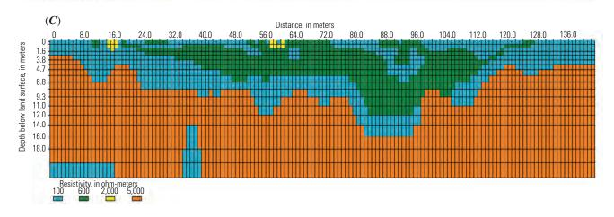
Appendix 5–1.3. Sections from line 6 showing inversion results of the (A) field data and (B) synthetic forward-model data for the Wenner-Schlumberger array, as well as (C) the forward model itself for the scenario with voids.
