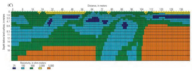
Appendix 5–7.1. Sections from line 2 showing inversion results of the (A) field data and (B) synthetic forward-model data for the dipole-dipole array, as well as (C) the forward model itself for the scenario with voids.
