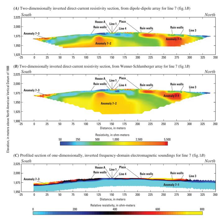
**Figure 12.** Surface-geophysical data showing inverted direct-current resistivity sections from (A) dipole-dipole and (B) Wenner-Schlumberger arrays, as well as (C) inverted frequency-domain electromagnetic data from line 7.
