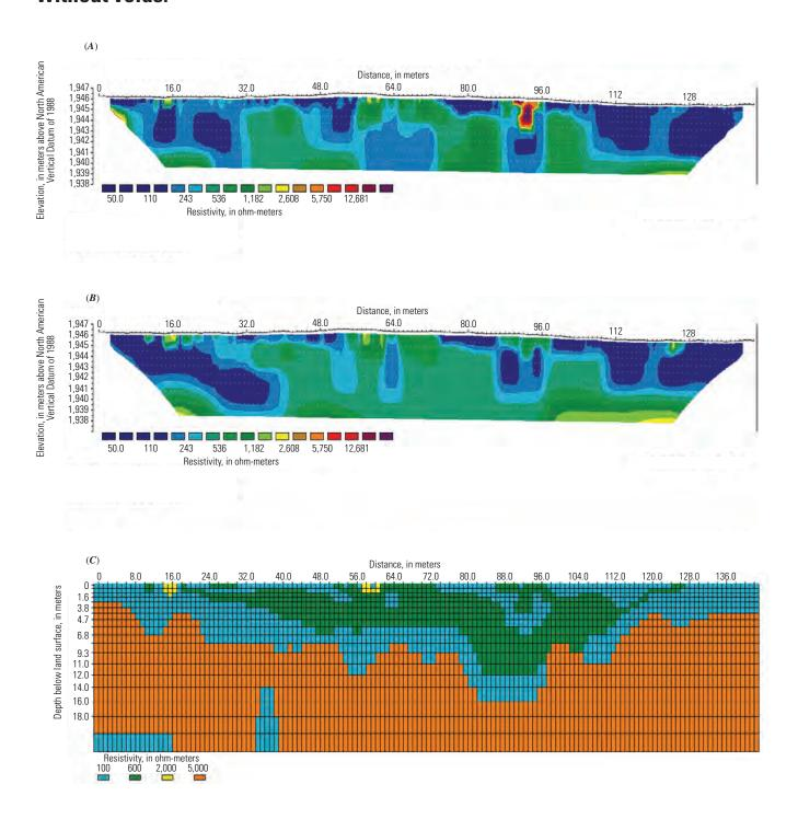
Appendix 5–2.1. Sections from line 3 showing inversion results of the (A) field data and (B) synthetic forward-model data for the dipole-dipole array, as well as (C) the forward model itself for the scenario with voids.
