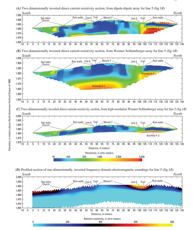
**Figure 14.** Surface-geophysical data showing inverted direct-current resistivity sections from (A) dipole-dipole, and (B) Wenner-Schlumberger arrays, as well as (D) inverted frequency-domain electromagnetic data from line 5.
