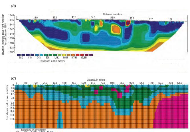
Appendix 5–1.2. Sections from line 6 showing inversion results of the (A) field data and (B) synthetic forward-model data for the dipole-dipole array, as well as (C) the forward model itself for the scenario without voids.
