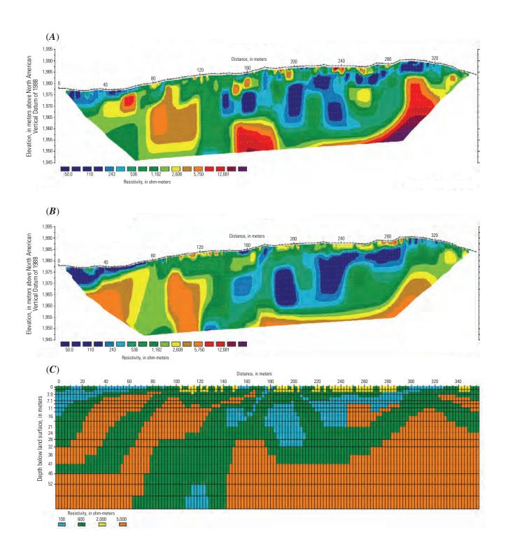
Appendix 5–2.3. Sections from line 3 showing inversion results of the (A) field data and (B) synthetic forward-model data for the Wenner-Schlumberger array, as well as (C) the forward model itself for the scenario with voids.
