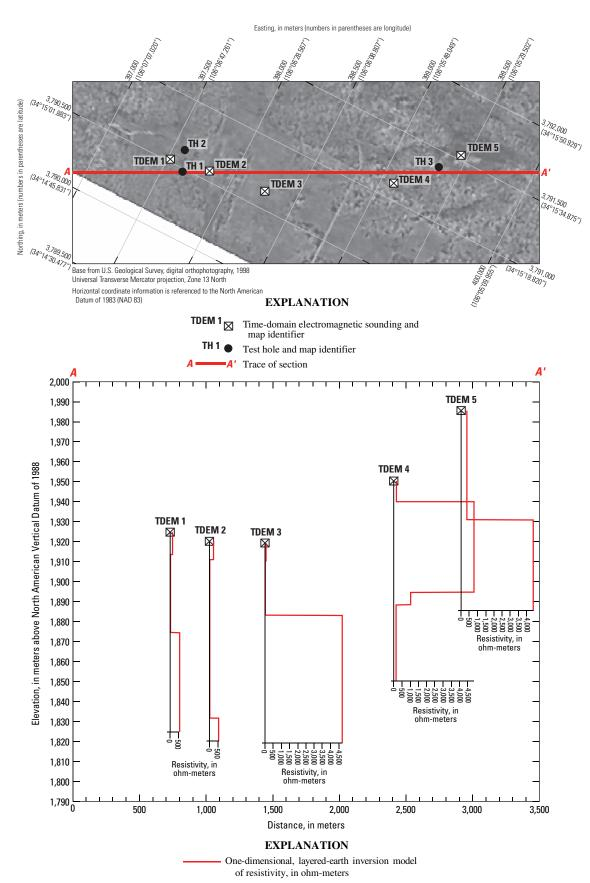
**Figure 6**. One-dimensional, layered-earth inversion models from time-domain electromagnetic sounding data (shown in profile along trace of section A–A').
