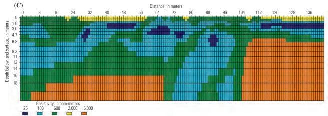
Appendix 5–6.3. Sections from line 5 showing inversion results of the (A) field data and (B) synthetic forward-model data for the Wenner-Schlumberger array, as well as (C) the forward model itself for the scenario with voids.
