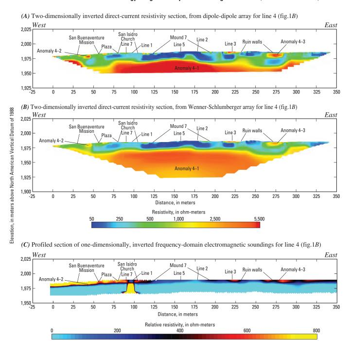
**Figure 11.** Surface-geophysical data showing inverted direct-current resistivity sections from (A) dipole-dipole and (B) Wenner-Schlumberger arrays, as well as (C) inverted frequency-domain electromagnetic data from line 4.
