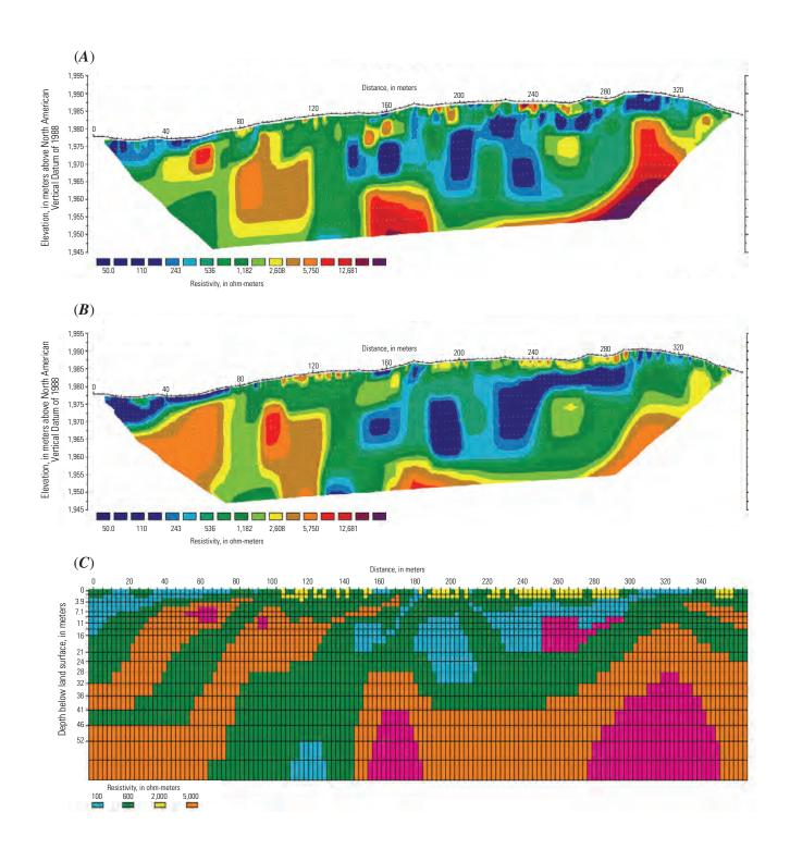
Appendix 5–2.2. Sections from line 3 showing inversion results of the (A) field data and (B) synthetic forward-model data for the dipole-dipole array, as well as (C) the forward model itself for the scenario without voids.
