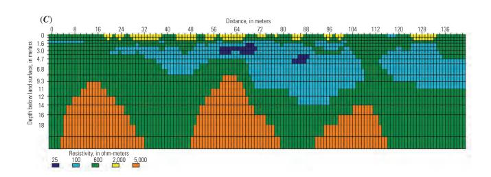
Appendix 5–7.5. Sections from line 2 showing inversion results of the (A) field data and (B) synthetic forward-model data for the high-resolution Wenner-Schlumberger array, as well as (C) the forward model itself for the scenario with voids.
