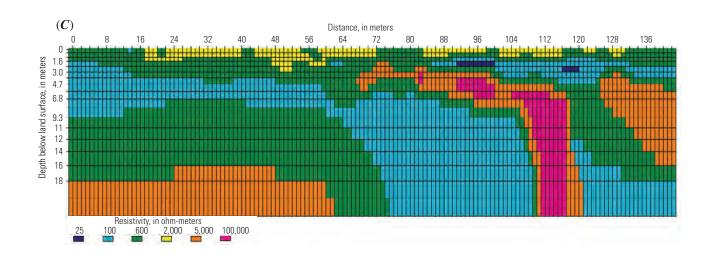
Appendix 5–5.4. Sections from line 1 showing inversion results of the (A) field data and (B) synthetic forward-model data for the Wenner-Schlumberger array, as well as (C) the forward model itself for the scenario without voids.
