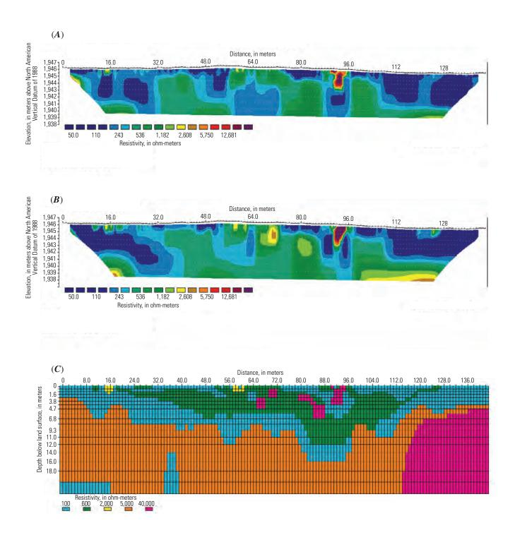
Appendix 5–1.6. Sections from line 6 showing inversion results of the (A) field data and (B) synthetic forward-model data for the high-resolution Wenner-Schlumberger array, as well as (C) the forward model itself for the scenario without voids.
