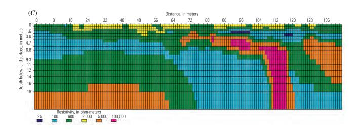
Appendix 5–5.2. Sections from line 1 showing inversion results of the (A) field data and (B) synthetic forward-model data for the dipole-dipole array, as well as (C) the forward model itself for the scenario without voids.
