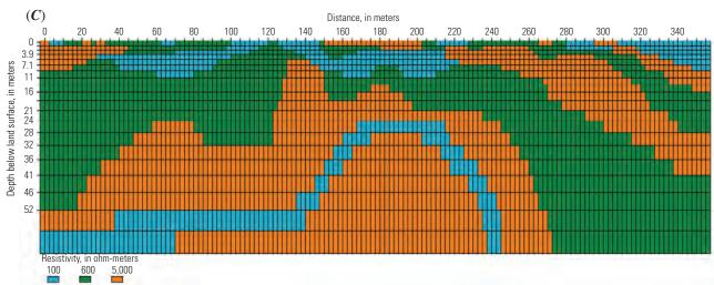
Appendix 5–4.3. Sections from line 7 showing inversion results of the (A) field data and (B) synthetic forward-model data for the Wenner-Schlumberger array, as well as (C) the forward model itself for the scenario with voids.
