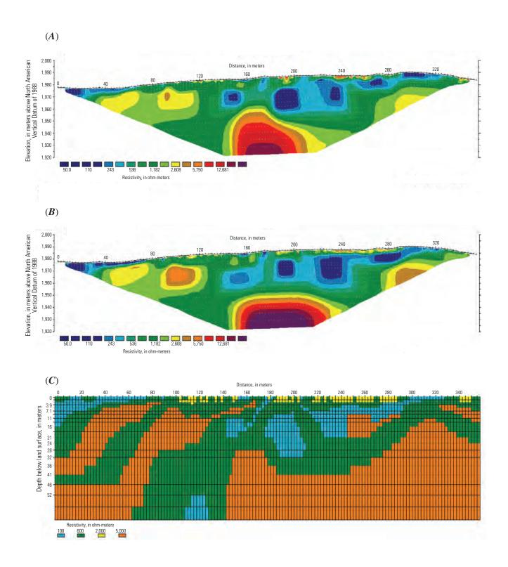
Appendix 5–3.1. Sections from line 4 showing inversion results of the (A) field data and (B) synthetic forward-model data for the dipole-dipole array, as well as (C) the forward model itself for the scenario with voids.
