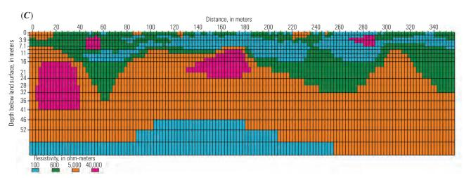
Appendix 5–3.2. Sections from line 4 showing inversion results of the (A) field data and (B) synthetic forward-model data for the dipole-dipole array, as well as (C) the forward model itself for the scenario without voids.
