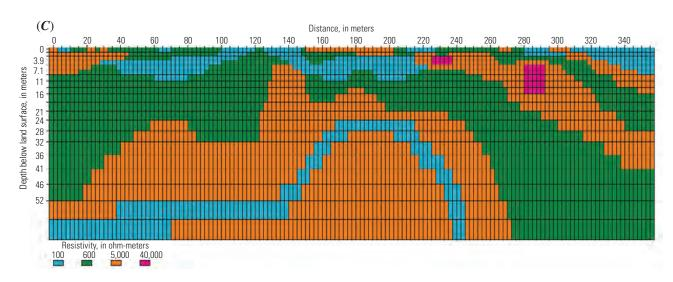
Appendix 5–4.4. Sections from line 7 showing inversion results of the (A) field data and (B) synthetic forward-model data for the Wenner-Schlumberger array, as well as (C) the forward model itself for the scenario without voids.
