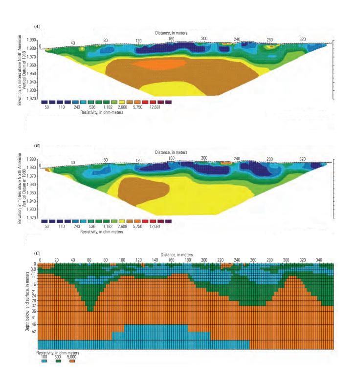
Appendix 5–4.1. Sections from line 7 showing inversion results of the (A) field data and (B) synthetic forward-model data for the dipole-dipole array, as well as (C) the forward model itself for the scenario with voids.
