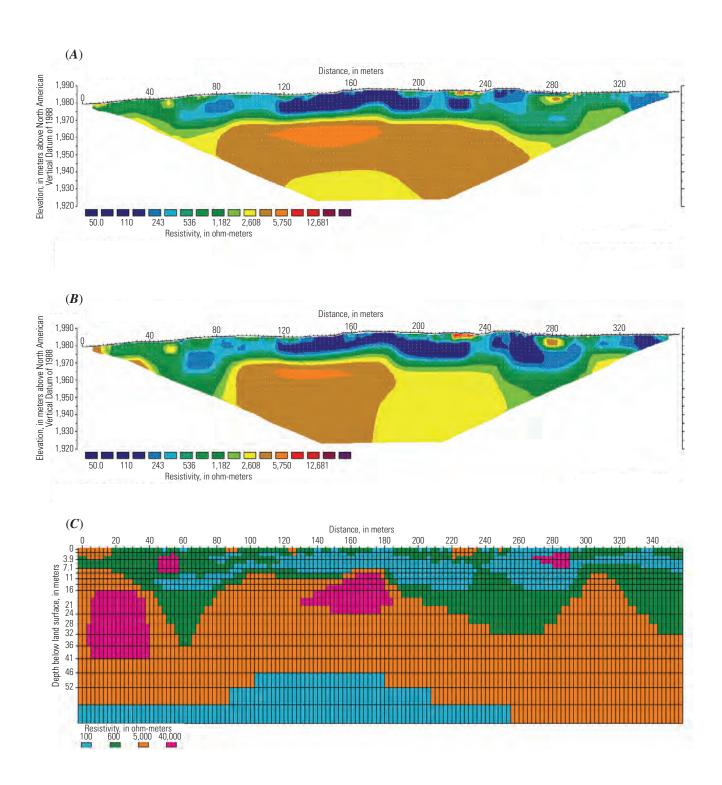
Appendix 5–3.4. Sections from line 4 showing inversion results of the (A) field data and (B) synthetic forward-model data for the Wenner-Schlumberger array, as well as (C) the forward model itself for the scenario without voids.
