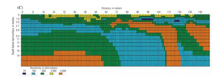
Appendix 5–5.3. Sections from line 1 showing inversion results of the (A) field data and (B) synthetic forward-model data for the Wenner-Schlumberger array, as well as (C) the forward model itself for the scenario with voids.
