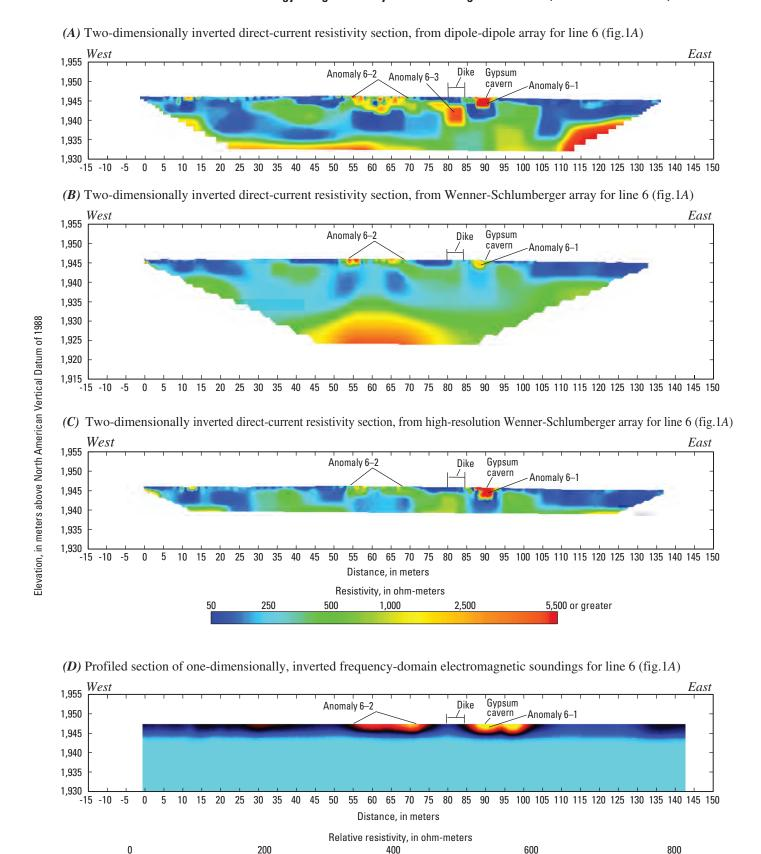
**Figure 7.** Profiles of surface-geophysical data from line 6 (fig. 1*A*) showing inverted direct-current resistivity sections from the (*A*) dipole-dipole, (*B*) Wenner-Schlumberger, and (*C*) high-resolution Wenner-Schlumberger arrays, as well as (*D*) profiled, inverted frequency-domain electromagnetic soundings.
