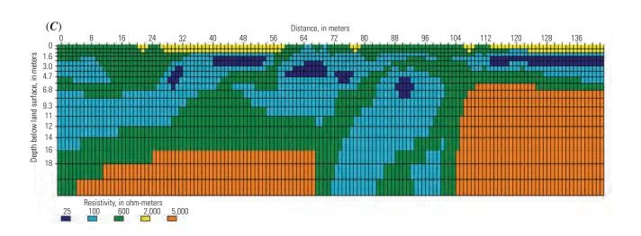
Appendix 5–6.5. Sections from line 5 showing inversion results of the (A) field data and (B) synthetic forward-model data for the high-resolution Wenner-Schlumberger array, as well as (C) the forward model itself for the scenario with voids.
