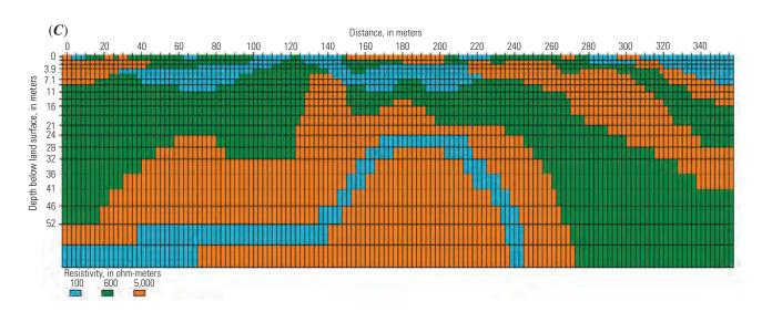
Appendix 5–5.1. Sections from line 1 showing inversion results of the (A) field data and (B) synthetic forward-model data for the dipole-dipole array, as well as (C) the forward model itself for the scenario with voids.
