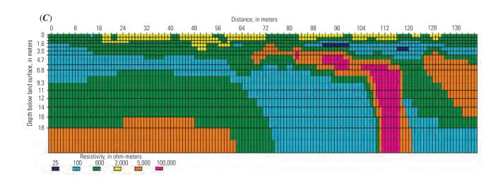
Appendix 5–5.6. Sections from line 1 showing inversion results of the (A) field data and (B) synthetic forward-model data for the high-resolution Wenner-Schlumberger array, as well as (C) the forward model itself for the scenario without voids.
