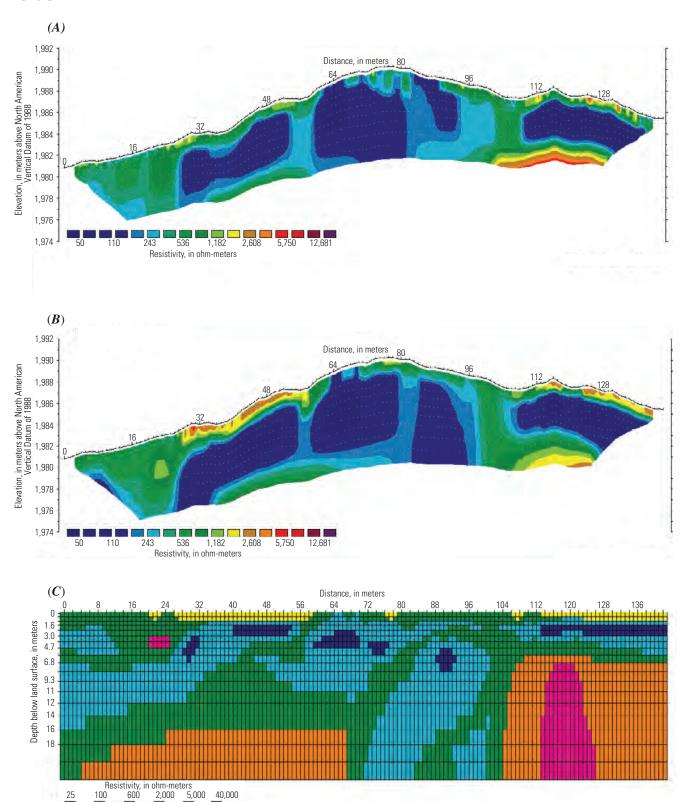
Appendix 5–6.6. Sections from line 5 showing inversion results of the (A) field data and (B) synthetic forward-model data for the high-resolution Wenner-Schlumberger array, as well as (C) the forward model itself for the scenario without voids.
