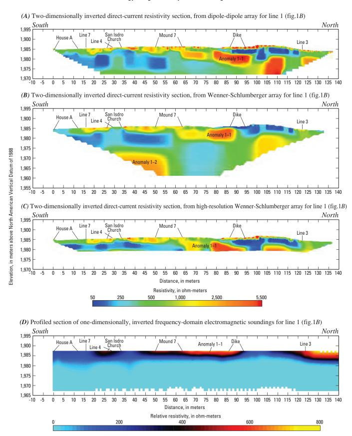
**Figure 13.** Surface-geophysical data showing inverted direct-current resistivity sections from (A) dipole-dipole and (B) Wenner-Schlumberger arrays, as well as (D) inverted frequency-domain electromagnetic data from line 1.
