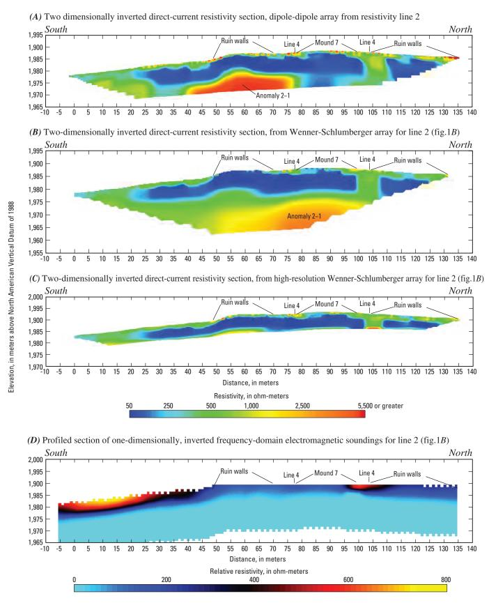
**Figure 15.** Surface-geophysical data showing inverted direct-current resistivity sections from (A) dipole-dipole, and (B) Wenner-Schlumberger arrays, as well as (D) inverted frequency-domain electromagnetic data from line 2.
