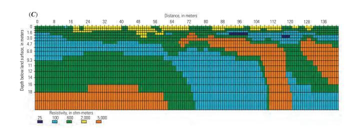
Appendix 5–6.1. Sections from line 5 showing inversion results of the (A) field data and (B) synthetic forward-model data for the dipole-dipole array, as well as (C) the forward model itself for the scenario with voids.
