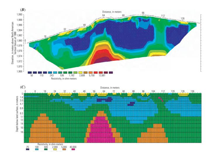
Appendix 5–7.2. Sections from line 2 showing inversion results of the (A) field data and (B) synthetic forward-model data for the dipole-dipole array, as well as (C) the forward model itself for the scenario without voids.
