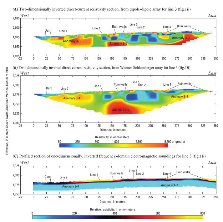
**Figure 10.** Surface-geophysical data showing inverted direct-current resistivity sections from (A) dipole-dipole and (B) Wenner-Schlumberger arrays, as well as (C) inverted frequency-domain electromagnetic data from line 3.
