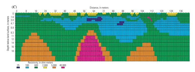
Appendix 5–7.6. Sections from line 2 showing inversion results of the (A) field data and (B) synthetic forward-model data for the high-resolution Wenner-Schlumberger array, as well as (C) the forward model itself for the scenario without voids.
