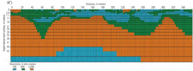
Appendix 5–3.3. Sections from line 4 showing inversion results of the (A) field data and (B) synthetic forward-model data for the Wenner-Schlumberger array, as well as (C) the forward model itself for the scenario with voids.
