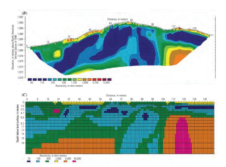
Appendix 5–6.2. Sections from line 5 showing inversion results of the (A) field data and (B) synthetic forward-model data for the dipole-dipole array, as well as (C) the forward model itself for the scenario without voids.
