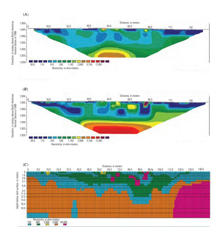
Appendix 5–1.4. Sections from line 6 showing inversion results of the (A) field data and (B) synthetic forward-model data for the Wenner-Schlumberger array, as well as (C) the forward model itself for the scenario without voids.
