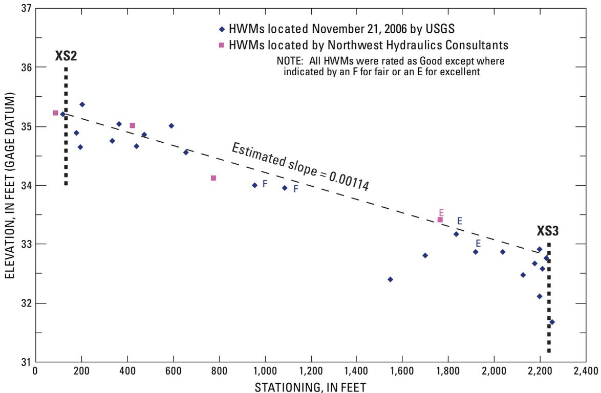
**Figure 2.** High-water marks (HWMs) from peak flow of November 6, 2006, that was surveyed November 21, 2006, by the U.S. Geological Survey on the right bank between cross sections 2 (XS2) and 3 (XS3) on the Skagit River about 3,000–5,000 feet downstream of the streamflow-gaging station, Skagit River near Concrete, Washington (station No. 12194000).
