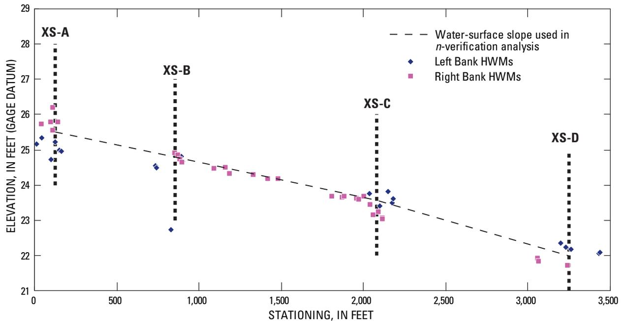
**Figure 5.** High-water marks (HWMs), cross sections (XS), and water-surface profile from the peak flow of November 27, 1949 on the Skagit River about 3,000–5,000 feet downstream of the streamflow-gaging station, Skagit River near Concrete, Washington (station No. 12194000).
