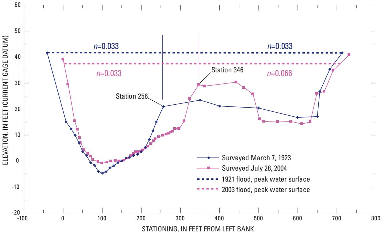
**Figure 3.** Cross section XS2 as surveyed in 1923 and 2004,  $n$  values for the particular subareas ( $n$ ), peak water surface for the 1921 and 2003 floods, and the points at which the cross sections were subdivided into two subareas. [Note: Stationing for the 1923 surveyed cross section was adjusted to fit the stationing surveyed in 2004.]
