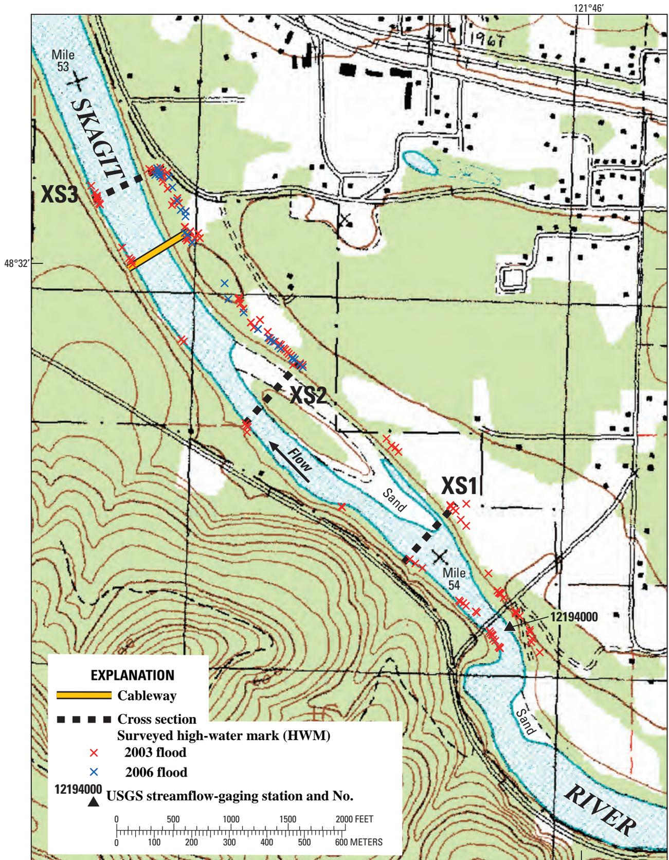
**Figure 1.** Topographic map of the slope-area measurement reach on the Skagit River near Concrete showing the three cross sections (XS1, XS2, and XS3), the streamflow-gaging station, and HWMs from the 2003 flood and the 2006 flood surveyed by the U.S. Geological Survey.
