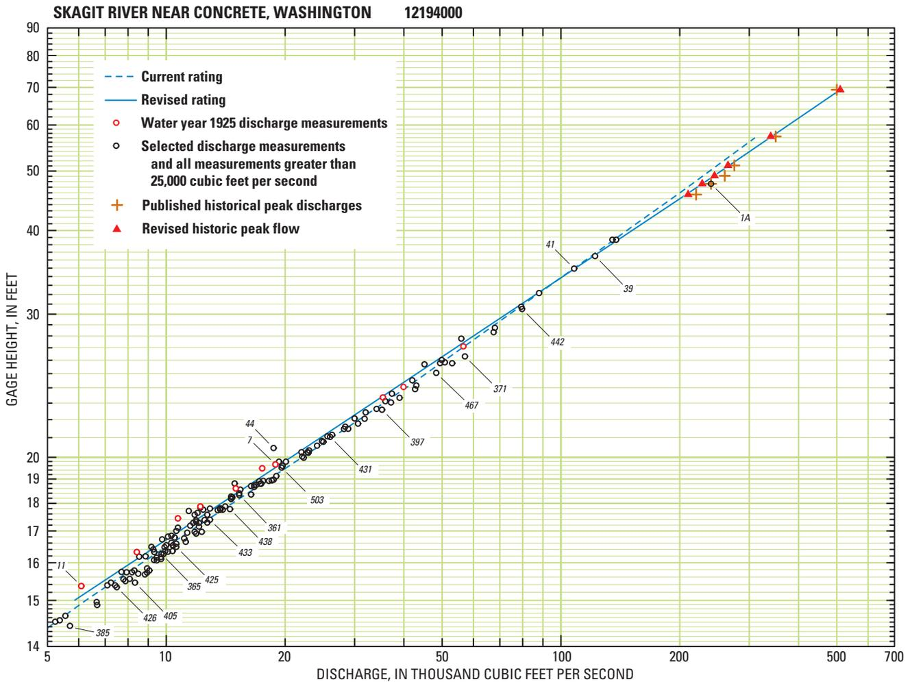
**Figure 7.** Stage-discharge rating based on revised 1921 peak discharge recalculation extended to a gage height of 69.3 feet and the current stage-discharge rating for Skagit River near Concrete, Washington, showing selected discharge measurements, published historical peak discharges, and the proposed revised historic peak flows.
