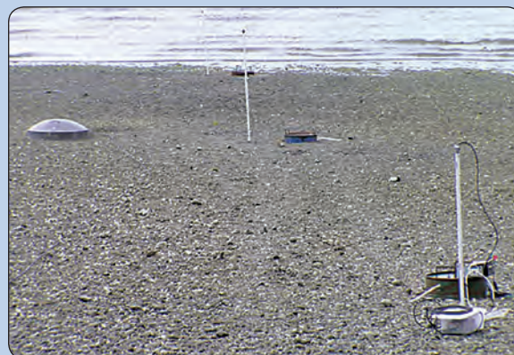
Sidebar E. Linear array of minipiezometers (white pipes), Lee-type seepage meters (partly buried colored barrels), and electromagnetic seepage meter (ESM) (aluminum dome) at Sunset Beach are exposed at low tide. When the beach is submerged at high tide, the ESM is capable of measuring and recording seepage rates at 1-minute intervals. Photograph taken by F. William Simonds, U.S. Geological Survey, June 9, 2006.
