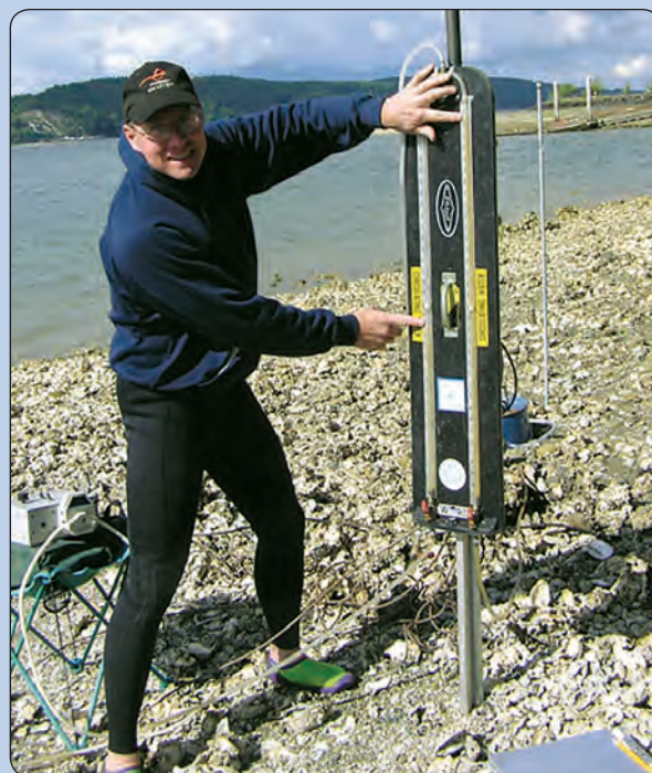
▼ Sidebar B. Difference in vertical hydraulic head between surface water and ground water can be directly measured using a manometer in conjunction with a minipiezometer. Relative ground-water head, on the right side of the manometer, is higher than the relative surface-water head, on the left side of the board, indicating an upward vertical hydraulic gradient. Photograph taken by F. William Simonds, U.S. Geological Survey, June 26, 2005.
