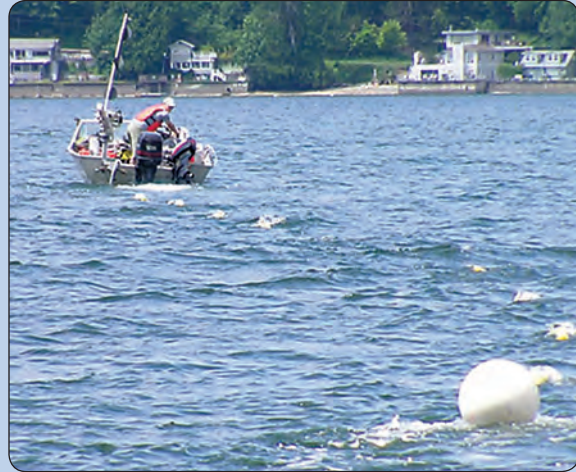
▼ Sidebar D. A streaming resistivity survey was conducted using a boat towing a 130-meter cable near the surface of the water. The cable, which is wrapped with pieces of styrofoam to stay afloat, has two source electrodes nearest the boat and nine receiver electrodes spaced 10 meters apart. Data are collected as the cable is towed parallel to the shoreline in about 3 to 10 meters of water. Photograph taken by F. William Simonds, U.S. Geological Survey, June 8, 2006.
