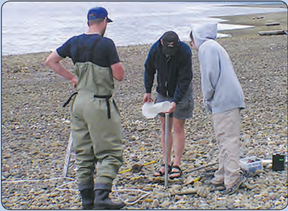
Sidebar H. Conducting slug tests in a minipiezometer at the Landon Road intensive study site. The intertidal area on the north shore of Lynch Cove is composed of cobbles and gravel indicative of a higher energy environment. Photograph taken by F. William Simonds, U.S. Geological Survey, June 22, 2005.
