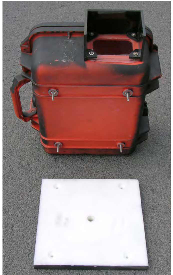
Figure 5. This view shows the screws protruding from the bottom of the Pelican 1400 case, which are used to attach the polyethylene sheet that may be used to mount the camera enclosure on a standard surveyor's tripod. The rain/sun shield and the window are attached over the window opening by using a single set of 4 stainless steel machine screws.
