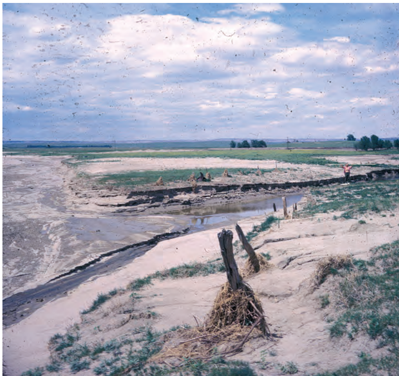
Figure A78. View looking upstream, Jimmy Camp Creek at Fountain, Colorado, July 17, 1965. (Man is holding rod at high-water mark at cross section 1, 250 feet right of left end of cross section.)
