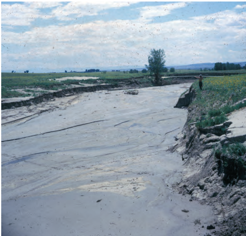
Figure A76. View looking downstream from about 200 feet above cross section 2, Jimmy Camp Creek at Fountain, Colorado, July 17, 1965. (Man is holding rod at high-water mark at cross section 2.)
