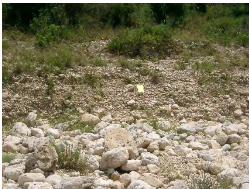
Figure A6. Coarse materials in channel and flood plain of Seco Creek, Texas, June 2003. View toward right bank in slope-area reach. Notebook for scale.
