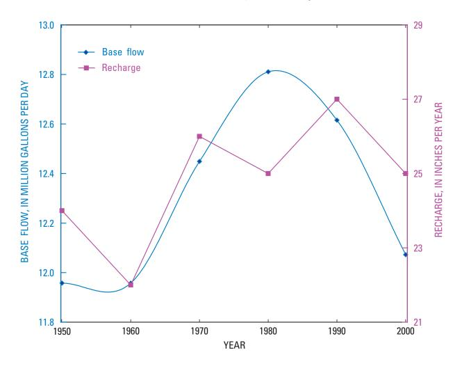
**Figure 9–2.** Simulated base flow in the Winnicut River and estimated recharge for 50 years from 1950 to 2000, Seacoast model area, southeastern New Hampshire.
