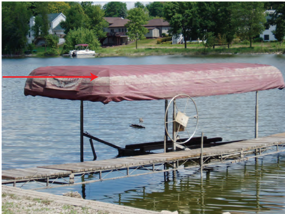
B. Jefferson high-water mark 41, corroborated with water-stain/mud lines on nearby step, light pole, and previously surveyed high-water marks by Jefferson County during the June flood.
