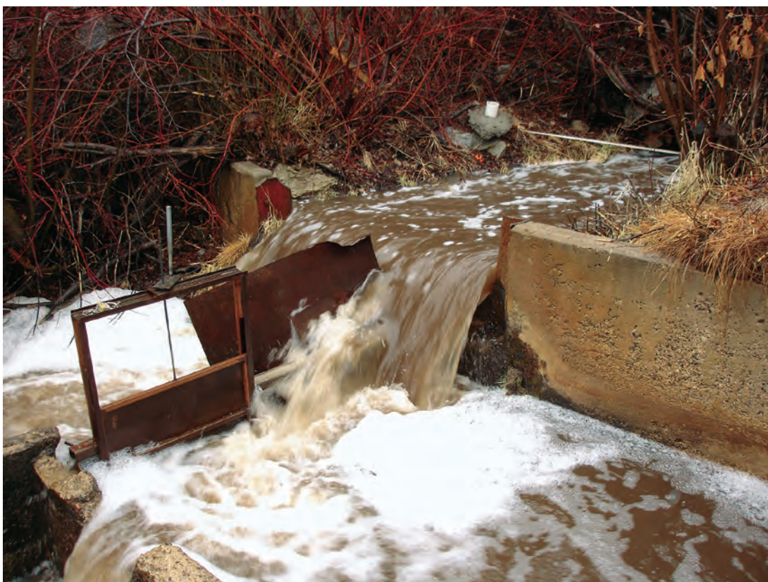
B. Storm runoff in January 2007, when discharge was 13 cubic feet per second. Photograph taken by James Wood, U.S. Geological Survey, January 4, 2007.
