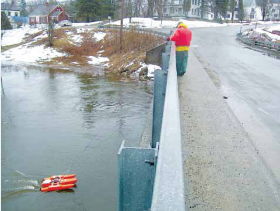
Figure 10. Streamflow measurement taken with acoustic Doppler current profiler on Nezinscot River, April 17, 2007, Turner, Maine.
