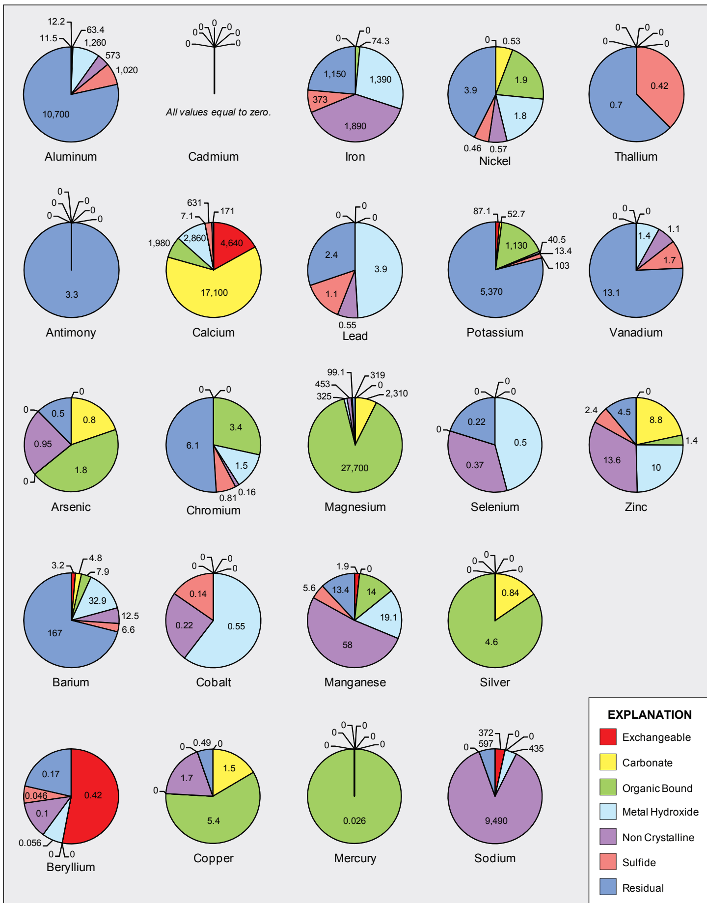
Appendix 5D. Sequential Extraction Procedure analysis of organic mix with Chesapeake Blue compost, seep 3-4W reactive mat pilot test area, West Branch Canal Creek, Aberdeen Proving Ground, Maryland (units are milligrams per kilogram).
