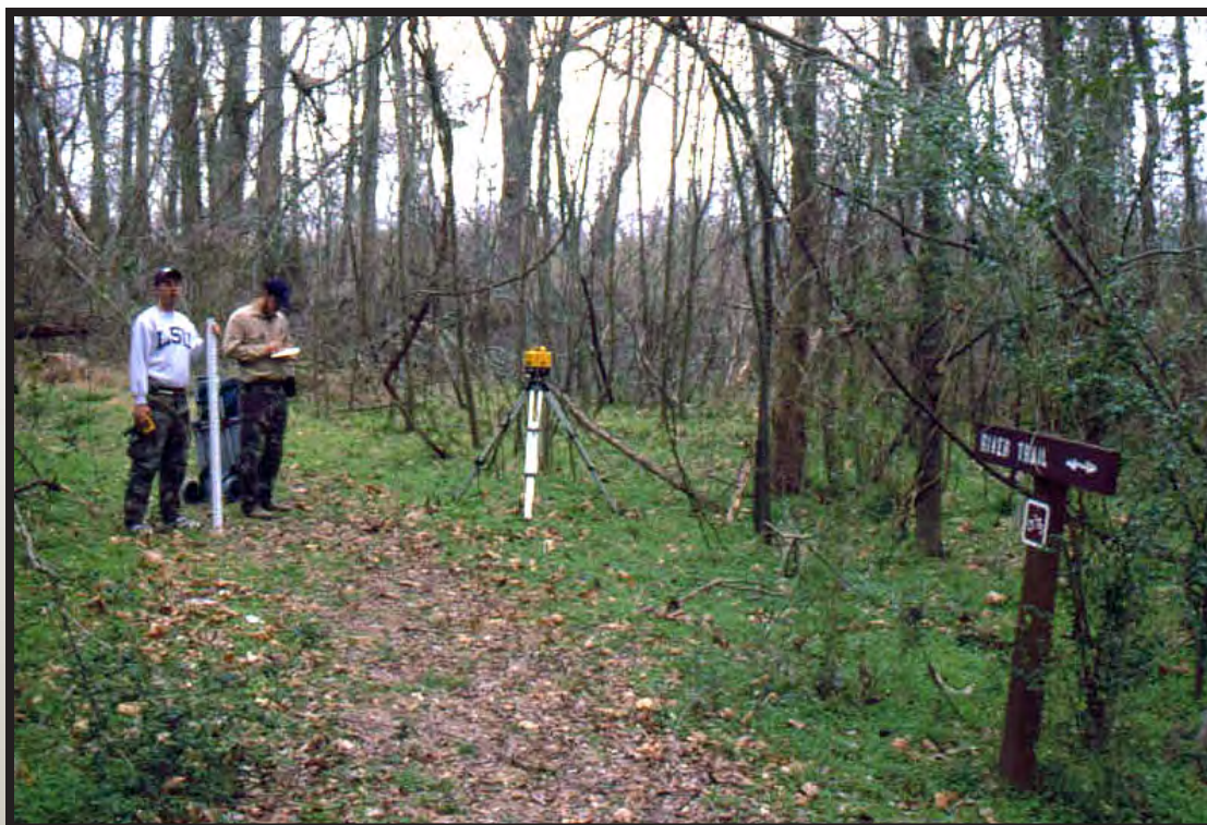
Figure 12. Photograph of trail at Congaree National Park and laser level equipment used to establish vertical elevations of ground and water surfaces.
