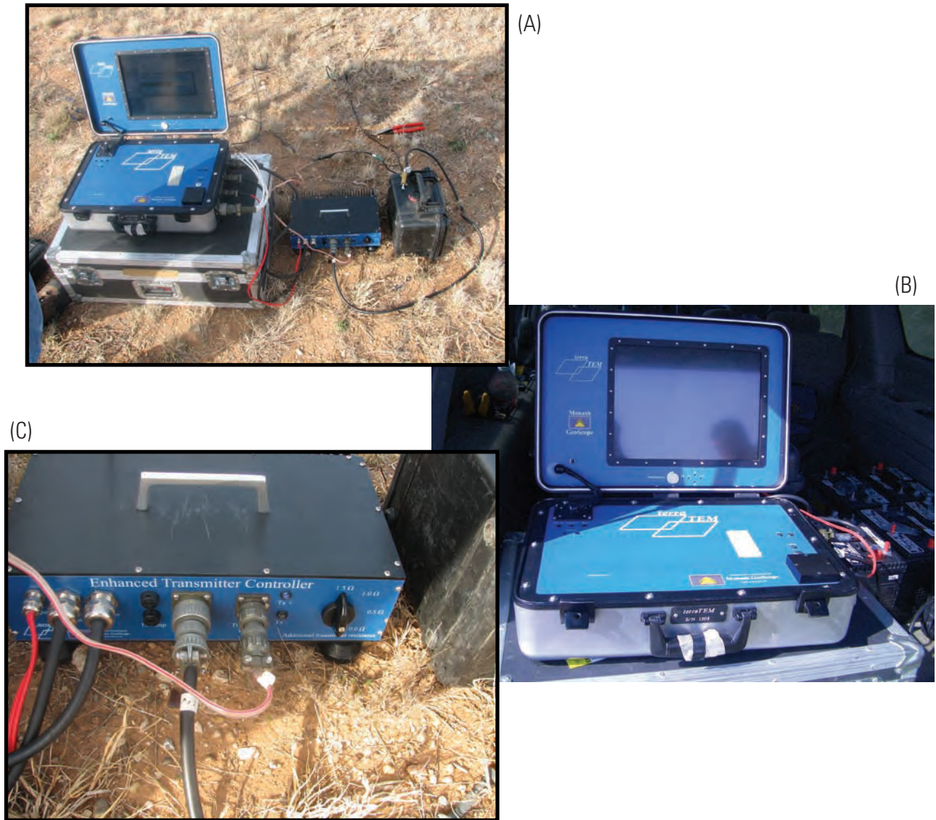
Figure 10. Time-domain electromagnetic sounding equipment used in north-central Nebraska: (A) complete unit including transmitter/receiver, current controller, and battery pack; (B) close up of terraTEM transmitter/receiver unit; and (C) close up of current controller.
