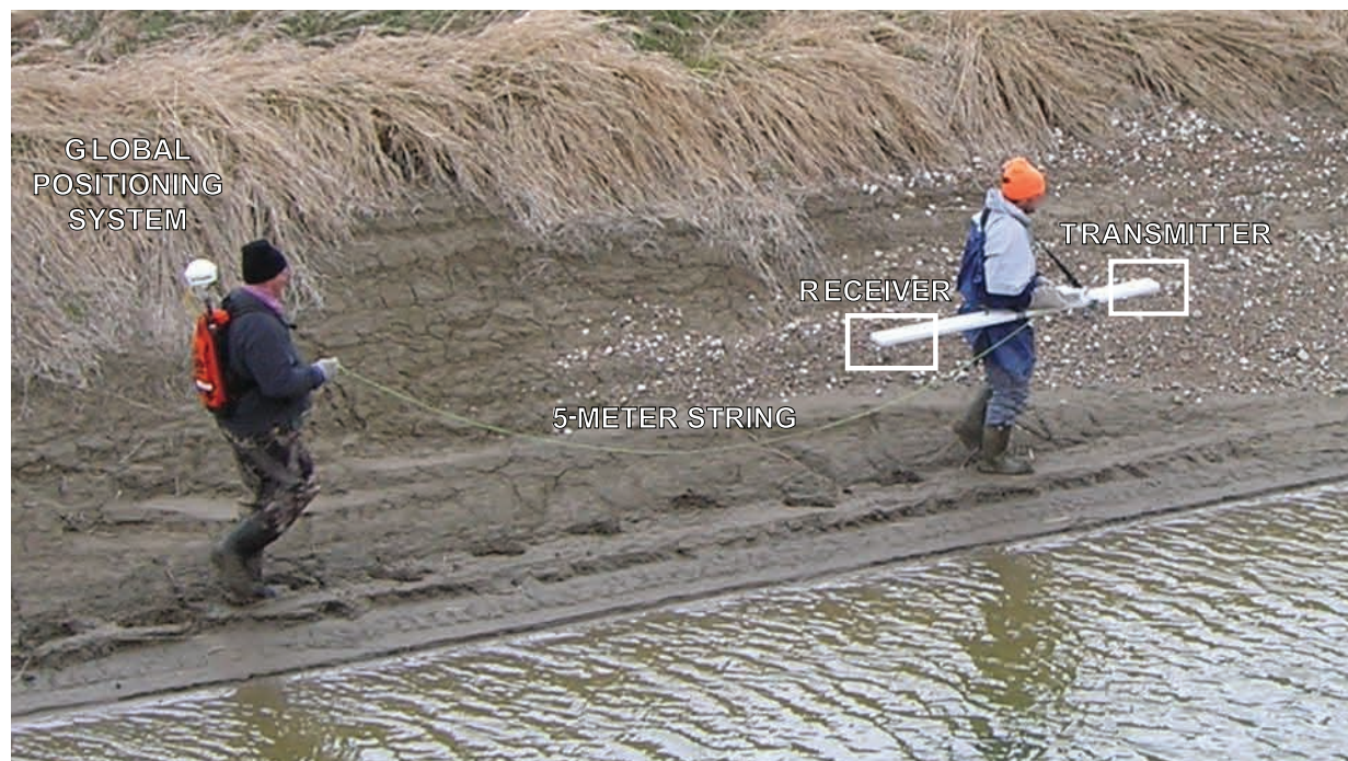
Figure 8. GEM-2 frequency-domain electromagnetic continuous-resistivity profiling equipment used in north-central Nebraska.
