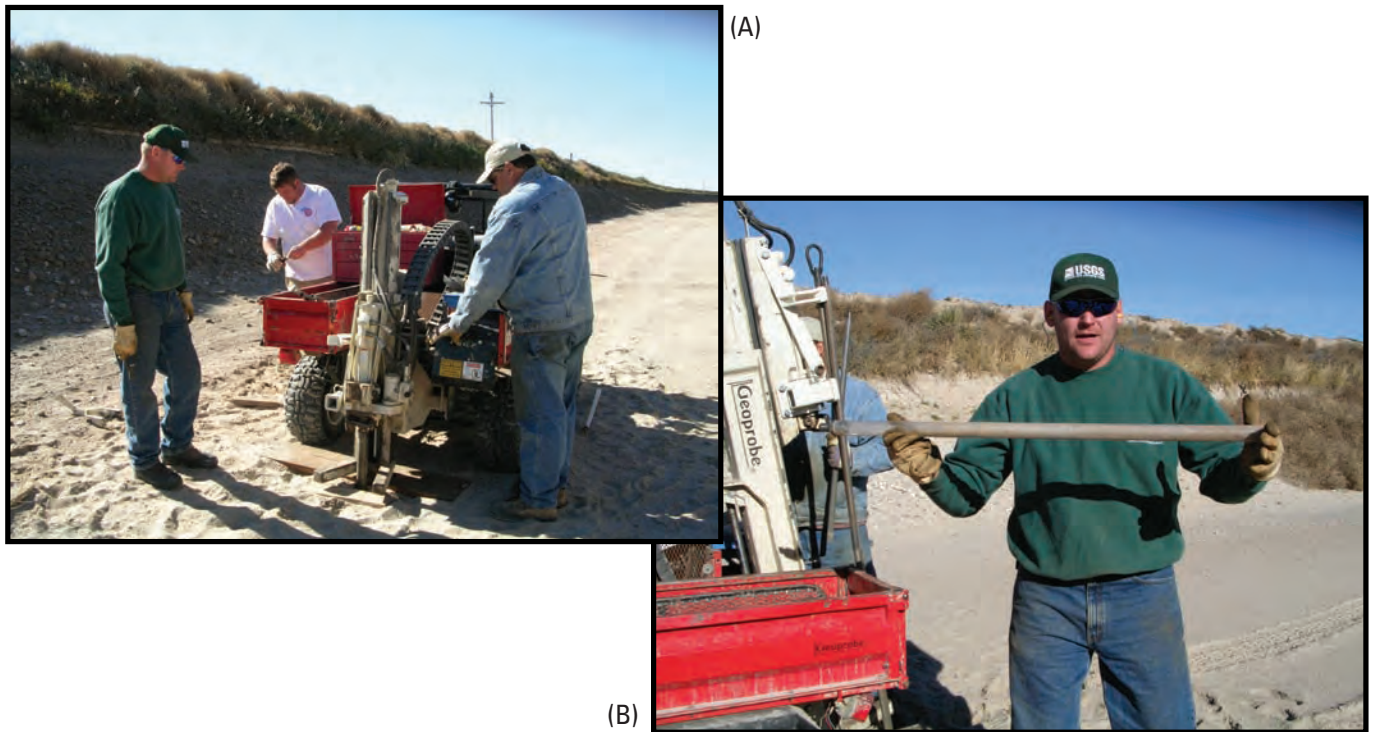
Figure 6. Test-hole coring equipment used in Nebraska: (A) Geoprobe machine mounted on a utility vehicle; and (B) core sample collected at the site, stored in a polyethylene tube.
