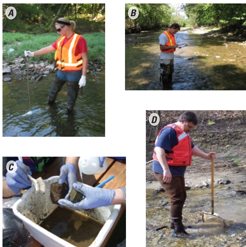
Figure 2. Data collection activities at biological sampling sites in Johnson County, Kansas, 2007, including (A) collecting a water sample for chemical analysis, (B) conducting a habitat assessment, (C) scraping periphyton from streambed rocks, and (D) using a kicknet to collect macroinvertebrates.
