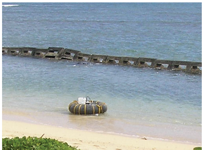
Figure E1. Photograph showing the floating inner-tube platform holding multiparameter water-quality sonde and sample bottles. (Photograph by Joshua Marvit).
