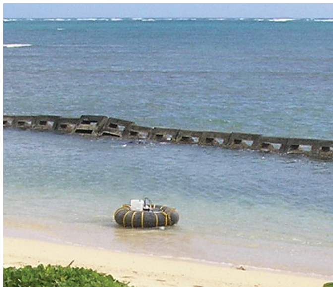
Figure 3. Photograph showing the floating inner-tube platform holding multiparameter water-quality sonde and sample bottles, Kualoa Beach, Oahu, Hawaii. (Photograph by Joshua Marvit.)
