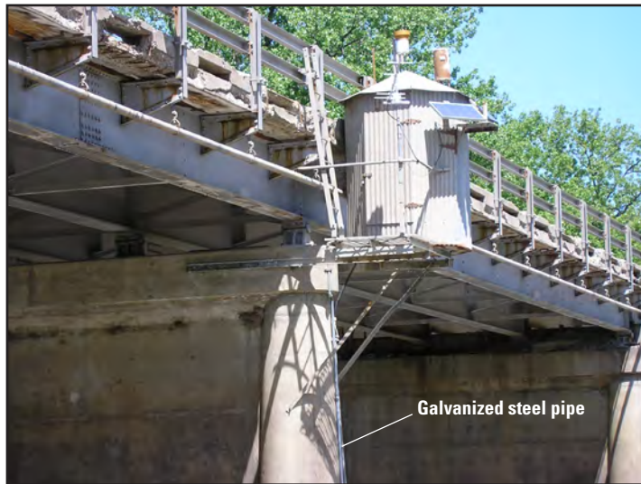
Existing streamgage shelter on the downstream side of pier 7. Note the galvanized steel pipe fastened on the conical column encasing the river channel-bed monitor shielded cable.
