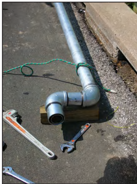
Three-inch galvanized steel pipe with offset encasing the transducer head, which is flush with pipe. Offset designed to prevent acoustic signal interference from pier and footing.
