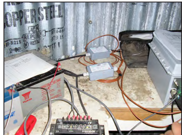
Wiring of NEMA 0183 to SDI-12 conversion devices necessary to ensure recording and transmission of river channel-bed monitor depth soundings.
