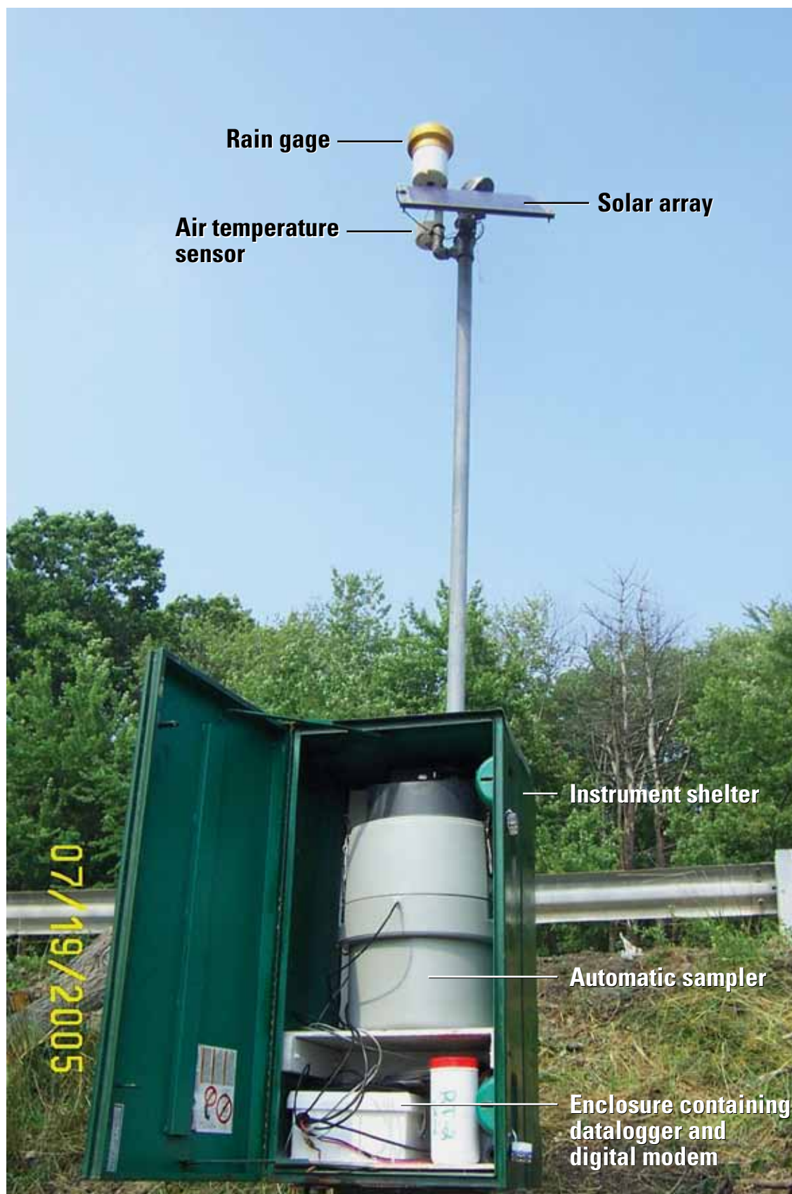
Figure 4. A typical highway-monitoring station used to collect measurements of water level, water temperature, air temperature, specific conductance, and rainfall, and composite samples of highway runoff.
