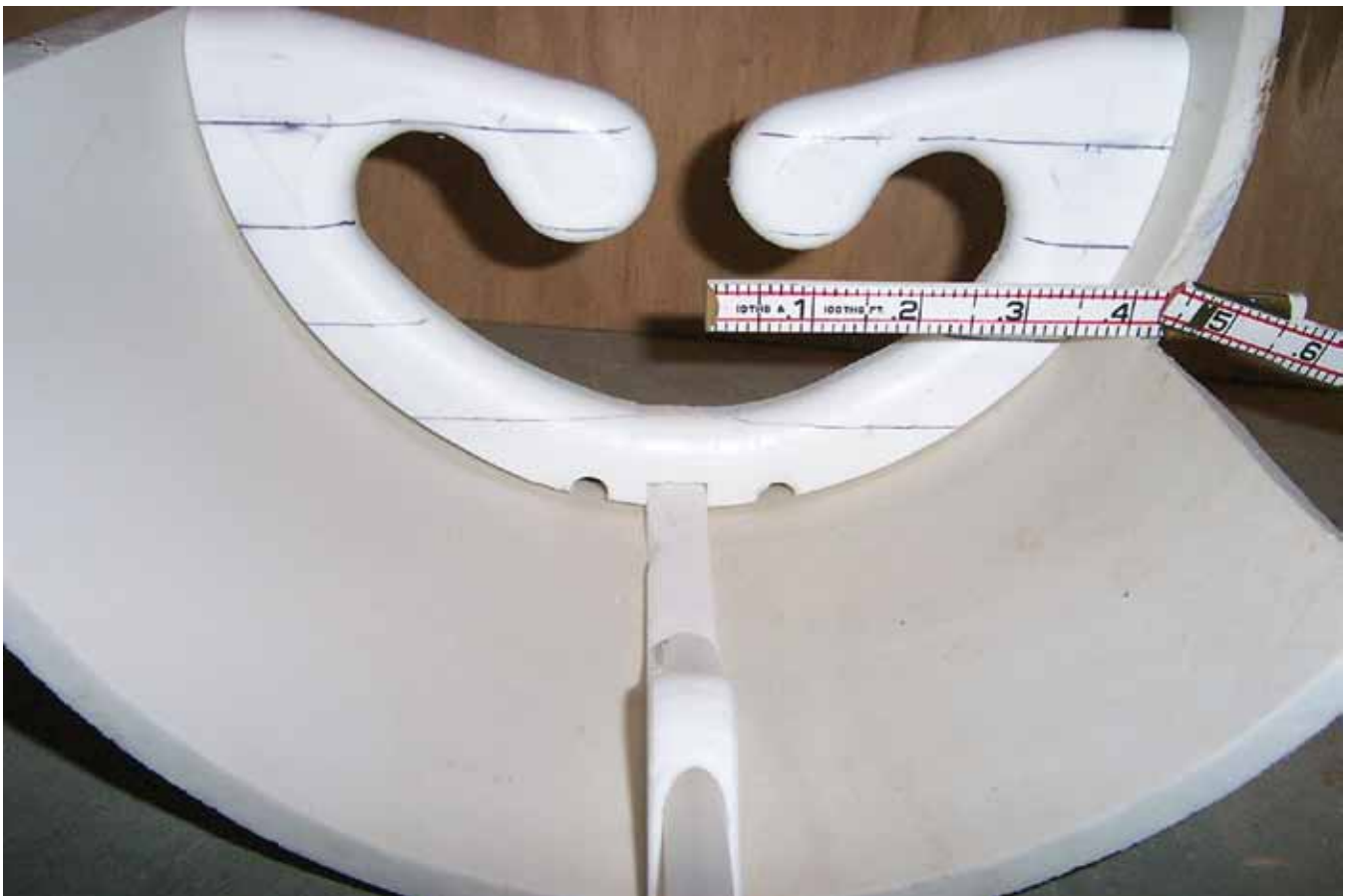
Figure 12. Static mixer mounted in a cut-out section of 12-inch-diameter plastic pipe.
