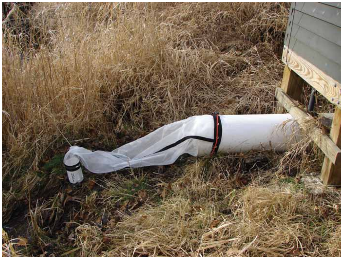
Figure 16. Plankton net attached to the outfall of the primary highway-runoff monitoring site on Interstate 495, Boxborough, Massachusetts.
