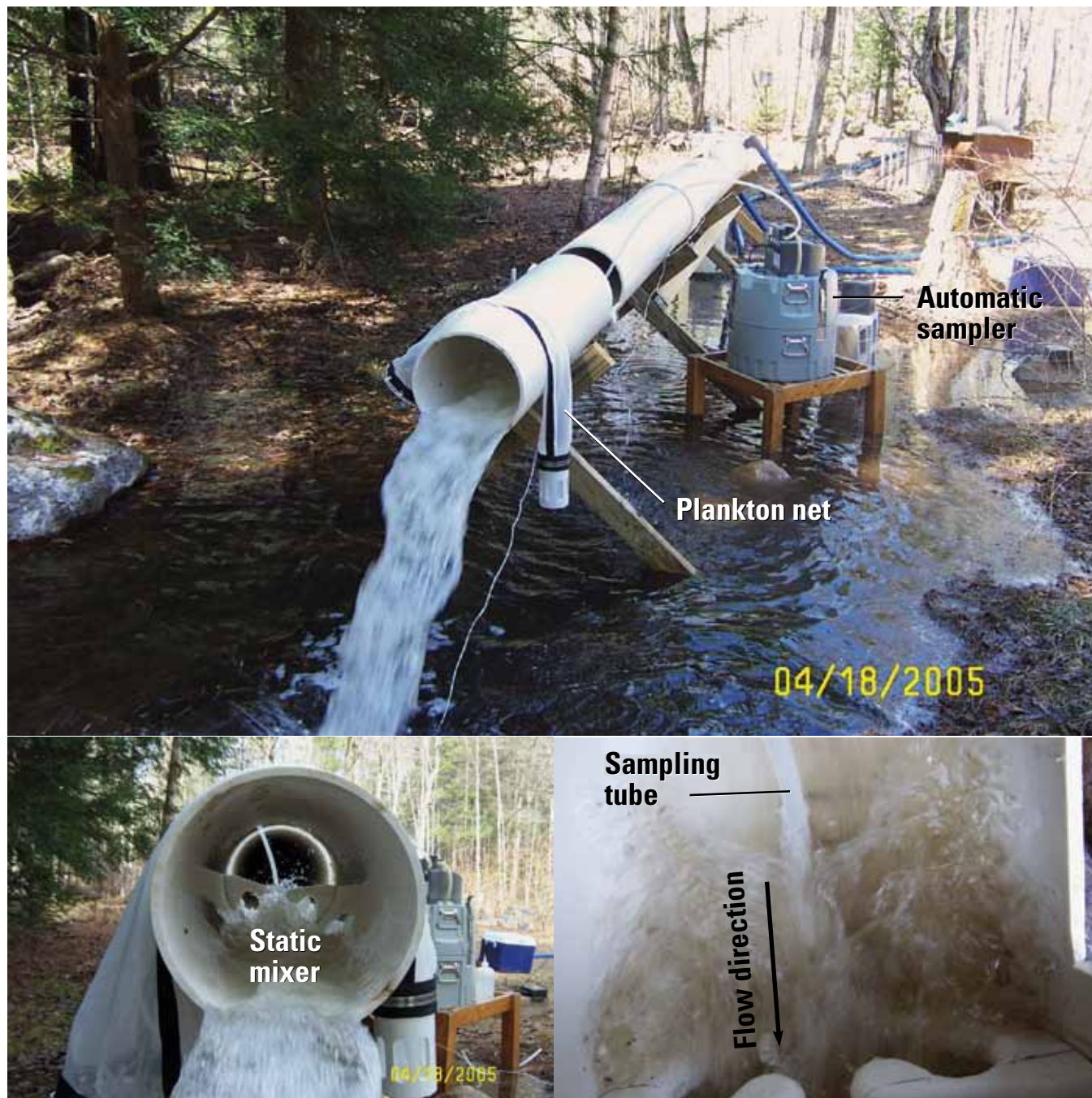
Figure 14. Test pipe and sampling equipment (top) where the static mixer assembly was tested; (lower left) looking upstream; and (lower right) turbulence created by the static mixer at the sampler intake location. The plankton net, which was used to collect the total mass of sediment at the end of the test pipe during the experiment, is draped over the end of the pipe in the photograph.
