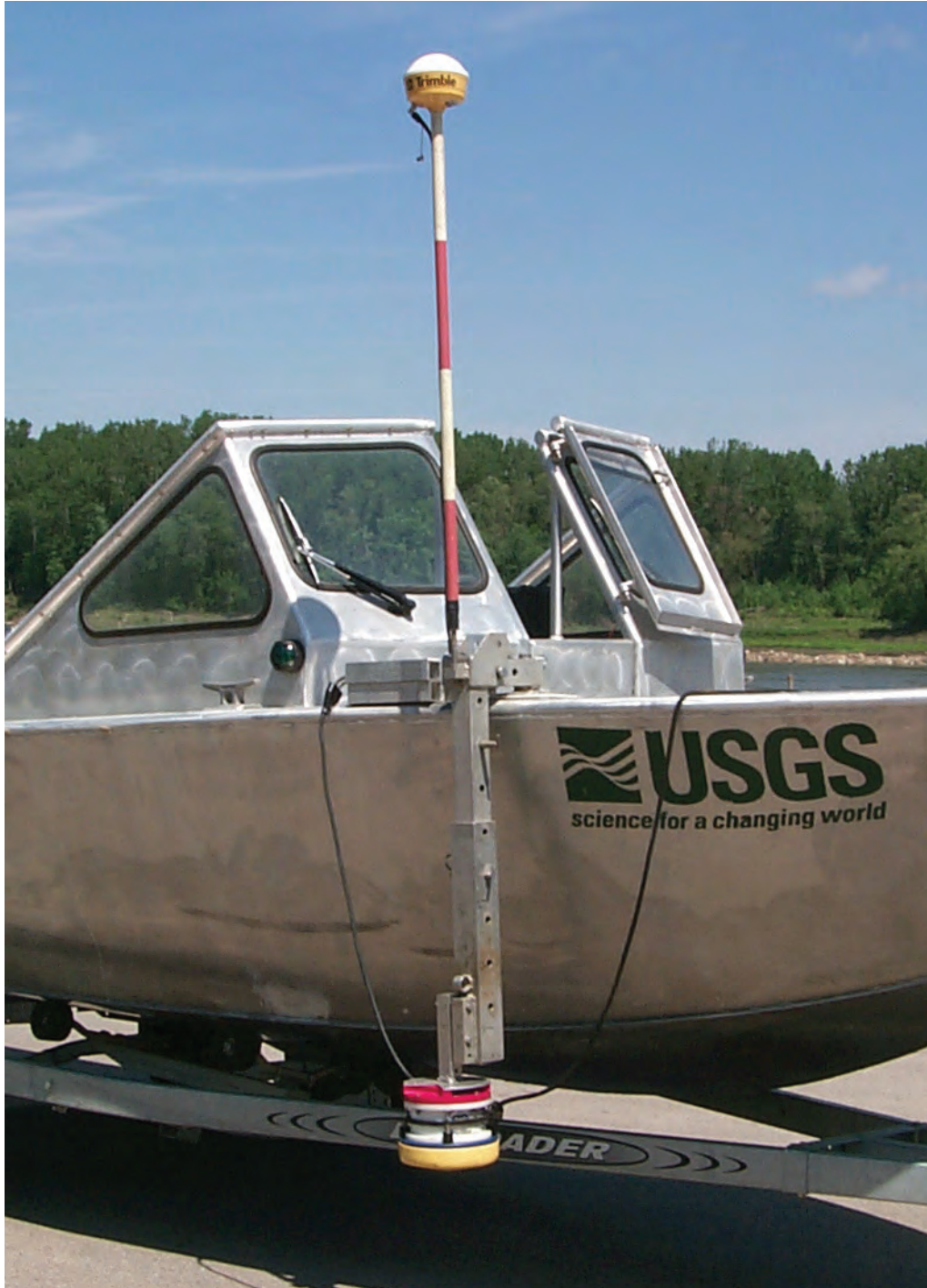
Figure 6. The Teledyne RD Instruments Rio Grande acoustic Doppler current profiler and differential Global Positioning System antenna on the starboard side of the U.S. Geological Survey Missouri Water Science Center survey boat.
