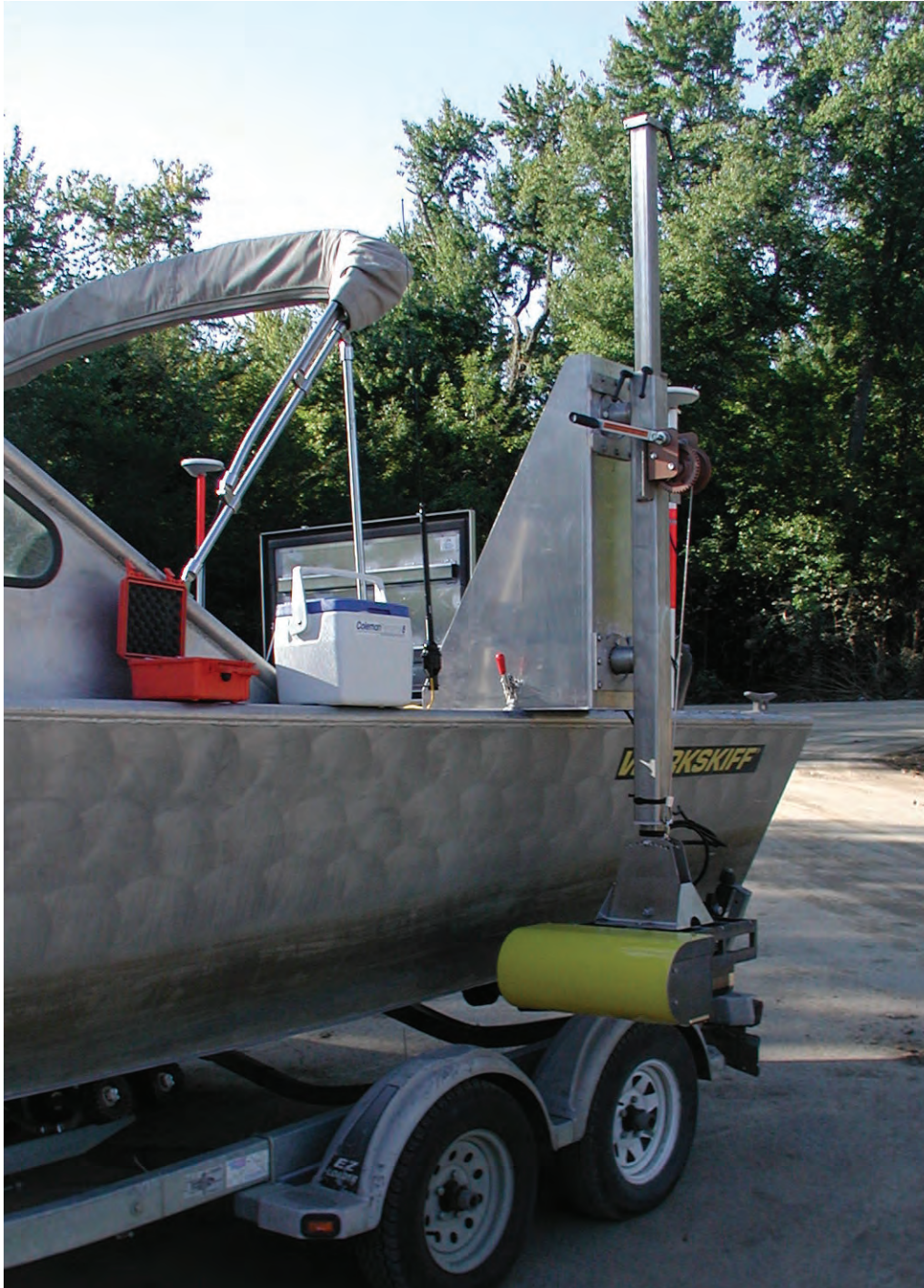
Figure 4. The RESON SeaBat™ 7125 multibeam echo sounder system on the port side of the U.S. Geological Survey Missouri Water Science Center survey boat.
