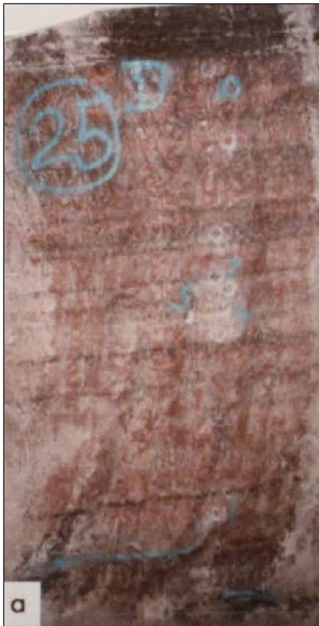
Figure 24. Photograph showing sylvite-bearing banded halite in Patience Lake Member of the Prairie Evaporite in ore zone A of the Cory Mine. Modified from Boys (1990); used with permission from the Department of Geological Sciences at the University of Saskatchewan.
