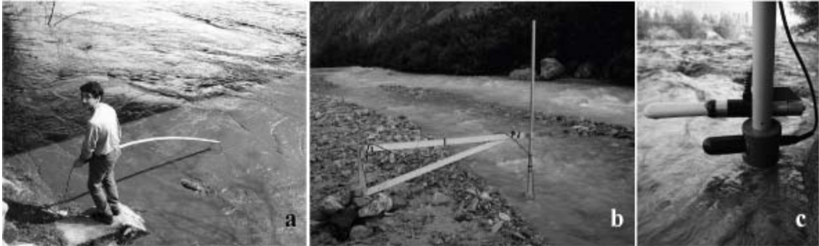
Figure 1a. The hydrophone hanging from the end of a rod (Isère River)
