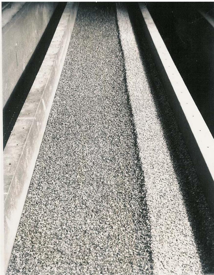
**Figure 1.** A section of the equilibrium channel at the completion of the experiment. The flow direction is towards the top of the page.
