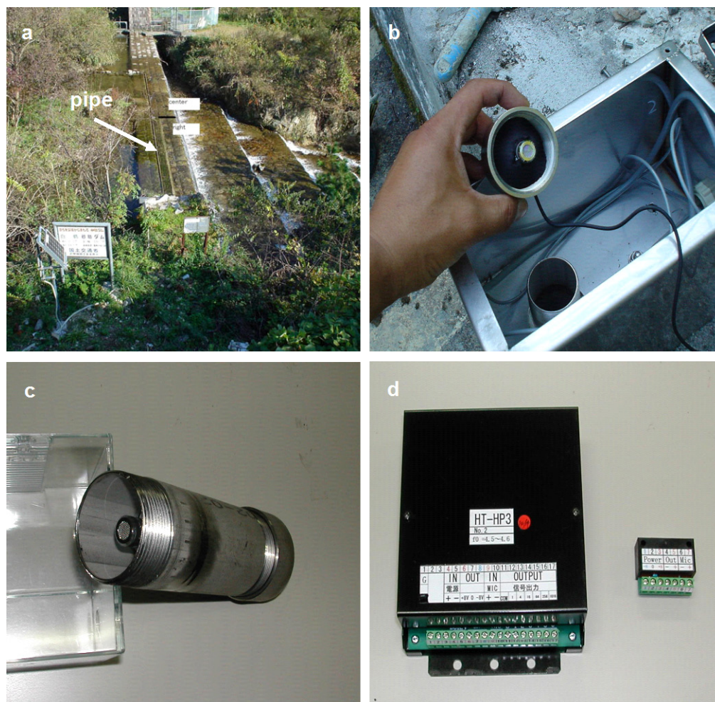
Figure 1. The Japanese acoustic bedload monitoring system consists of a half-buried pipe installed across the river-bed (a) exemplified by the Sumiyoshi River downstream of its tributary, the Nishi-takiga-tani; the waterproof pipe contains a microphone (b) and a preamplifier (c), from which acoustic signals are transmitted by cable to a converter (d).
