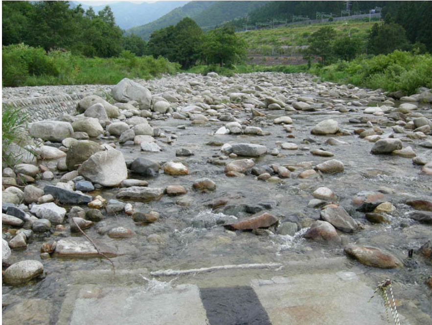
Figure 4. For calibration of bedload discharge the pipe geophone is positioned immediately in front of the slot opening of a Reid slot sampler. Upstream view on the Uonogawa (Tsuchitaru tributary).
