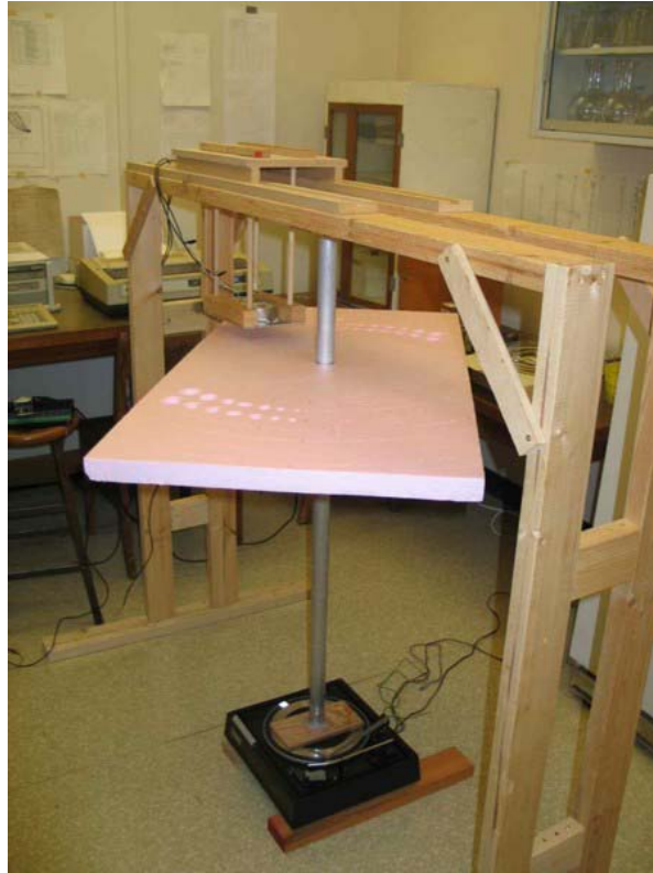
Figure 2: Rotating platter apparatus, designed to control particle trajectory and velocity.
