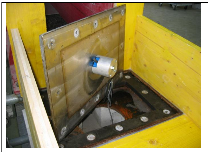
Figure 2. Geophone sensor in metal case fixed to the steel plate from underneath.
