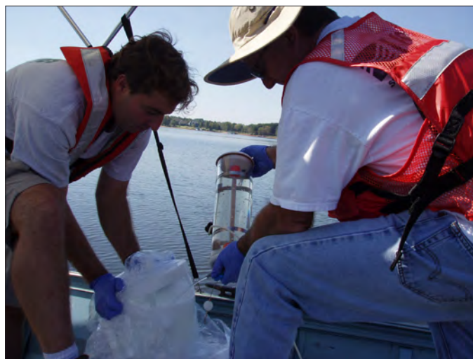
USGS field personnel collecting water sample in Lake William C. Bowen using a Van Dorn sampler and churn.
