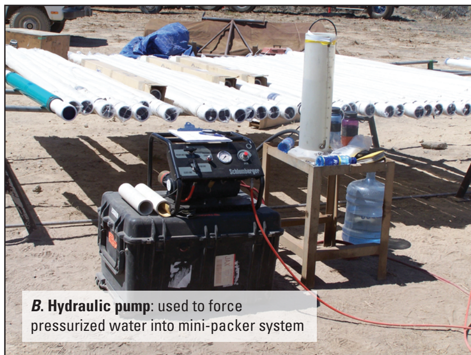
Figure 7. Testing a casing joint for leaks using (A) mini-packer system to force pressurized water across the joint and (B) hydraulic pump to pressurize water, Idaho National Laboratory, Idaho.
