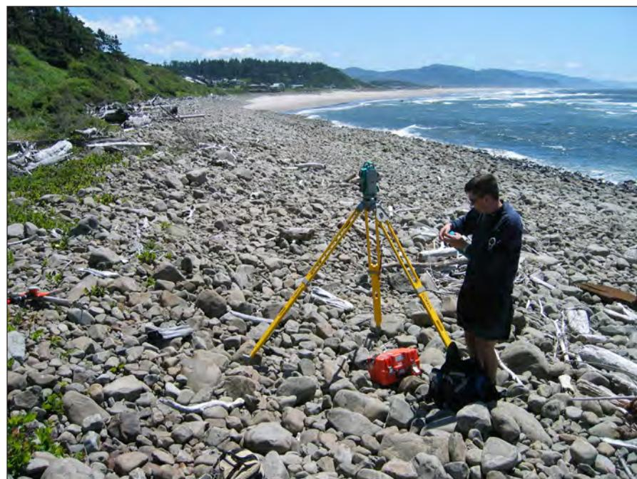
**Figure 2.** Natural cobble beach on the Oregon coast, being surveyed and with the cobble sizes measured to serve in the design of the artificial cobble berm for shore protection in Cape Lookout State Park.
