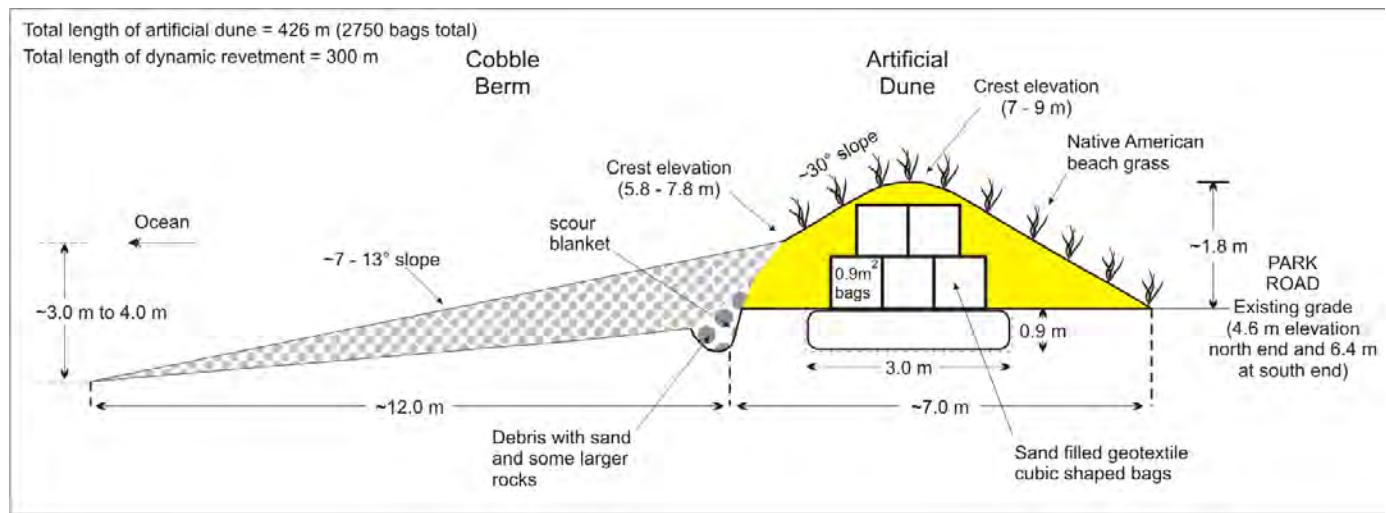
**Figure 5.** Design for the cobble berm and reinforced foredune to protect Cape Lookout State Park from erosion and flooding. The elevations are referenced to the NAVD 88 datum.
