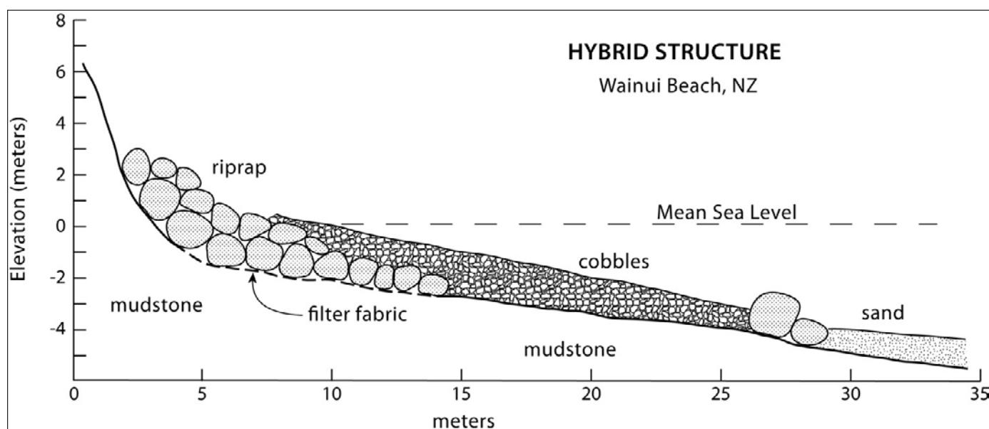
**Figure 8.** Hybrid "Design with Nature" approach for protecting a bluff from erosion, consisting of a cobble berm backed by a natural form of boulder revetment.
