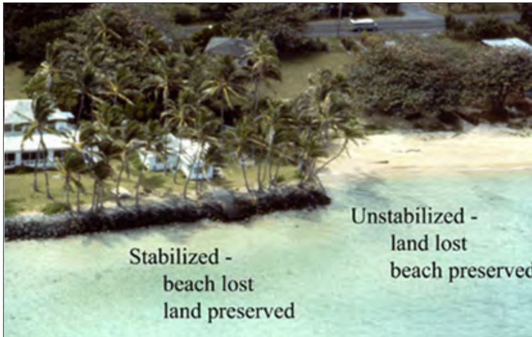
Figure 2. Example of the impact of seawalls on beaches under conditions of ‘passive’ erosion. Photo Credit Chip Fletcher (Hawaii).
