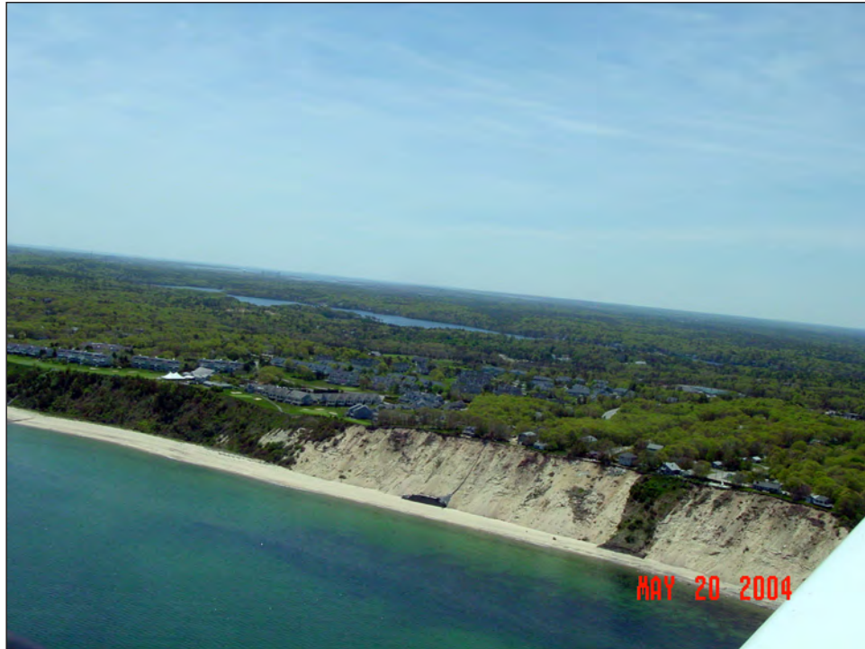
Figure 5. An eroding coastal bank/bluff along the south shore of Massachusetts providing source sand to the fronting and downdrift beaches.
