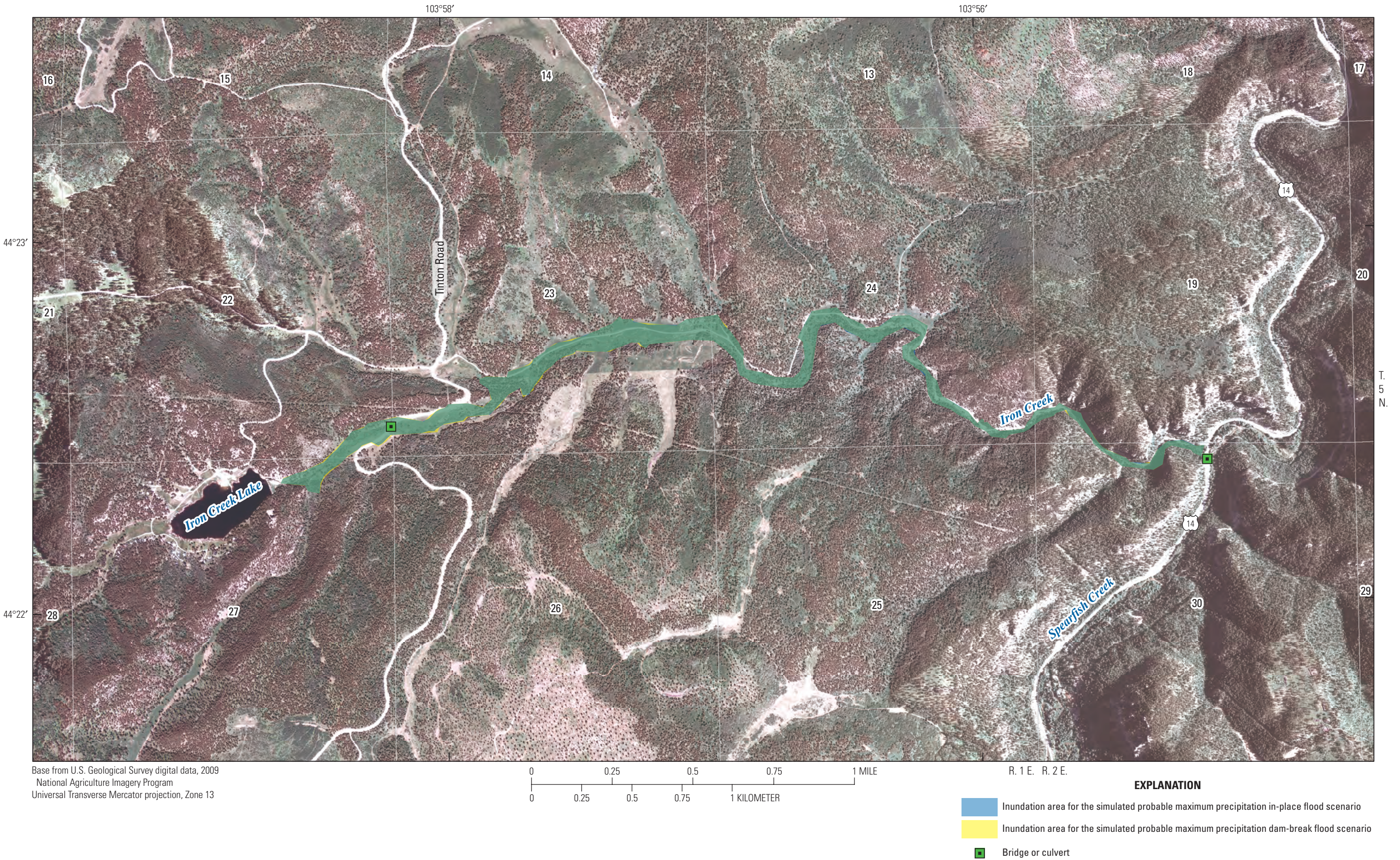
Figure 18. Flood inundation map for a simulated dam break from a probable maximum precipitation inflow design flood for Iron Creek Lake.
