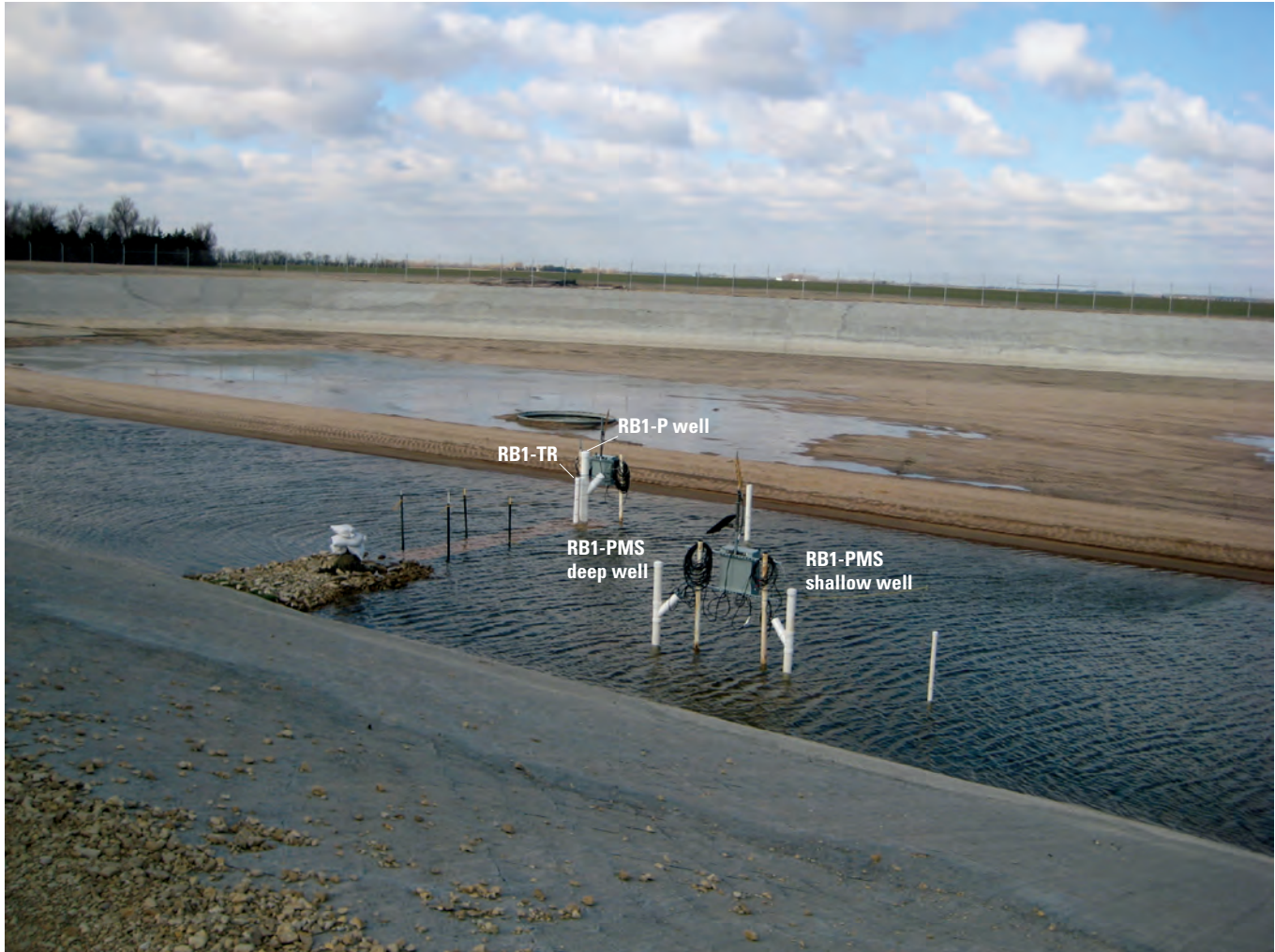
Figure 3. RB1-TR, RB1-P well, and RB1-PMS wells installed along the eastern edge of the original RB1 basin. Photographed from the northeast during artificial recharge when trench was flooded with treated surface water.
