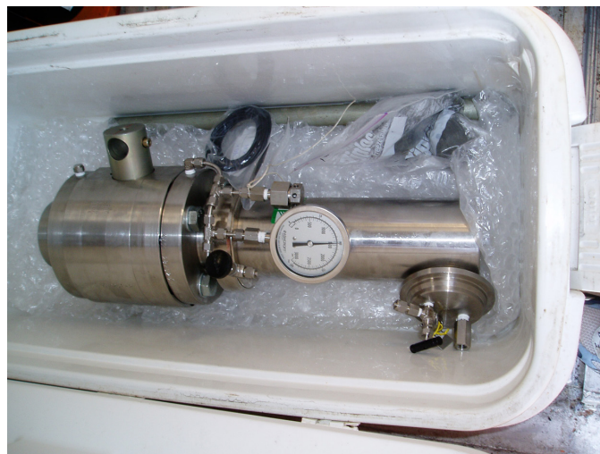
Figure 3-5. A Parr pressure vessel fitted with a HYACINTH ball valve for shipping short lengths of core under full in situ pressures.
