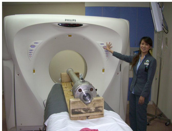
Figure 3-2. HYACINTH pressure core inside aluminum storage chamber about to undergo X-ray computed tomography scan at Gleneagles Hospital in Singapore.
