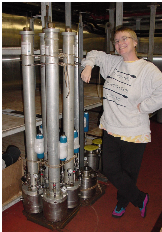
Figure 3-1. Five HYACINTH pressure cores stored in the reefer on the JOIDES Resolution ready for shore-based studies in Singapore.
