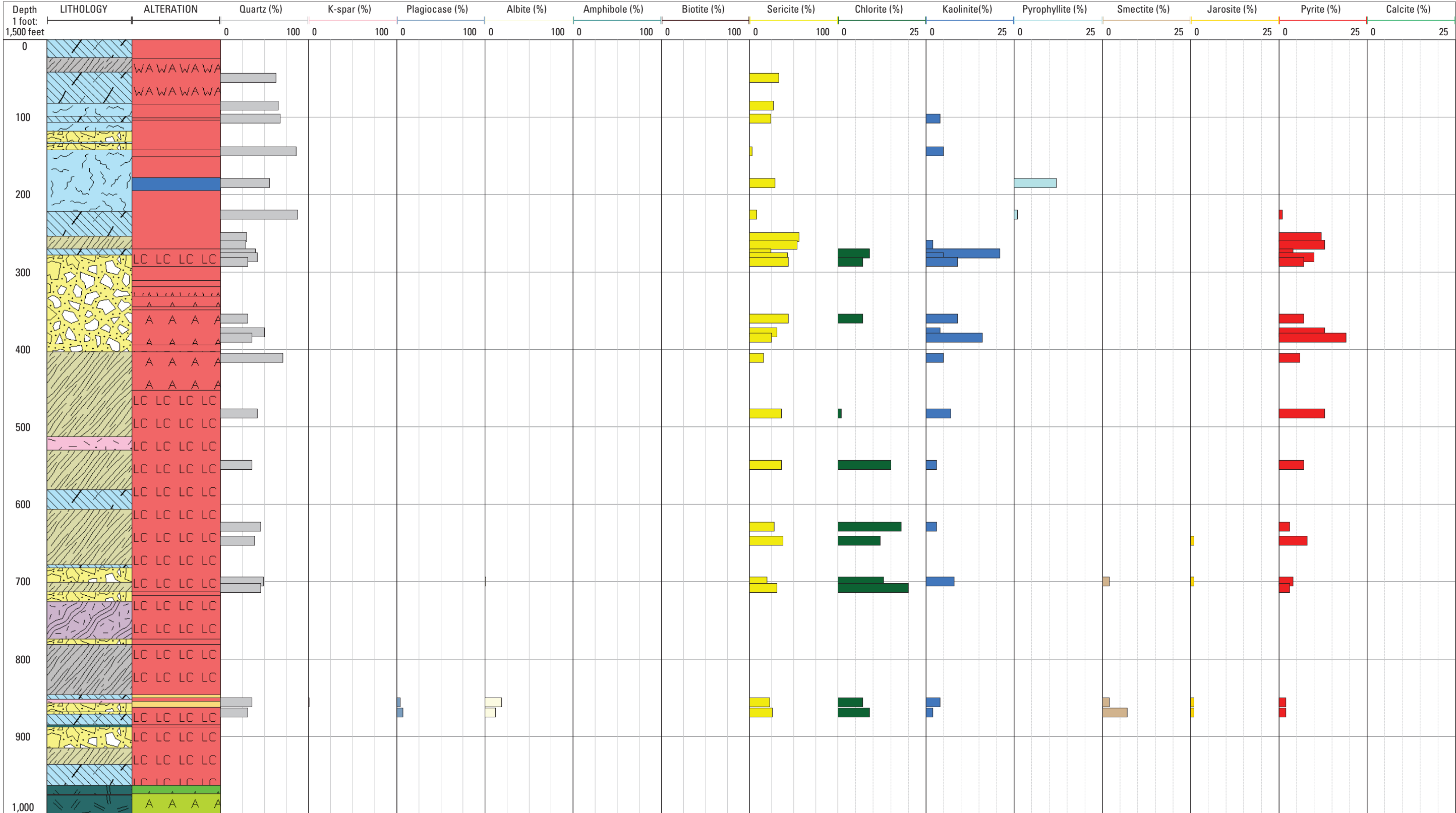
Figure 4. Core logs showing lithology, alteration assemblages, and quantitative mineralogy in drill holes A , WP1. B , WP2. C , WP3. D , WP4. E , HCBW1. F , HCBW3. See Appendix A for key to all lithology and alteration types.
