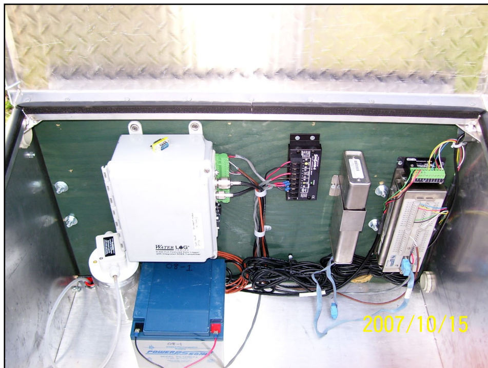
Figure 9. A, Instrumentation shelter and B, arrangement of data-collection instruments at U.S. Geological Survey well 441226069502201 in West Gardiner, Maine.
