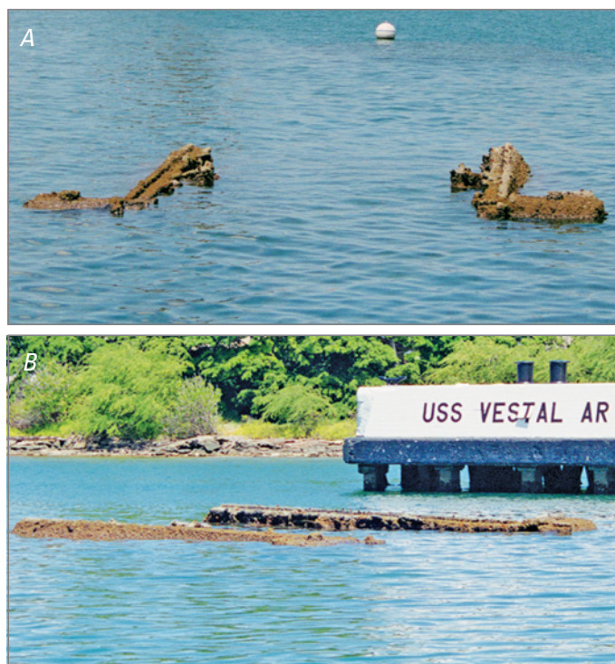
Figure 29. Views of the top edges of turret 2 during a very low tide in 2000. The top of the turret and guns were removed in 1943. A, The turret as viewed from the USS Arizona Memorial toward the bow. The rangefinder projections are visible at the breech (near) end of the turret. The port tilt between the two forward ends measures about 0.5^\circ ; the port tilt across the aft ends measures 1.25^\circ . A portion of photo DN-SC-02-05621, dated June 3, 2000 from www.defenseimagery.mil/ . B, The turret as viewed from the port side looking toward Ford Island, with the aft tilt visible. The port side edge has an aft tilt of about 1.5^\circ ; the starboard side about 1.3^\circ . A portion of photo DN-SC-02-05620, dated June 3, 2000, from www.defenseimagery.mil/ . The tilts were determined from measurements made on March 4, 2008.
