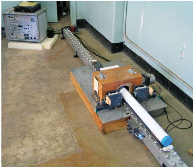
Figure 14. The USGS multisensor core logger set up in Navy Building 42, Ford Island, during the drilling operations. In this photo, an enameled steel Shelby tube is being scanned. The tube travels along the track from lower right to upper left.
