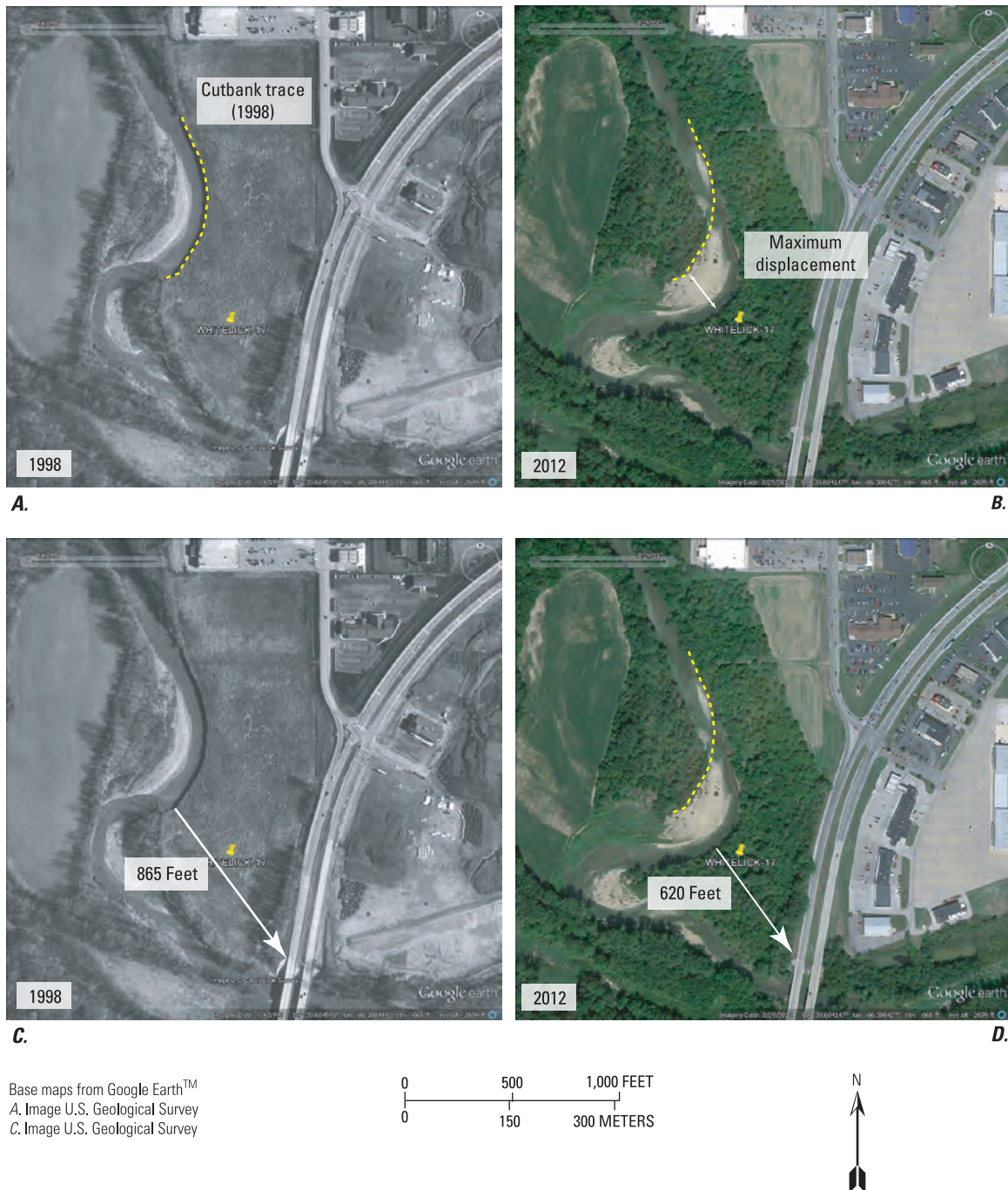
Figure 3. The steps taken to document channel-migration rates for a site along White Lick Creek at Mooresville, Indiana. A trace of the cutbank was added to the early (1998) image (A), the general location of maximum channel-displacement was identified in the late (2012) image (B), and distance measurements to a common reference point were completed for the early and late images (C and D).
