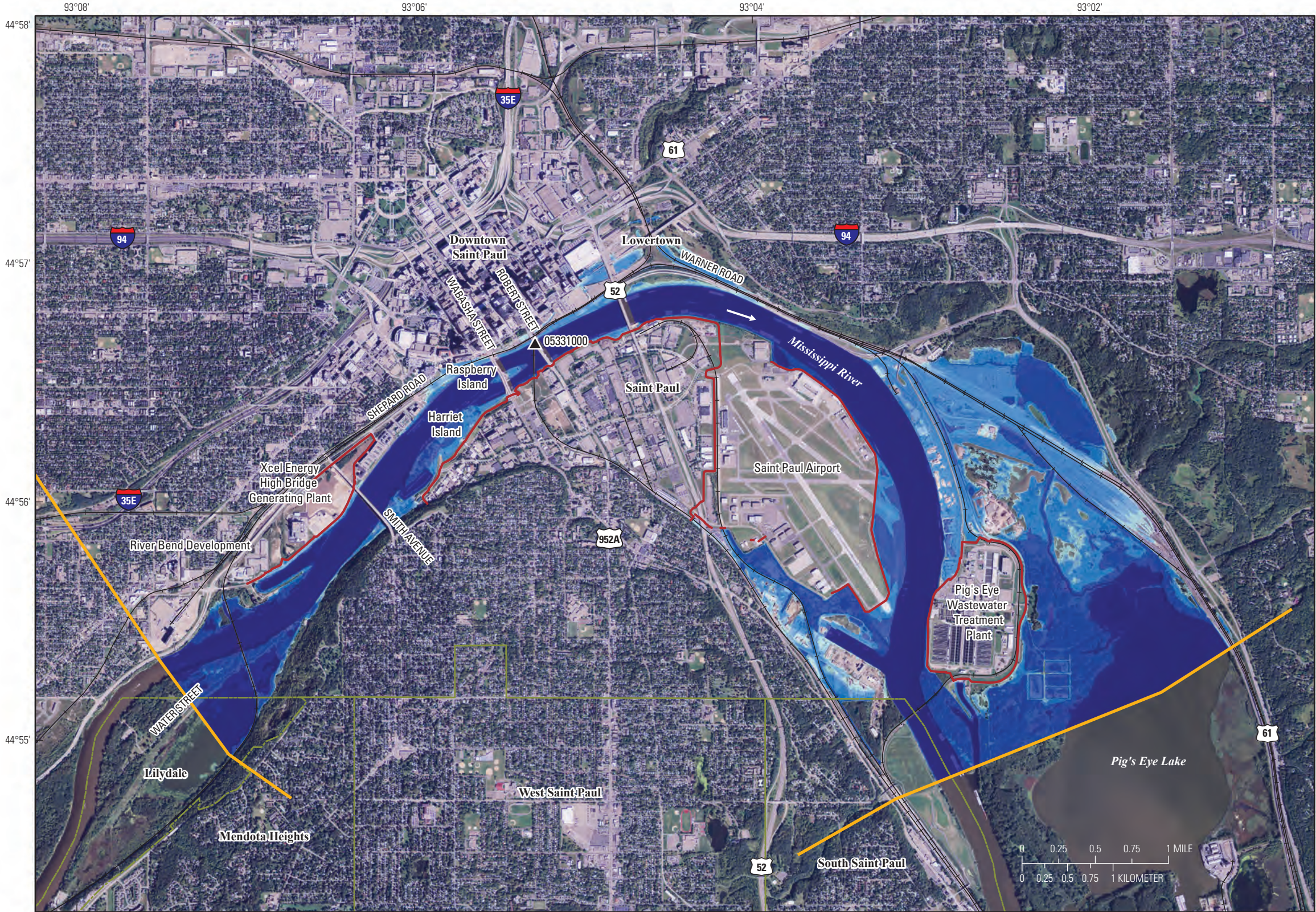
Sheet 15. Flood-inundation map of the Mississippi River at Saint Paul, Minnesota, at the U.S. Geological Survey streamgage 05331000 for a corresponding stage of 23.0 feet and an elevation of 706.8 feet above North American Vertical Datum of 1988.
