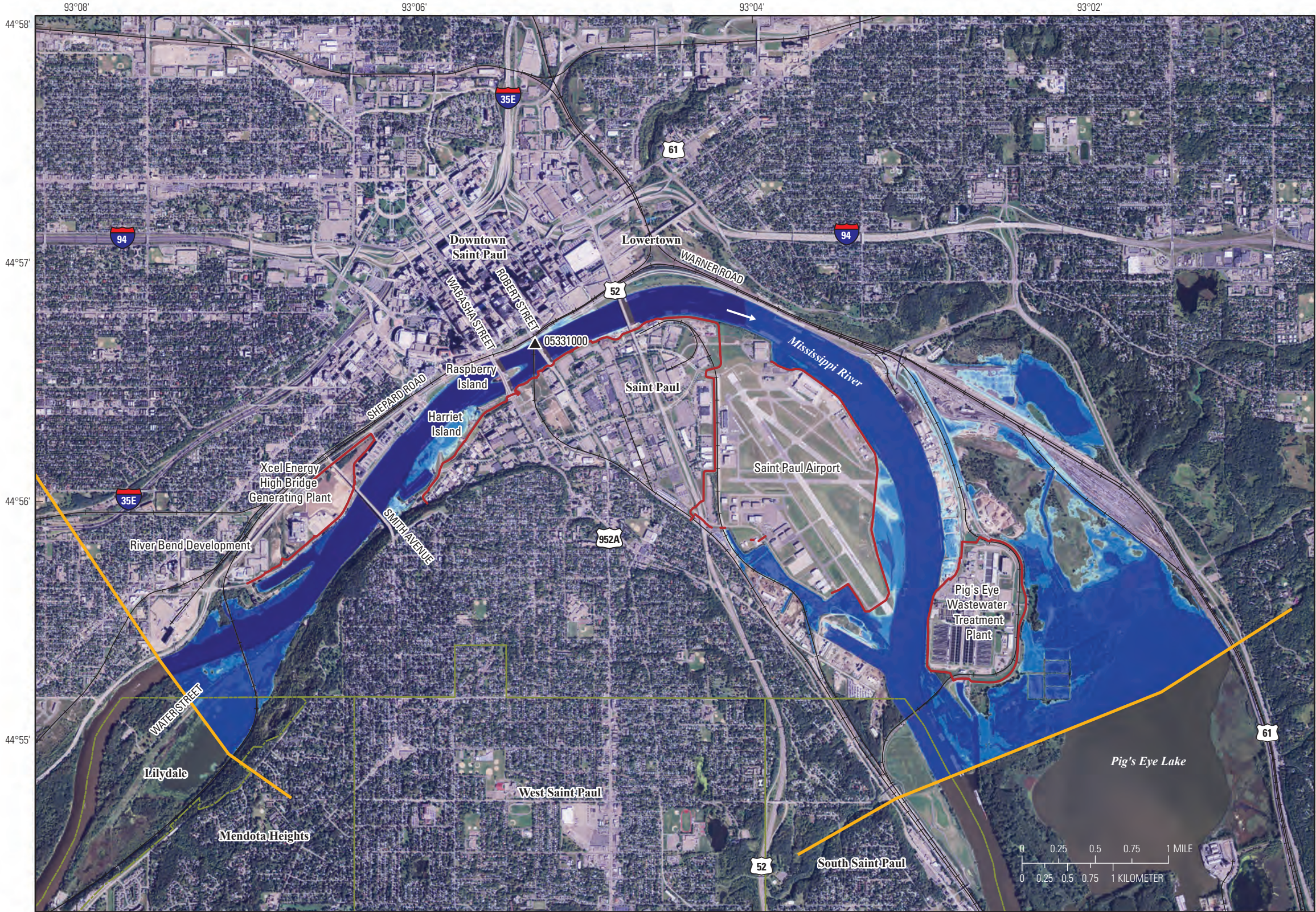
Sheet 11. Flood-inundation map of the Mississippi River at Saint Paul, Minnesota, at the U.S. Geological Survey streamgage 05331000 for a corresponding stage of 19.0 feet and an elevation of 702.8 feet above North American Vertical Datum of 1988.
