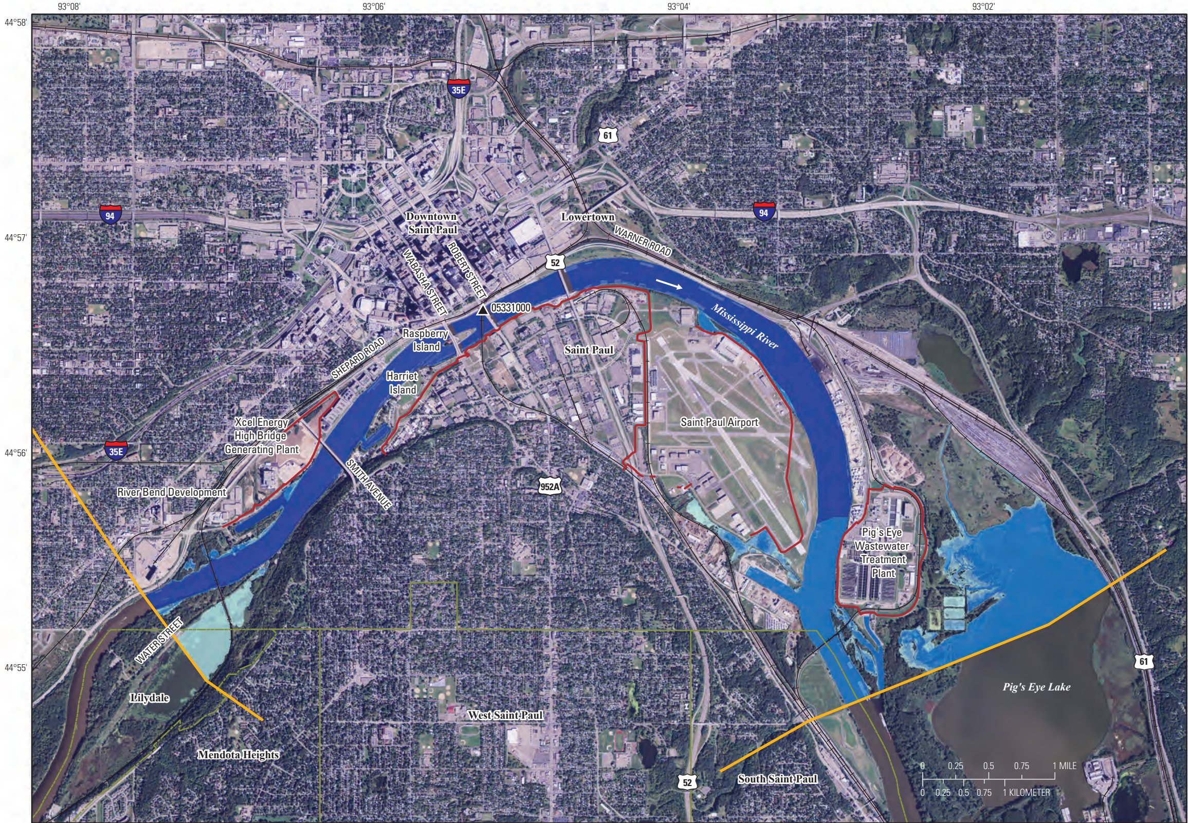
Sheet 2. Flood-inundation map of the Mississippi River at Saint Paul, Minnesota, at the U.S. Geological Survey streamgage 05331000 for a corresponding stage of 10.0 feet and an elevation of 693.8 feet above North American Vertical Datum of 1988.
