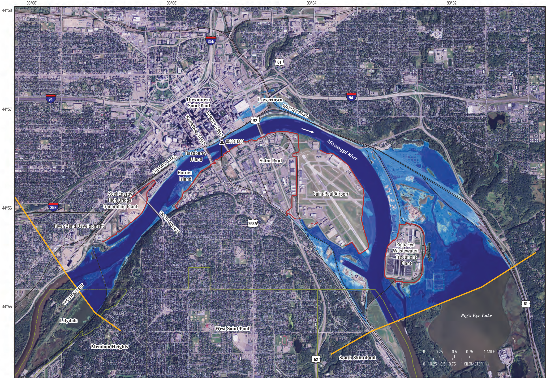
Sheet 16. Flood-inundation map of the Mississippi River at Saint Paul, Minnesota, at the U.S. Geological Survey streamgage 05331000 for a corresponding stage of 24.0 feet and an elevation of 707.8 feet above North American Vertical Datum of 1988.
