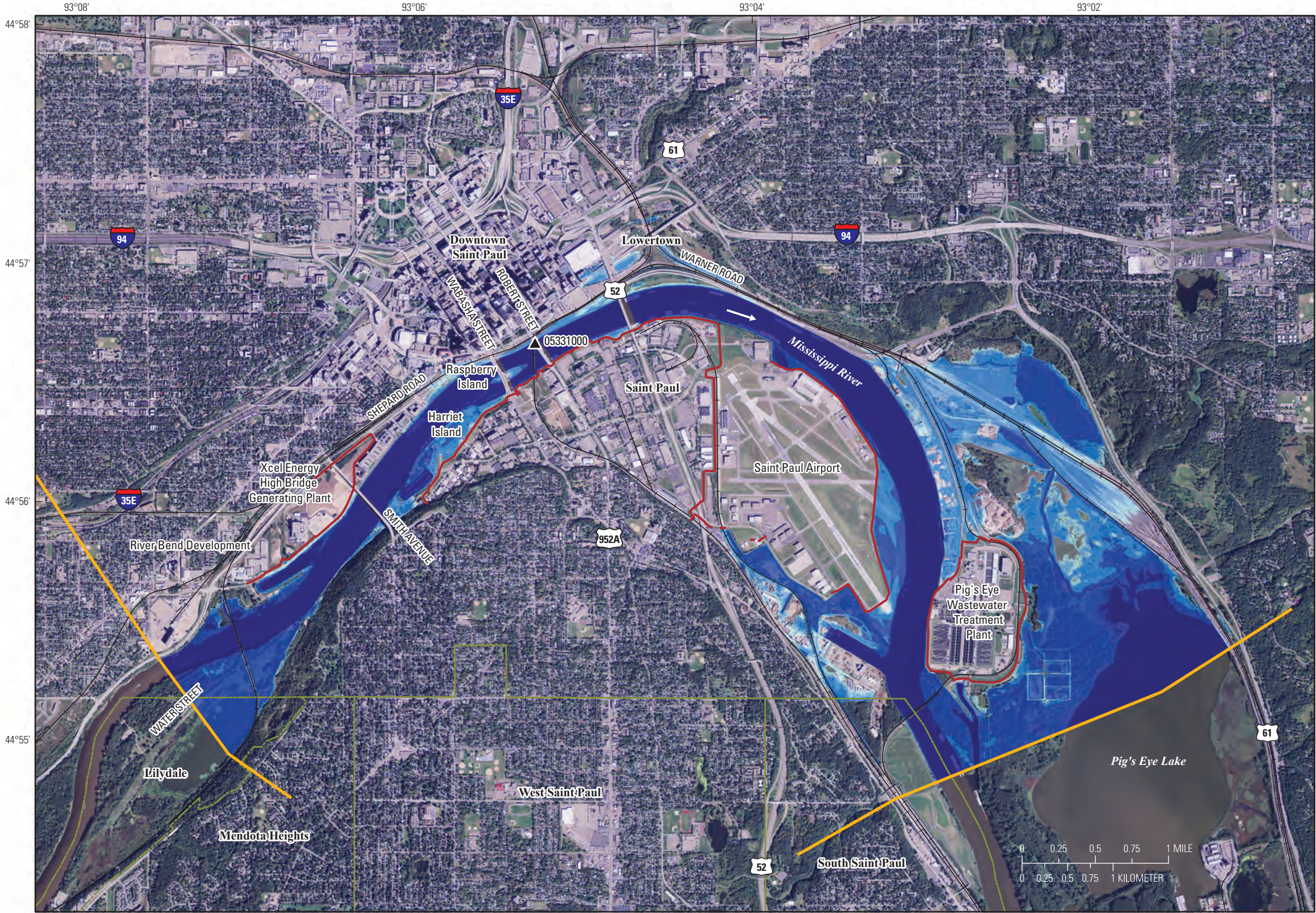
Sheet 14. Flood-inundation map of the Mississippi River at Saint Paul, Minnesota, at the U.S. Geological Survey streamgage 05331000 for a corresponding stage of 22.0 feet and an elevation of 705.8 feet above North American Vertical Datum of 1988.
