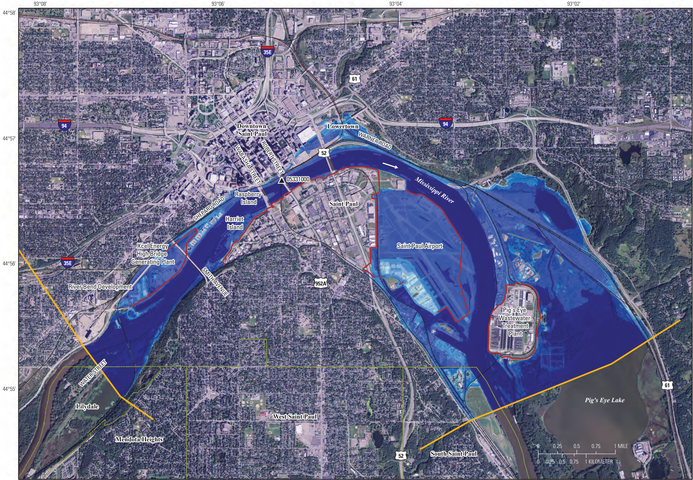
Sheet 22. Flood-inundation map of the Mississippi River at Saint Paul, Minnesota, at the U.S. Geological Survey streamgage 05331000 for a corresponding stage of 30.0 feet and an elevation of 713.8 feet above North American Vertical Datum of 1988.
