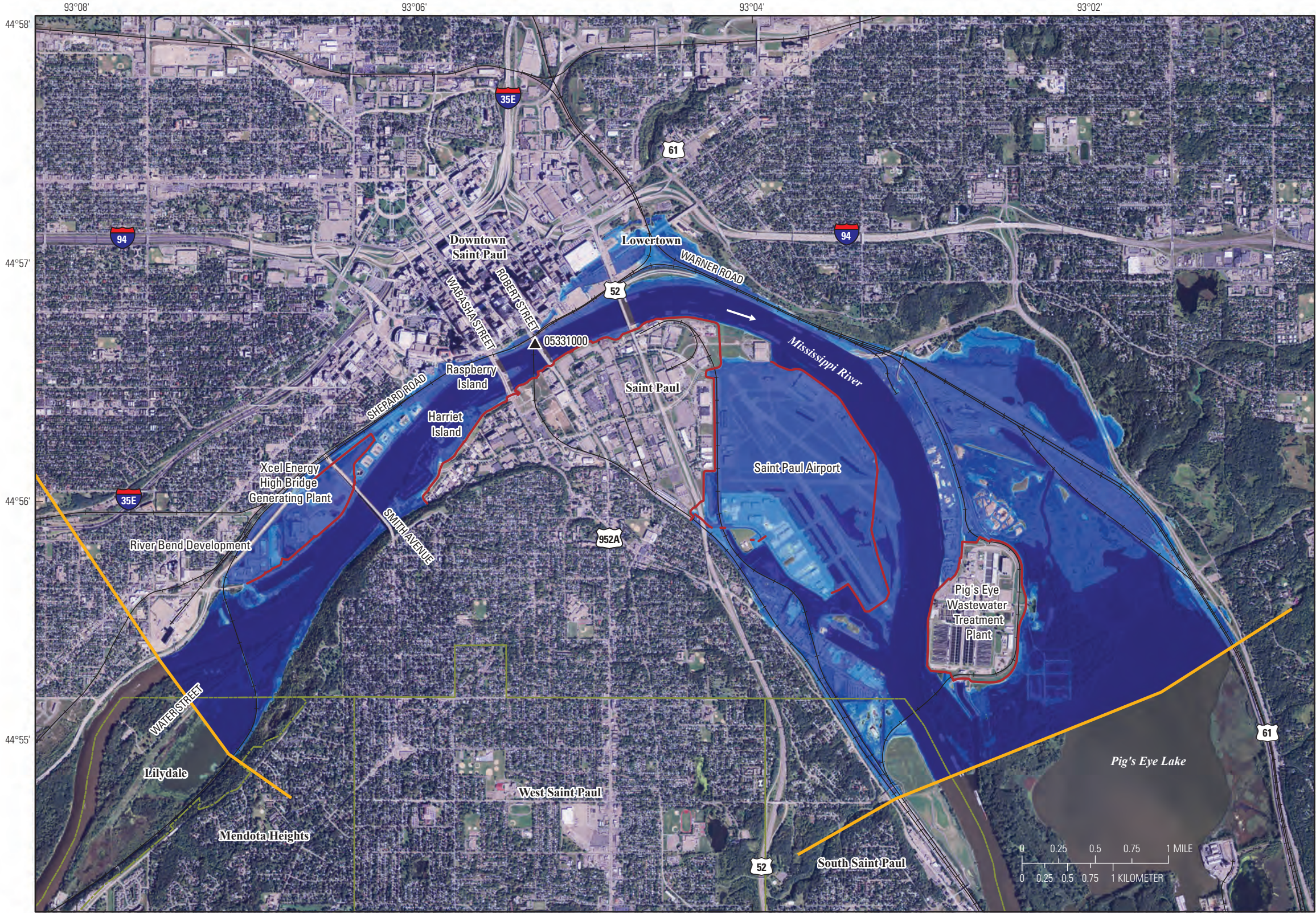
Sheet 23. Flood-inundation map of the Mississippi River at Saint Paul, Minnesota, at the U.S. Geological Survey streamgage 05331000 for a corresponding stage of 31.0 feet and an elevation of 714.8 feet above North American Vertical Datum of 1988.
