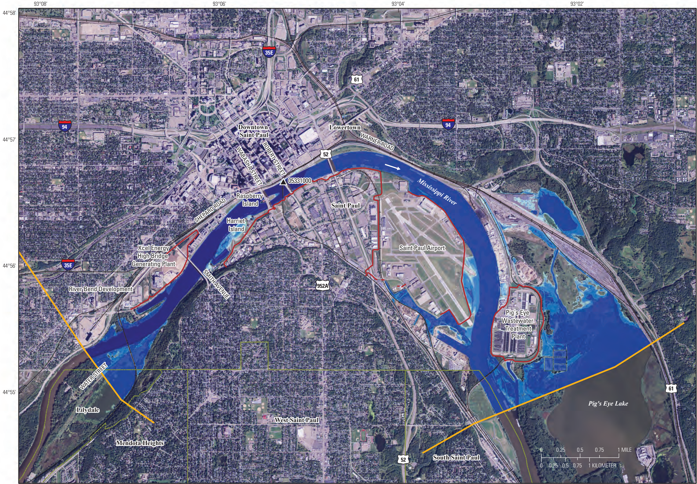
Sheet 10. Flood-inundation map of the Mississippi River at Saint Paul, Minnesota, at the U.S. Geological Survey streamgage 05331000 for a corresponding stage of 18.0 feet and an elevation of 701.8 feet above North American Vertical Datum of 1988.
