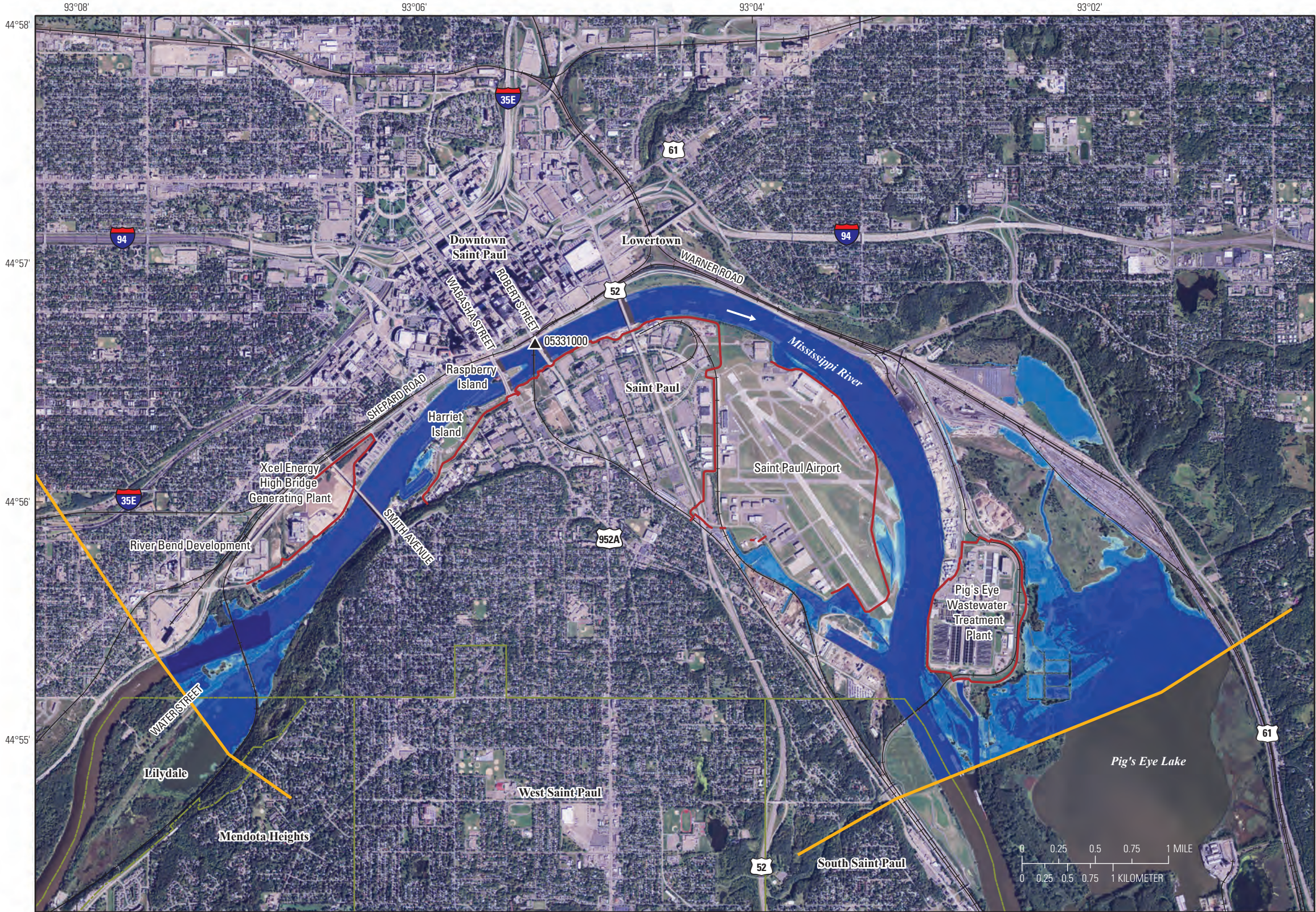
Sheet 8. Flood-inundation map of the Mississippi River at Saint Paul, Minnesota, at the U.S. Geological Survey streamgage 05331000 for a corresponding stage of 16.0 feet and an elevation of 699.8 feet above North American Vertical Datum of 1988.
