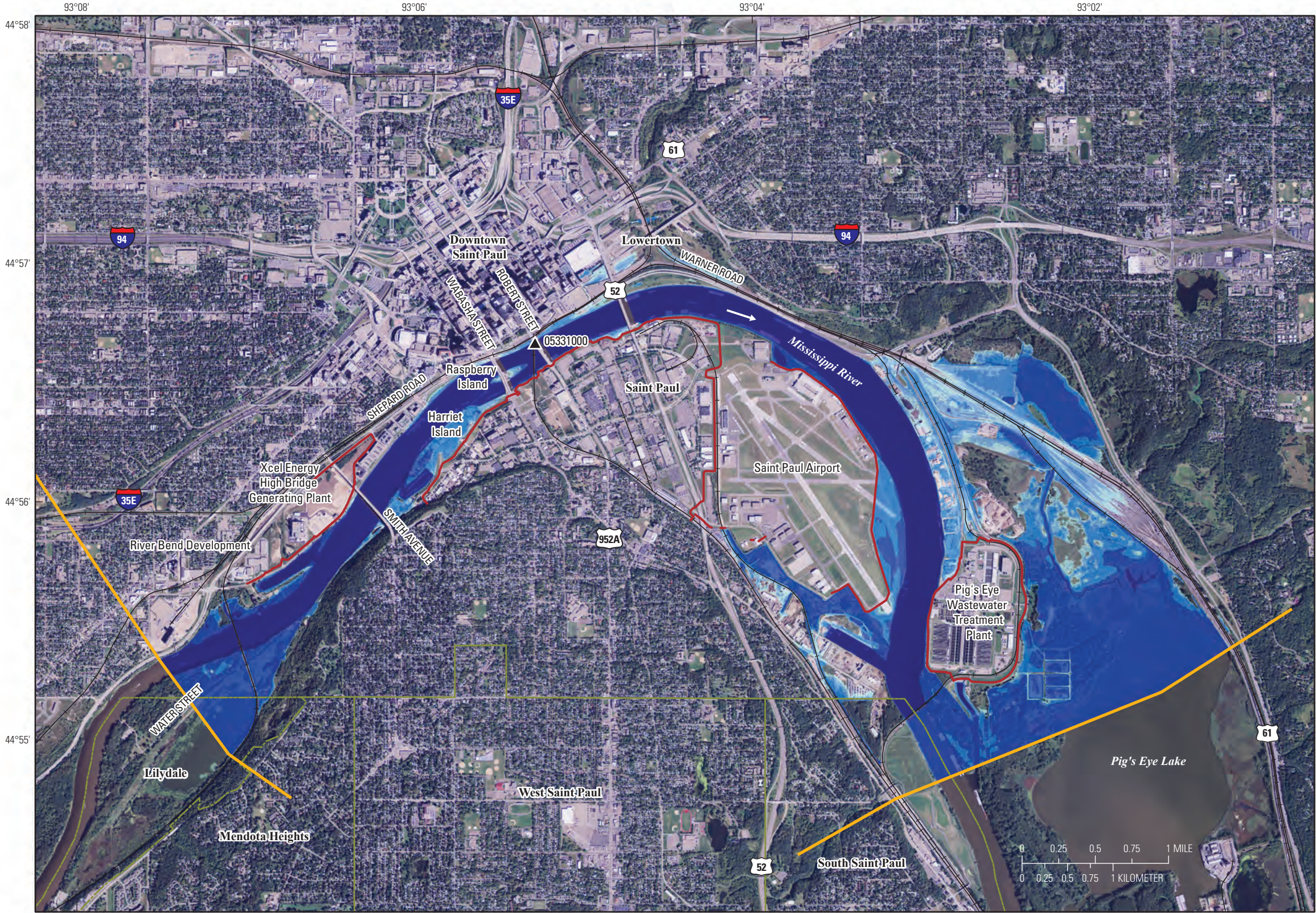
Sheet 13. Flood-inundation map of the Mississippi River at Saint Paul, Minnesota, at the U.S. Geological Survey streamgage 05331000 for a corresponding stage of 21.0 feet and an elevation of 704.8 feet above North American Vertical Datum of 1988.
