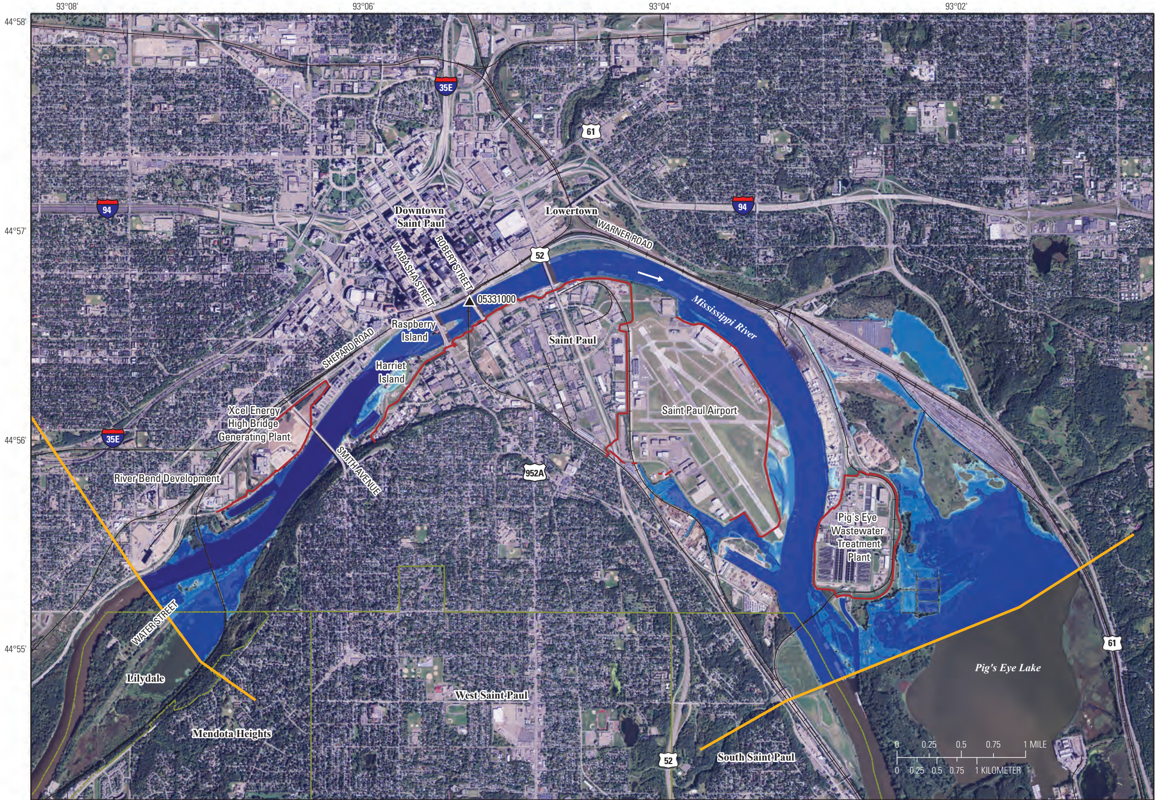
Sheet 9. Flood-inundation map of the Mississippi River at Saint Paul, Minnesota, at the U.S. Geological Survey streamgage 05331000 for a corresponding stage of 17.0 feet and an elevation of 700.8 feet above North American Vertical Datum of 1988.
