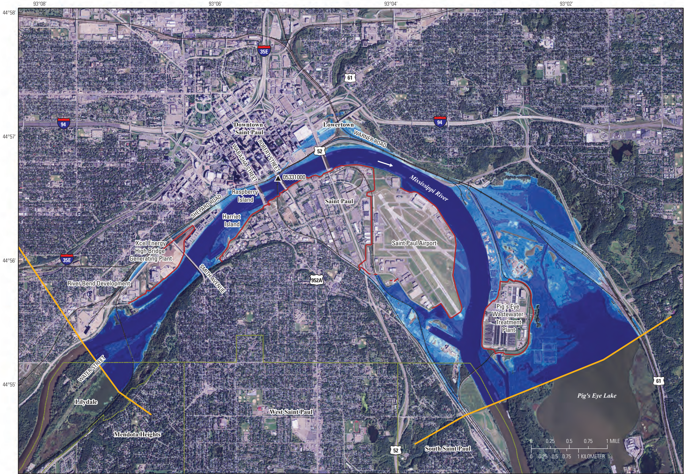
Sheet 17. Flood-inundation map of the Mississippi River at Saint Paul, Minnesota, at the U.S. Geological Survey streamgage 05331000 for a corresponding stage of 25.0 feet and an elevation of 708.8 feet above North American Vertical Datum of 1988.
