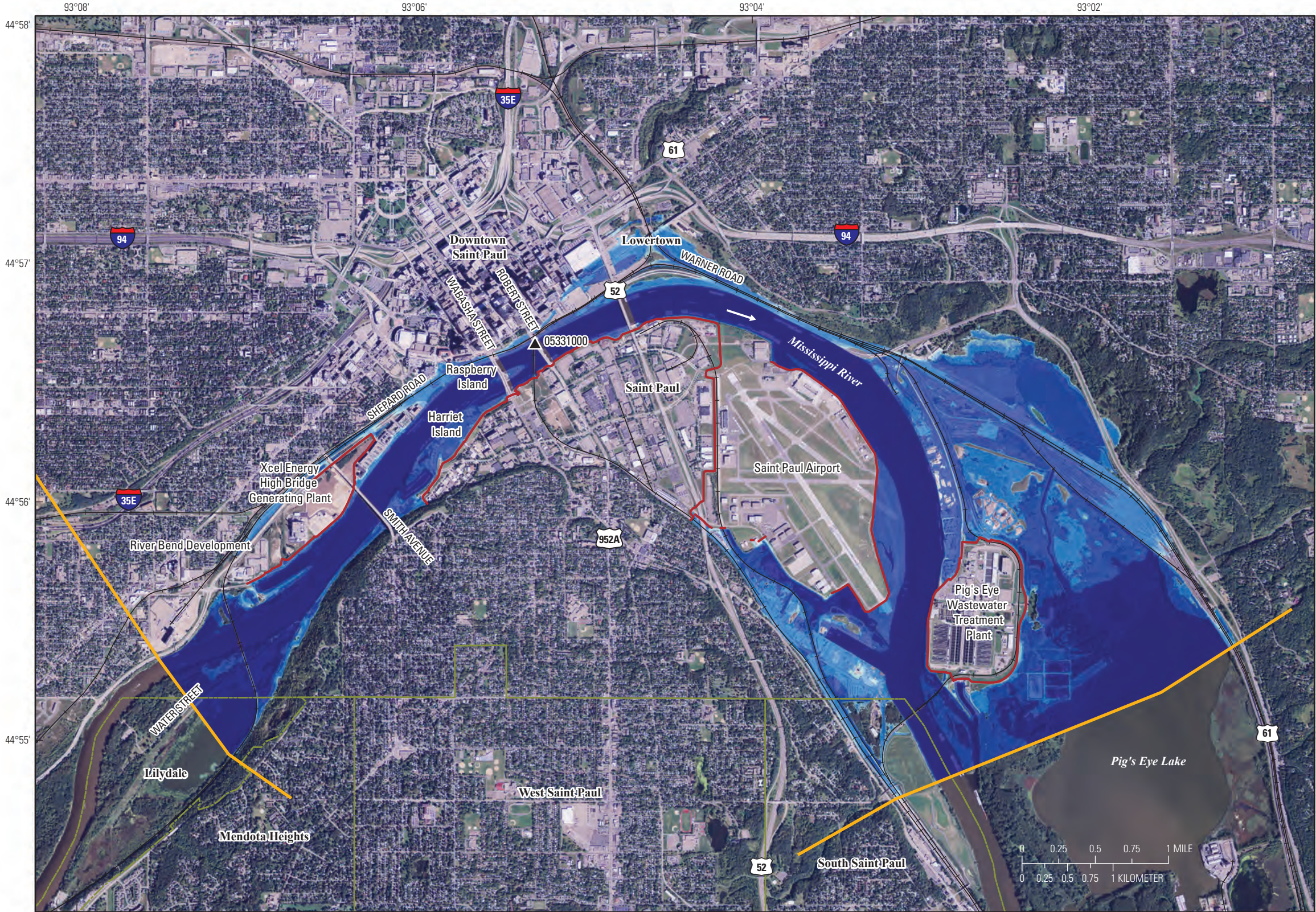
Sheet 19. Flood-inundation map of the Mississippi River at Saint Paul, Minnesota, at the U.S. Geological Survey streamgage 05331000 for a corresponding stage of 27.0 feet and an elevation of 710.8 feet above North American Vertical Datum of 1988.
