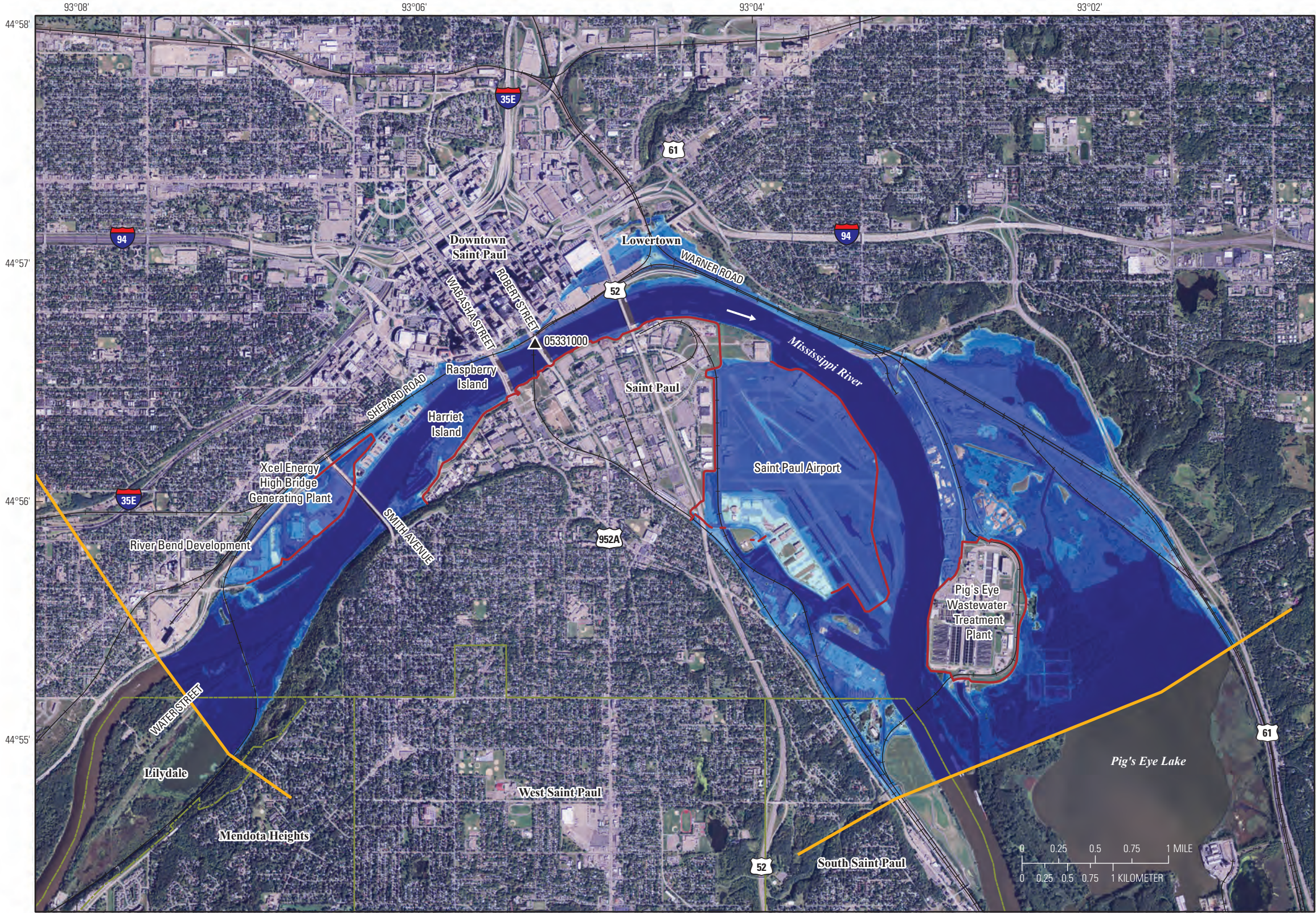
Sheet 21. Flood-inundation map of the Mississippi River at Saint Paul, Minnesota, at the U.S. Geological Survey streamgage 05331000 for a corresponding stage of 29.0 feet and an elevation of 712.8 feet above North American Vertical Datum of 1988.
