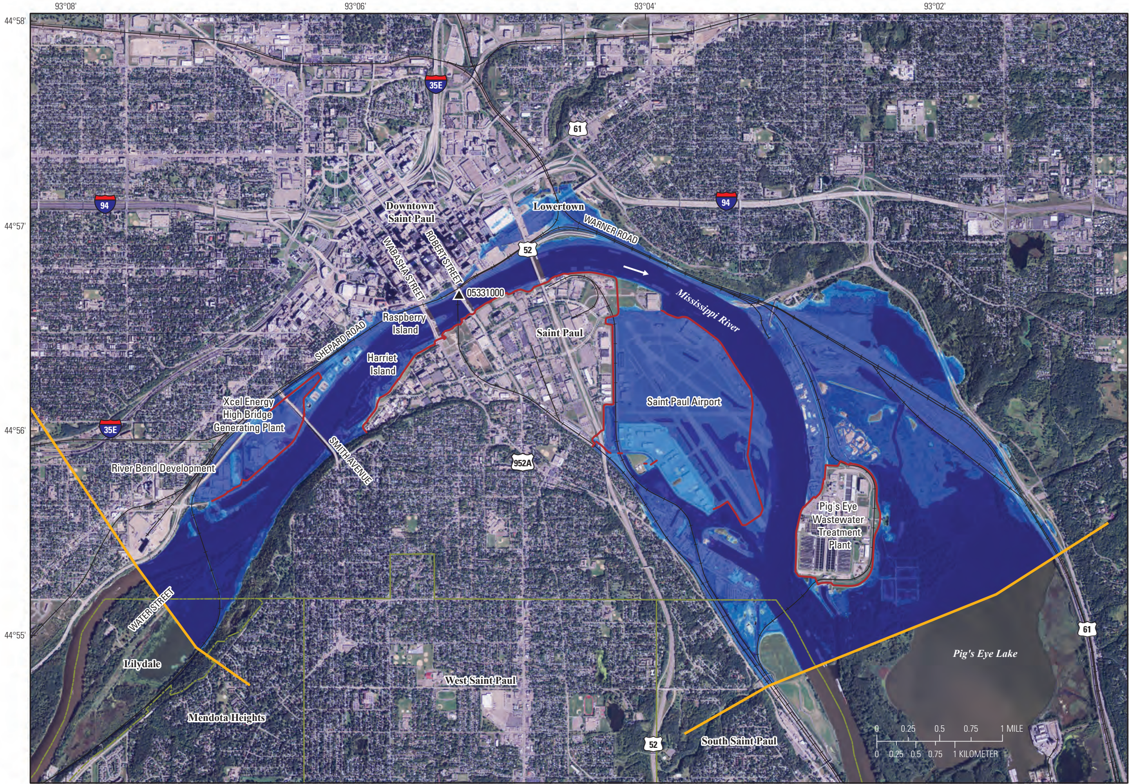
Sheet 24. Flood-inundation map of the Mississippi River at Saint Paul, Minnesota, at the U.S. Geological Survey streamgage 05331000 for a corresponding stage of 32.0 feet and an elevation of 715.8 feet above North American Vertical Datum of 1988.
