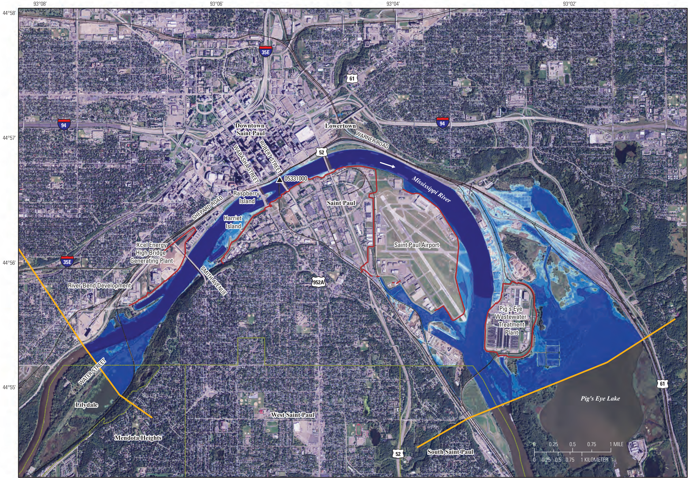
Sheet 12. Flood-inundation map of the Mississippi River at Saint Paul, Minnesota, at the U.S. Geological Survey streamgage 05331000 for a corresponding stage of 20.0 feet and an elevation of 703.8 feet above North American Vertical Datum of 1988.
