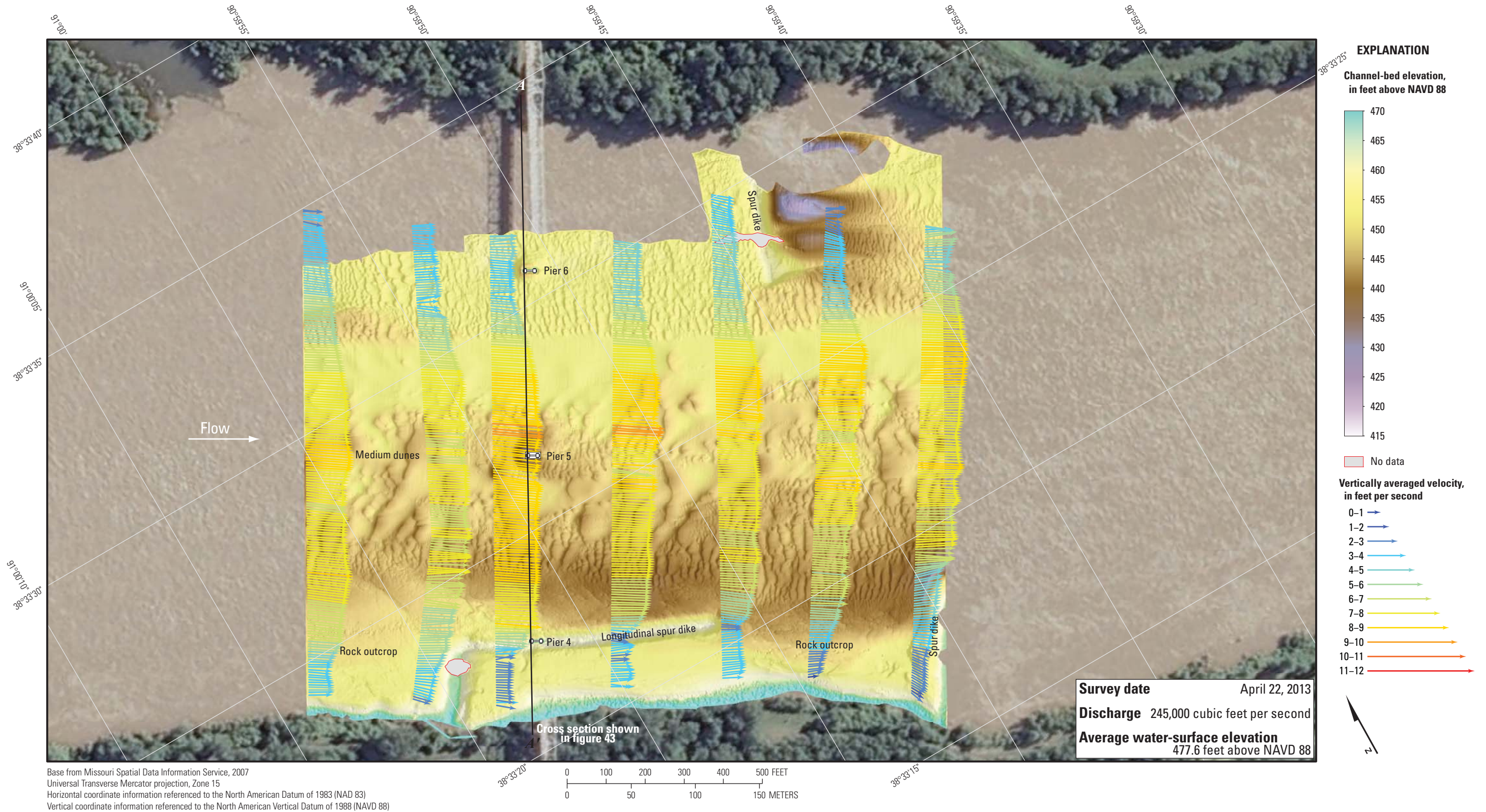
Figure 45. Bathymetry and vertically averaged velocities of the Missouri River channel in the vicinity of structure K0969 on State Highway 47 at Washington, Missouri.
