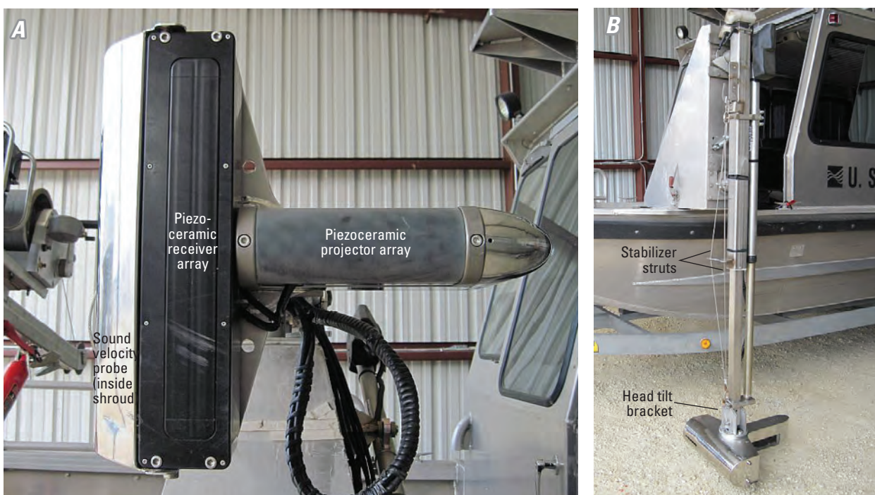
Figure 3. The Teledyne RESON SeaBat® 7125-SV2 multibeam echosounder, as viewed, A , from the bottom, and B , mounted on the port side of the U.S. Geological Survey boat.
