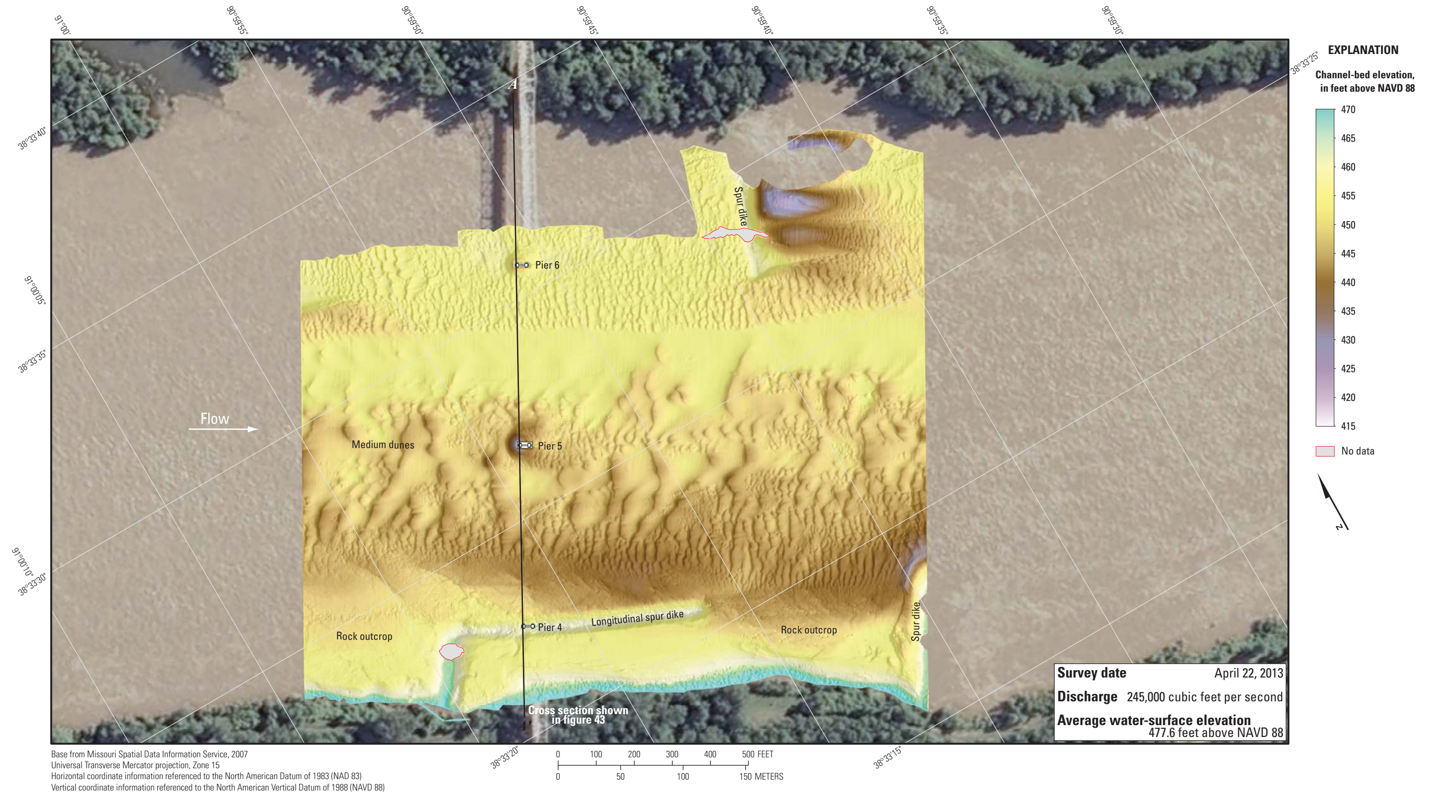
Figure 42. Bathymetric survey of the Missouri River channel in the vicinity of structure K0969 on State Highway 47 at Washington, Missouri.
