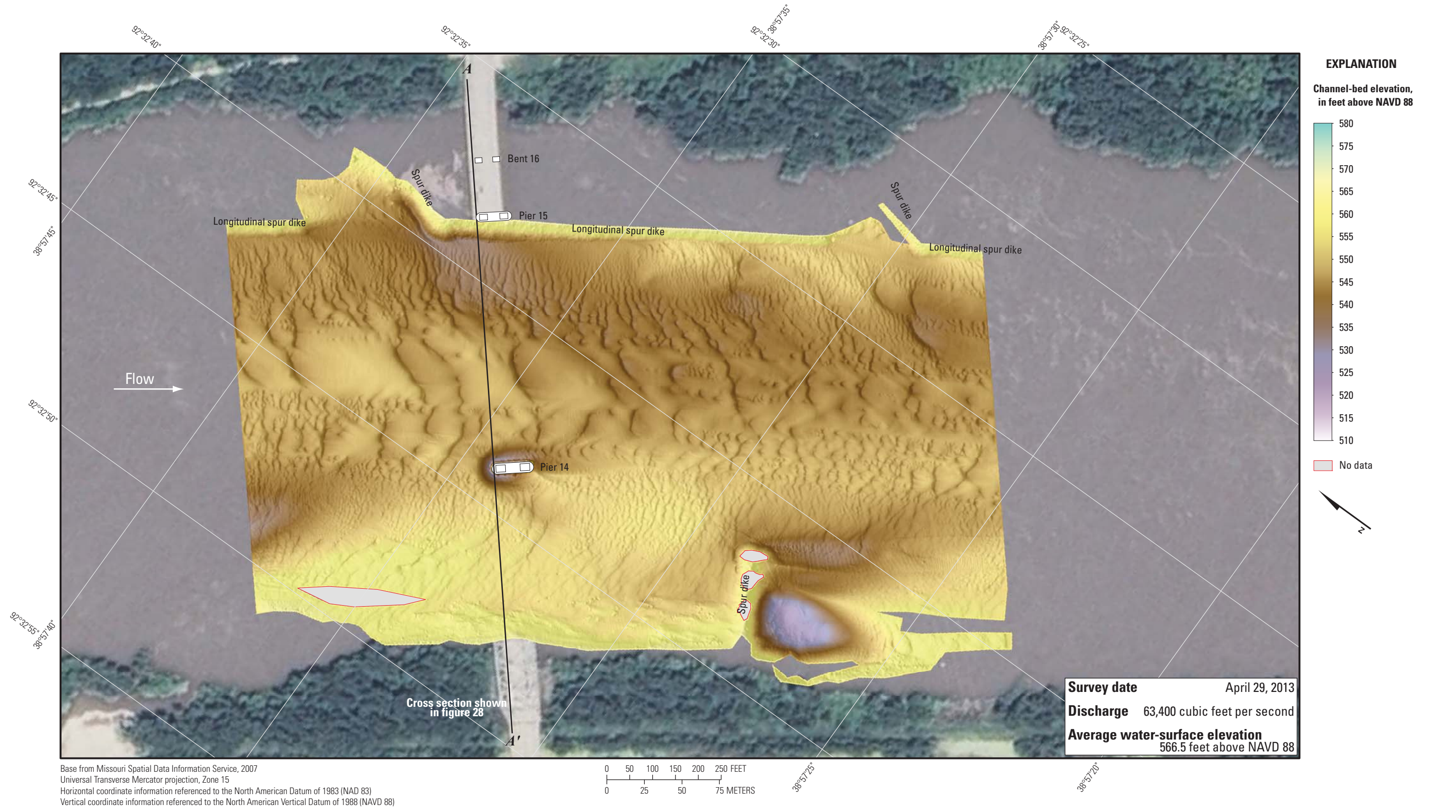
Figure 27. Bathymetric survey of the Missouri River channel in the vicinity of structure L0962 on Interstate 70 near Rocheport, Missouri.
