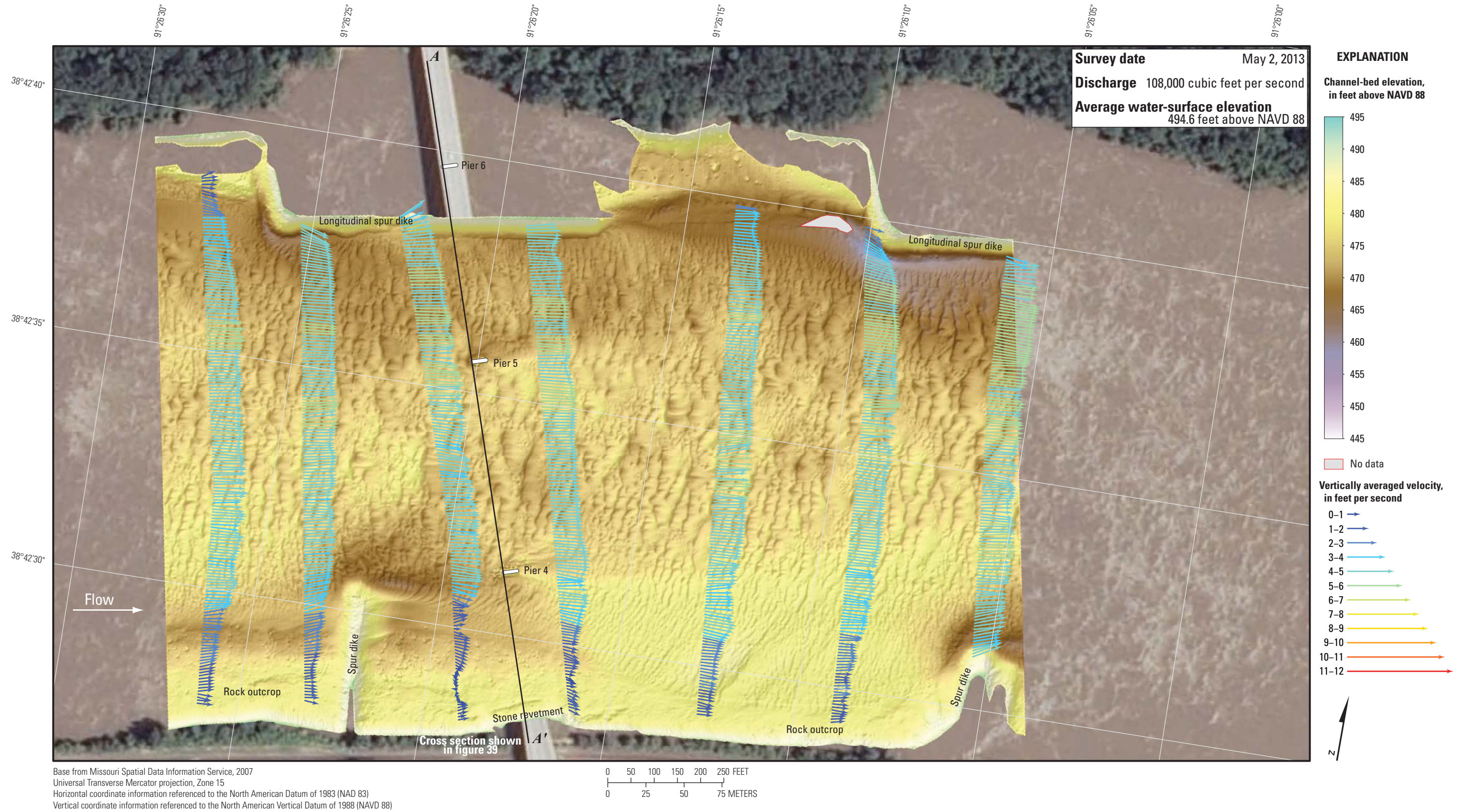
Figure 41. Bathymetry and vertically averaged velocities of the Missouri River channel in the vicinity of structure A6288 on State Highway 19 at Hermann, Missouri.
