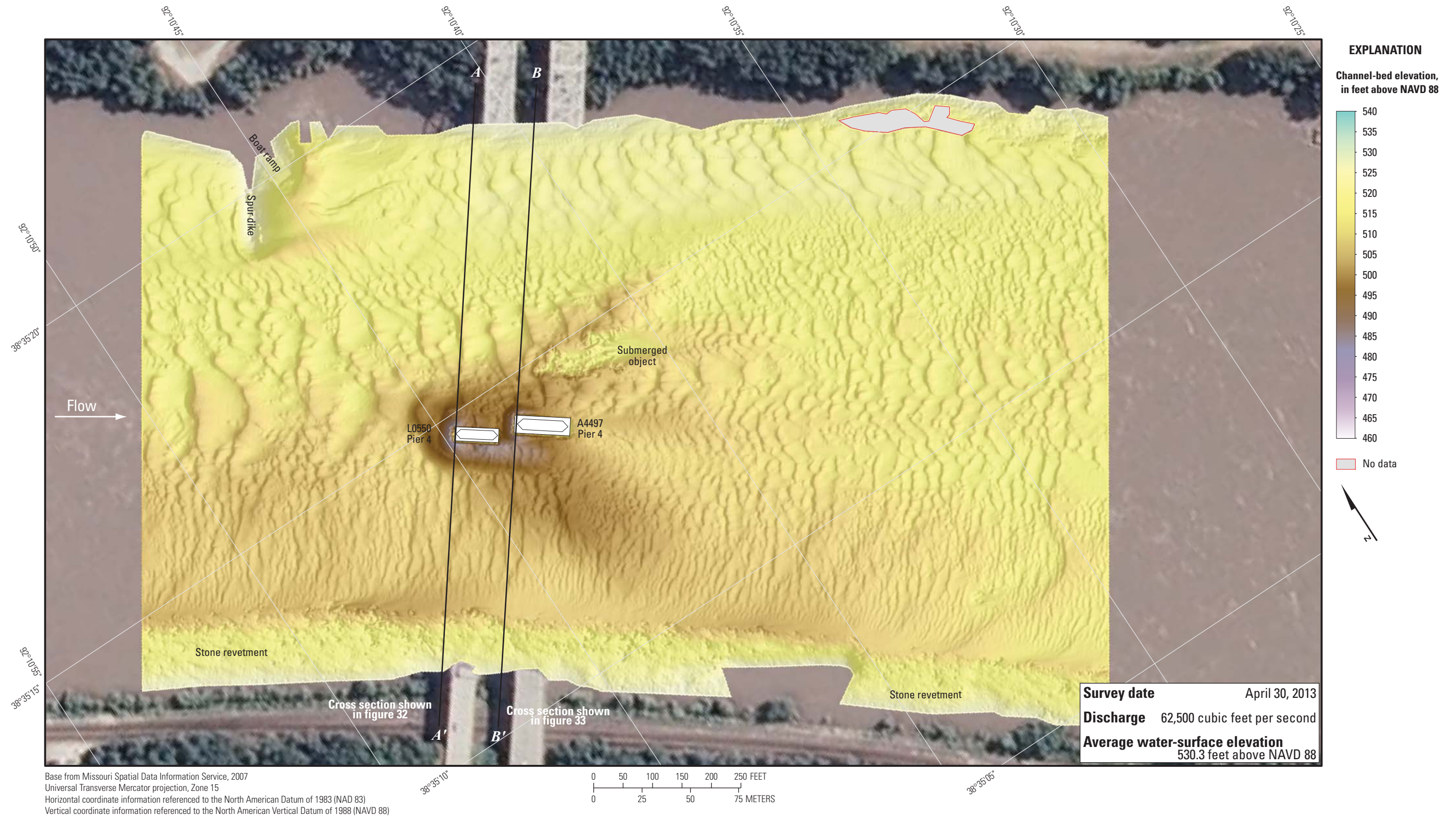
Figure 31. Bathymetric survey of the Missouri River channel in the vicinity of structures L0550 and A4497 on U.S. Highway 54 at Jefferson City, Missouri.
