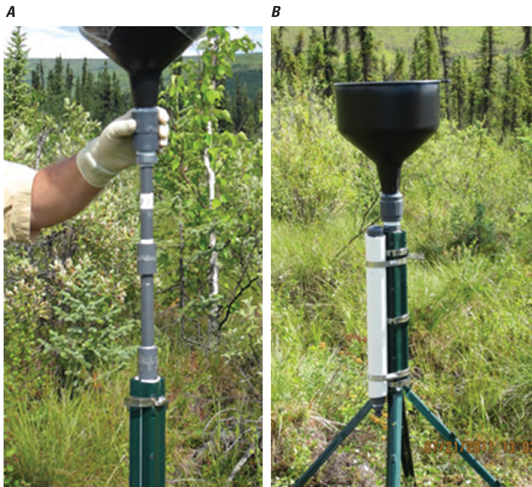
Fig. 1–2. An ion-exchange collector assembly. A , inserting the ion-exchange collector in the mounting stand. Note smoothed edges of both gray polyvinyl chloride couplings, which allow enough clearance for column to fit inside 1.25-inch diameter white polyvinyl chloride pipe pipe that is clamped inside of the mounting post legs. B , mounting stand containing a blank resin tube (capped and plugged) and the sample ion-exchange collector with a funnel attached. Note in this instance that protective nylon netting has not yet been placed over the funnel.
