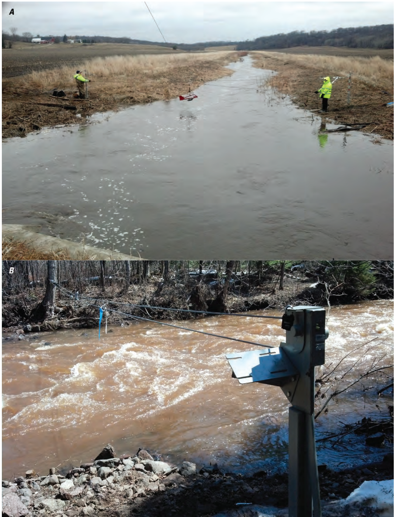
Figure 5. Configurations for collection of suspended-sediment concentrations at select sites. A , Cable-pulley deployment system at Cascade Creek at 45th Ave SW in Rochester, Minnesota (site 16), and B , Tacoma bank-operated-cableway at Sucker River near Palmers, Minnesota (site 2).
