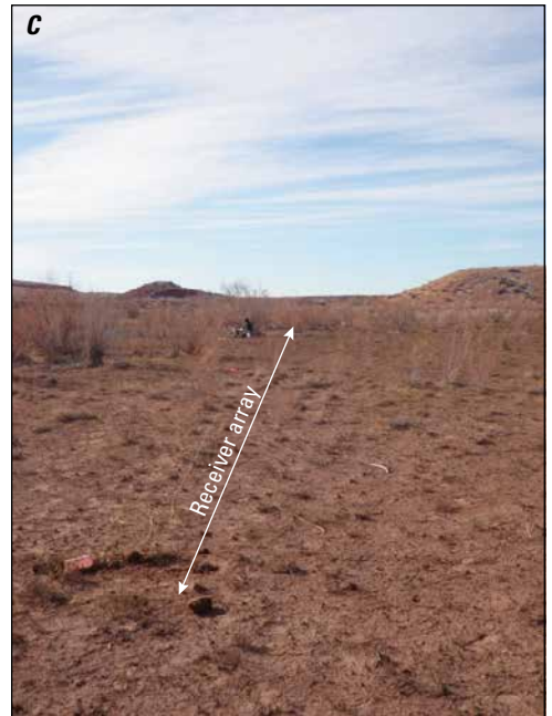
Figure 6. Diagram (A) and photographs (B, C) showing controlled source audio-frequency magnetotelluric setup used to study the Truxton Aquifer on the Hualapai Reservation, Mohave County, Arizona. Diagram (A) modified from Zonge, 1992; photographs by D.J. Bills (B) and Jon Mason (C) of the U.S. Geological Survey. m, meter; km, kilometer.
