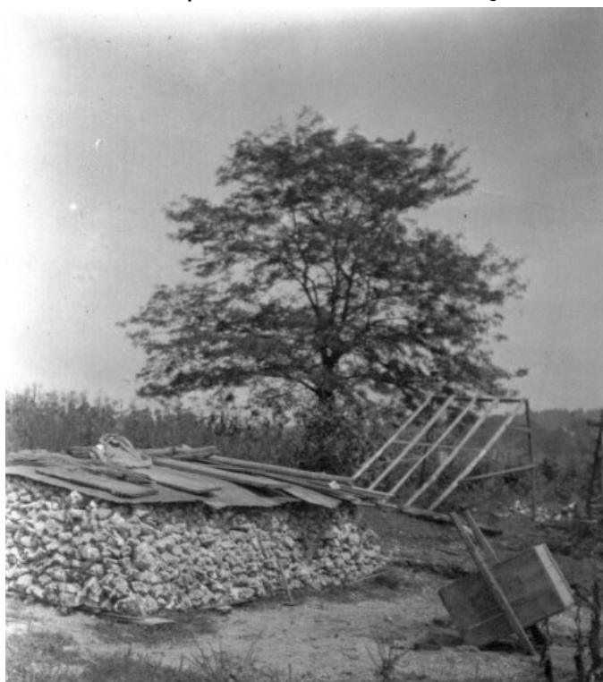
A. Cleaned barite stockpiled at mine site, rattle box in lower right
