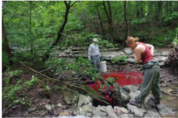
Figure 6. Swallet in Dry Creek in Ozark National Forest capturing all streamflow upgradient from CAFO spreading fields. In karst, surface water and groundwater interact as a single resource, with streams typically being pirated into the groundwater system as shown here, later resurging from downgradient springs back to the surface. Photo by Carol Bitting.
