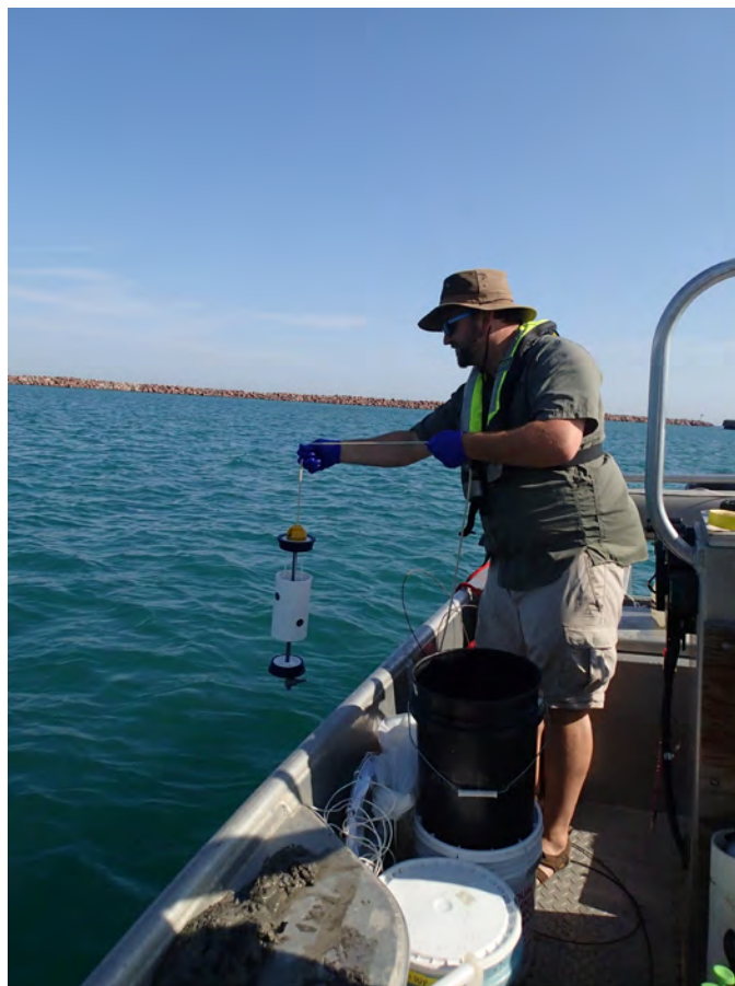
Figure 8. A Kemmerer™ vertical water sampler being deployed in Burns Harbor, Indiana, for sampling at 1-liter intervals, with subsequent compositing and subsampling for phytoplankton community, chlorophyll- a , and suspended solids.
