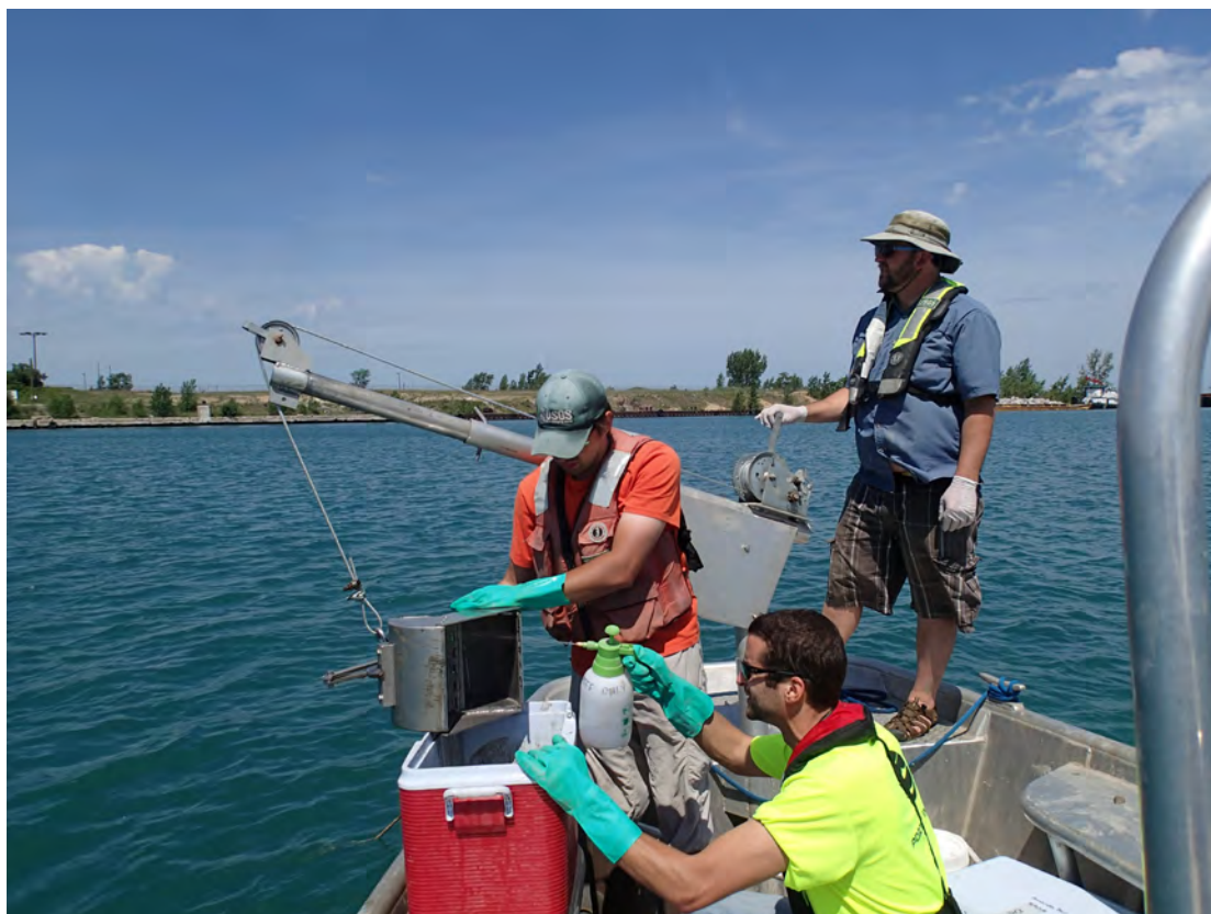
Figure 4. Ponar® dredge sampler containing bottom sediment being emptied and rinsed into a cooler for compositing into a single sample per location with subsequent subsampling for benthos community, particle-size fractionation, and volatile-on-ignition samples.
