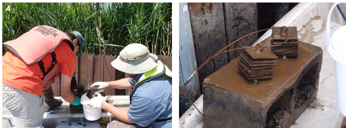
Figure 5. A , Hester-Dendy artificial substrate samplers being removed from a cement block and placed into a plastic bucket for later compositing and processing of attached benthic invertebrates. B , Close-up image of Hester-Dendy samplers after 6 weeks deployment.
