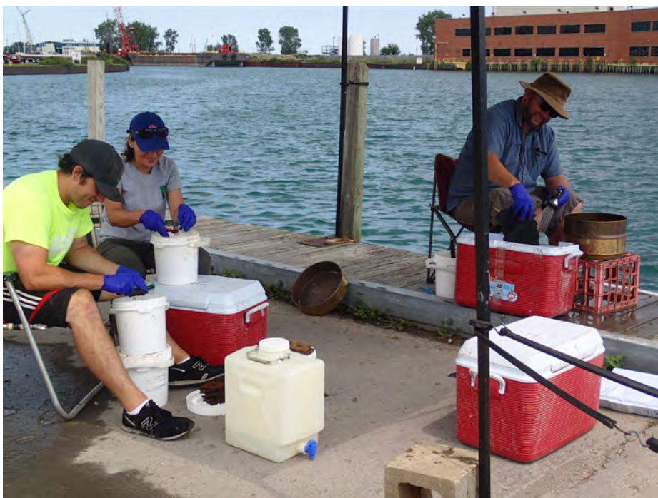
Figure 6. The processing of two types of benthos samples at Waukegan Harbor, Illinois: on the left, invertebrates being removed from plates of Hester-Dendy artificial substrate samplers prior to being sieved; on the right, invertebrates in composited sediment from Ponar® dredge samplers being removed from large rocks and debris during sieving.
