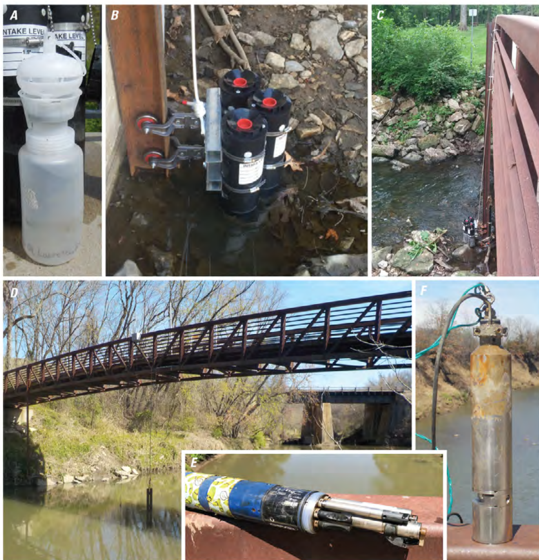
Figure 2. Sampling and monitoring stations used to evaluate a water-quality monitoring plan in Johnson County, Kansas: A , passive sampler, B , passive sampler carriage, C , passive sampler carriage installation at pylon of bridge, D , continuous water-quality monitor installation at Mill Creek (fig. 1, site 15), E , YSI Inc. EX02 multiparameter sonde, and F , Hach Co. Nitratax nitrate sensor.
