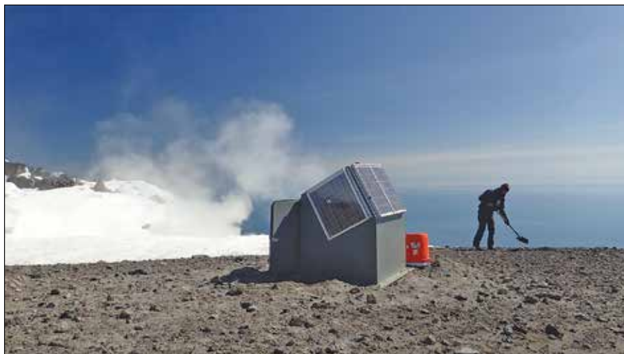
Figure 6. Joint MultiGAS/seismograph station AUSS installed on the summit of Augustine Volcano by AVO and CVO scientists on June 12 and 13, 2015. Photograph by Peter Kelly, USGS/CVO, June 13, 2015. AVO database image URL: https://www.avo.alaska.edu/images/image.php?id=79191 .
