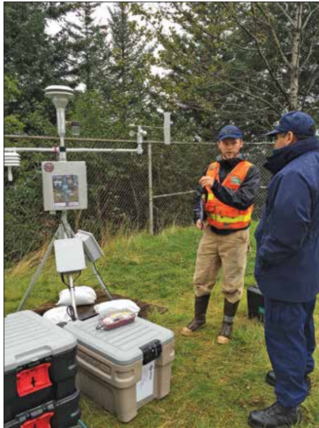
Figure 8. Alaska Volcano Observatory (AVO)-installed particulate monitors on Kodiak Island, to study resuspended 1912 volcanic ash and determine if the ash presents a health hazard to humans. In this image, AVO is training U.S. Coast Guard personnel on operation and maintenance of the monitor. Photograph by Kristi Wallace, USGS/AVO, September 8, 2015. AVO database image URL: https://www.avo.alaska.edu/images/image.php?id=80761 .
