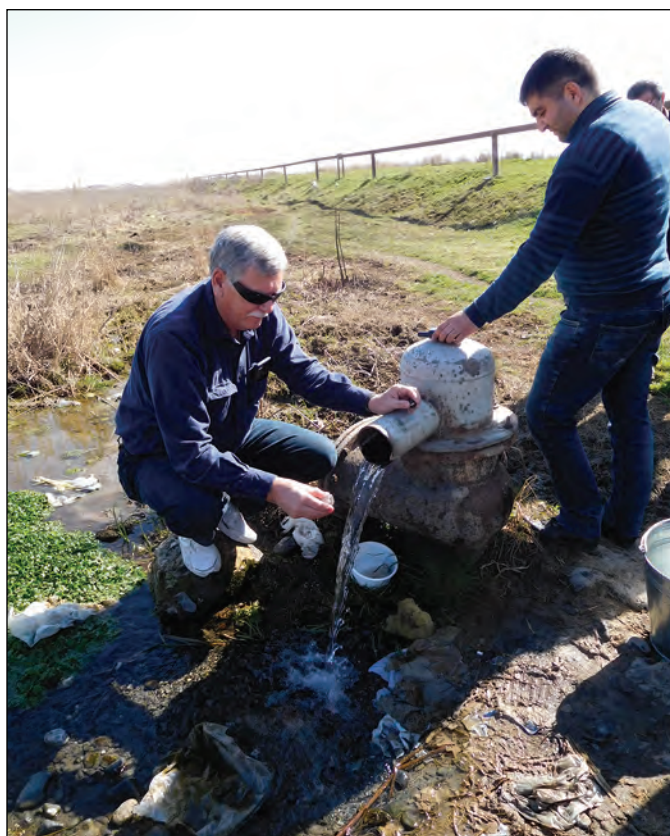
Figure 5. Collection of stable-isotope sample from a flowing well (U.S. Geological Survey site 400250044235601) in the Ararat Basin, Armenia.
